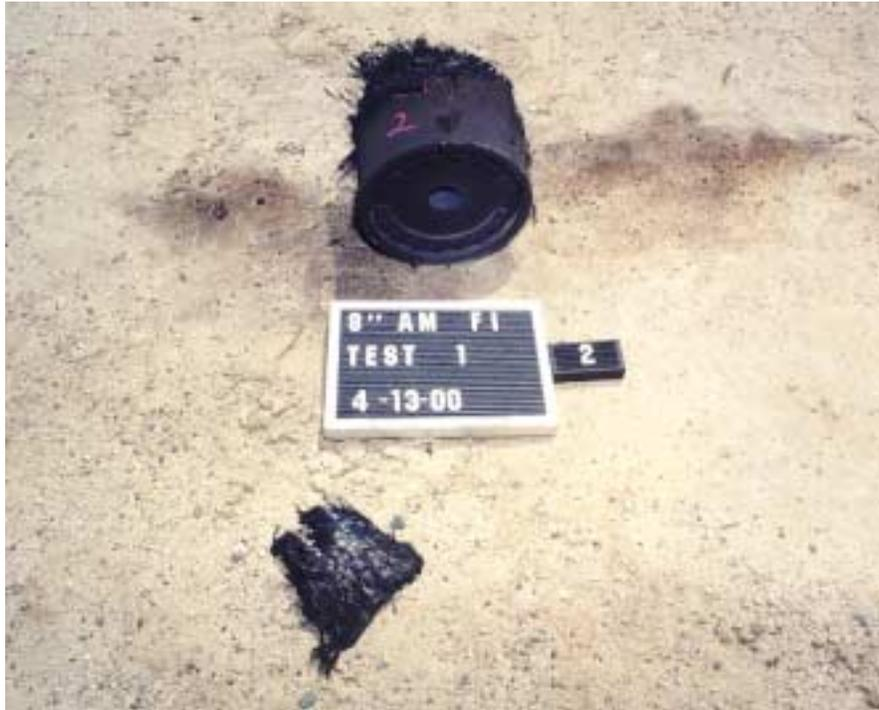
FIGURE 8. Material Recovered Following Fragment Impact Testing of IM Motor.
