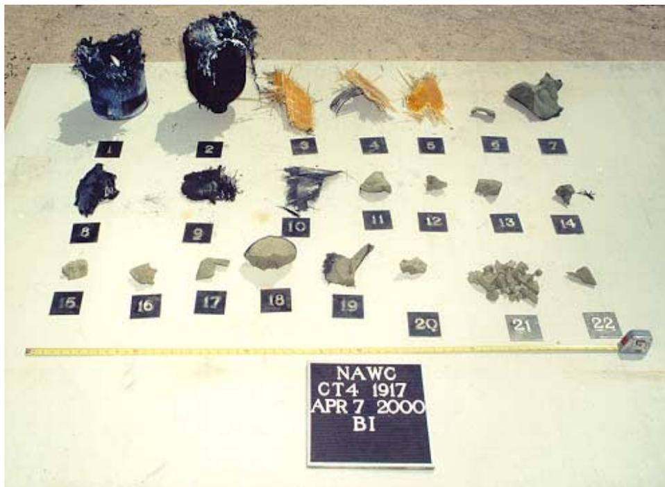
FIGURE 7. Material Recovered Following Bullet Impact Testing of IM Motor.
