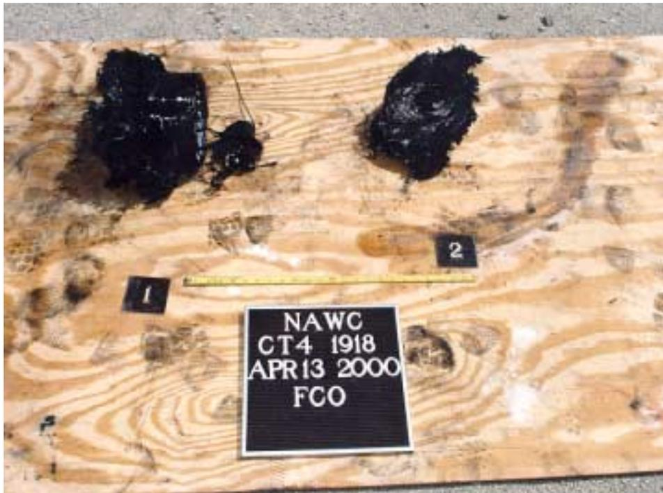
FIGURE 5. Material Recovered Following Fast Cookoff Testing of IM Motor.
