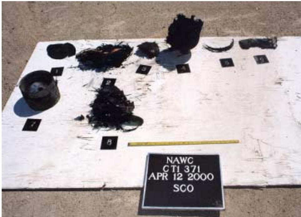
FIGURE 6. Material Recovered Following Slow Cookoff Testing of IM Motor.
