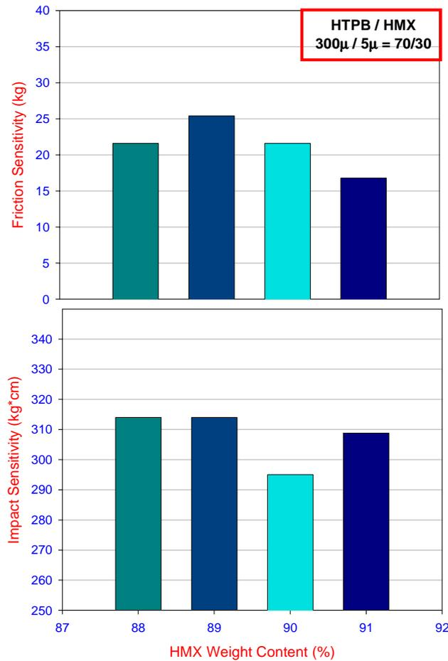
Generally speaking, the impact and friction sensitivity values of the developed formulations are quite good. It can be concluded that the influence of the solid loading (in the examined range of the HMX concentrations) on the small-scale safety characteristics is negligible.
