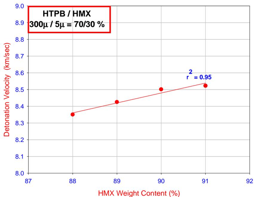
As it was expected, the detonation velocity increases with higher HMX loading. In the HMX content range studied this increase is quite close to linear. The value of detonation velocity approaches 8520 m/s at 91% HMX loading.
