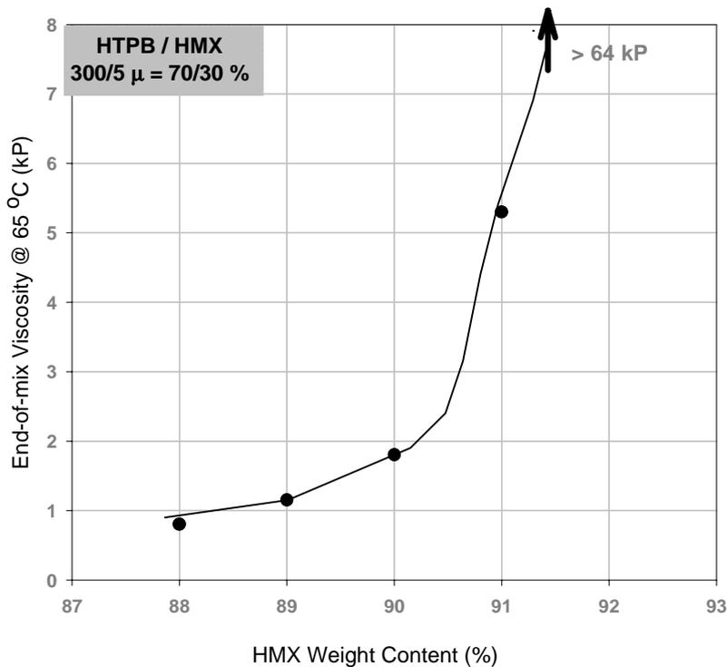
All formulations up to 90% of HMX are characterized by very good rheological properties (low end-of-mix viscosity values and no residual shear stress) due to the use of self-developed wetting agent. It seems that a weight loading of 91% HMX is a practical upper limit for these systems, taking into account processability
