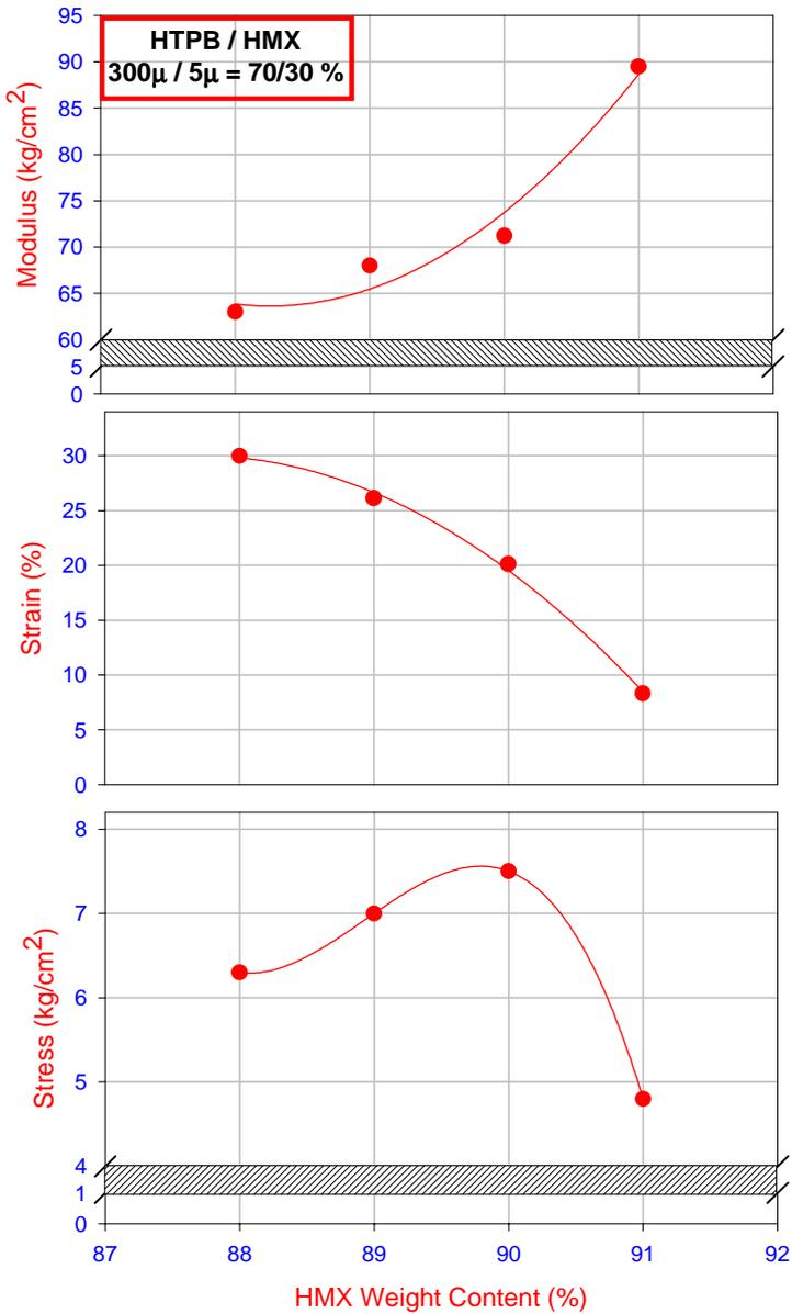
There is clear tendency of explosive's hardening with increase of solids loading. The increase of elasticity modulus and the decrease of real strain express this tendency. The mechanical properties are quite good up to 90% solids loading (engineering stress of 7.5 kg/cm<sup>2</sup>, real strain of 20%, origin modulus of 72 kg/cm<sup>2</sup>). Additional increase of HMX content up to 91% causes to deterioration of explosive's mechanical properties.
