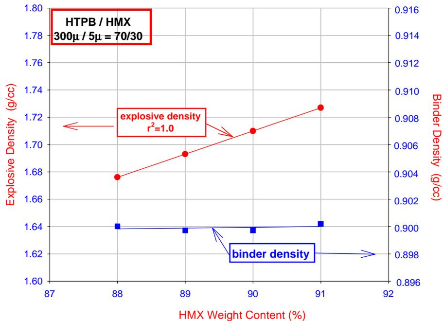
Actually, the measured explosive density values are equal to the TMD (Theoretic Maximal Density) values. It proves that even at the very high HMX content (relatively to conventional cure-cast PBX) the explosive is void free.
