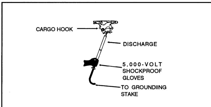
**Figure 5-14. Grounding technique.**
