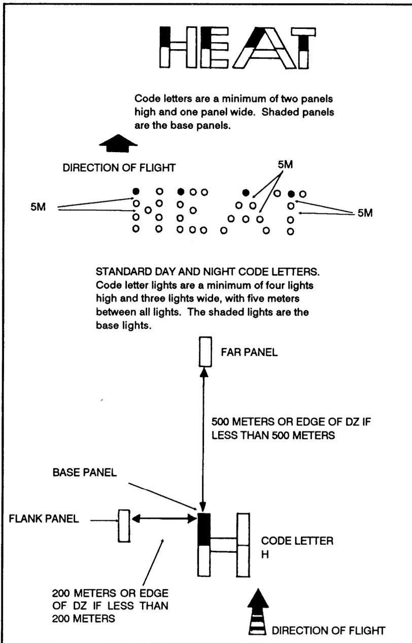
Figure 6-6. Horizontal clearance.
