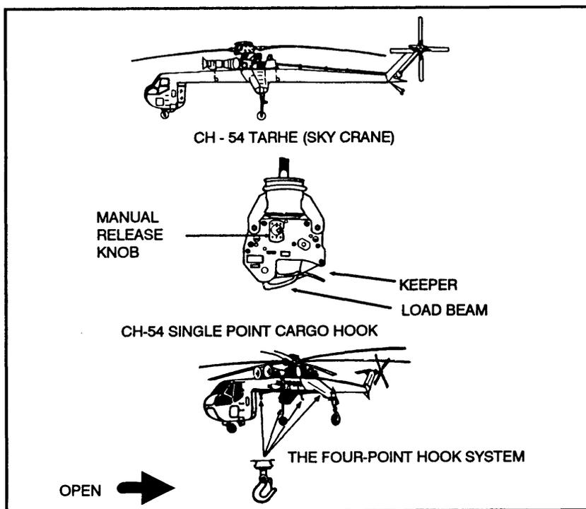
Figure 5-10. CH-54 Skycrane and its cargo hooks.
