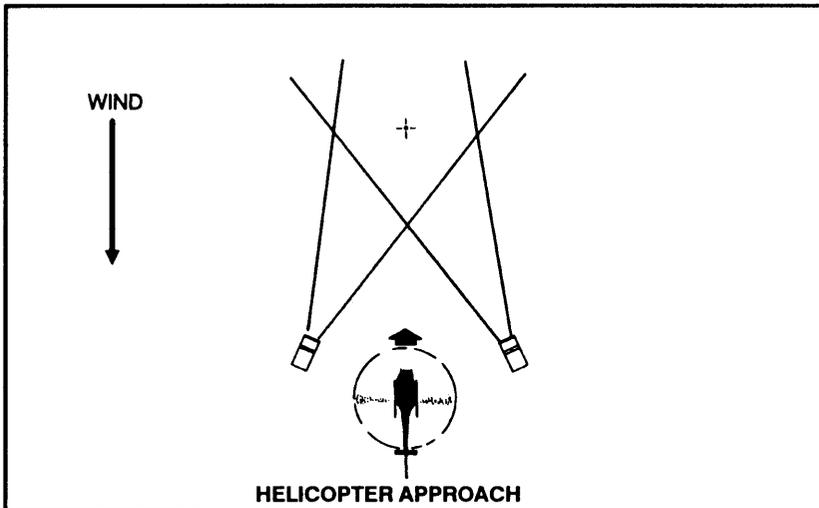
**Figure 4-14. Emergency night lighting by vehicle headlights.**
