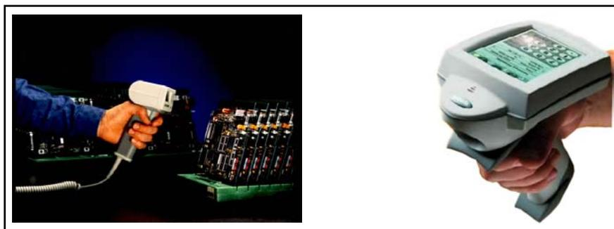
**Figure C-12. Bar Coded Data Collection Devices.**
