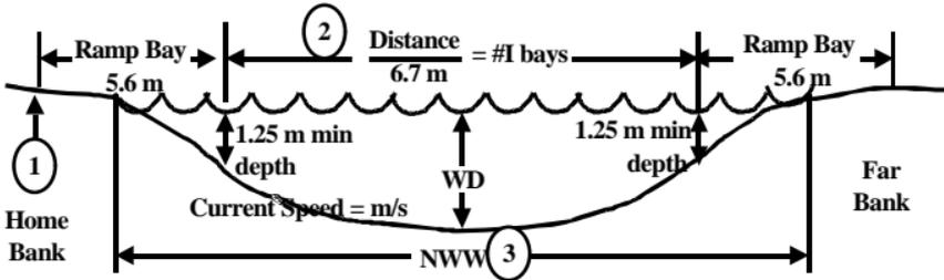
1. Start measurement at most suitable point where end of ramp bay is to be anchored (less ramp plates) and adjust measurement to meet 1.25 m min depth at 5.6 m.
