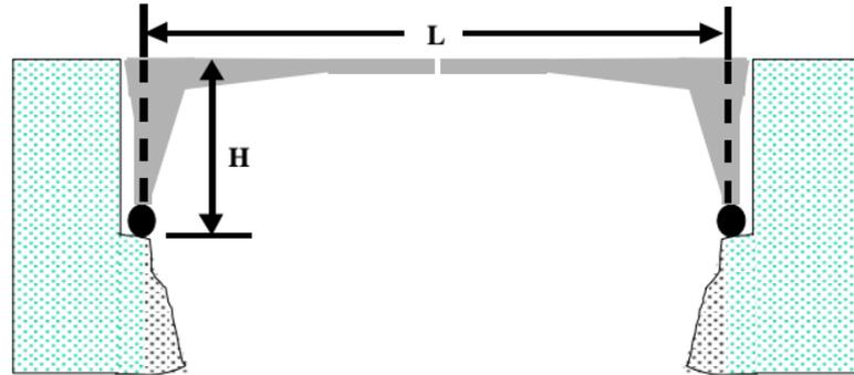
$H$  is the rise and  $L$  the span between bearings. For arch and pinned footing portal bridges calculate  $L_c$  by determining  $H/L$  and then  $L_c/L$ , and hence  $L_c$  from the supporting table. Interpolate as necessary.
