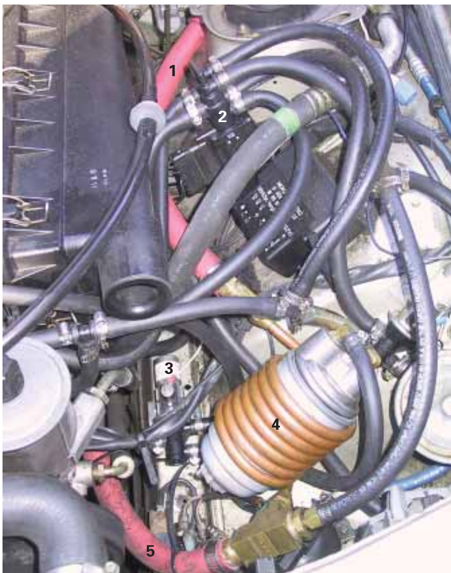
Under the 300CD's hood: 1) heater hose from heater-core splice; 2) six-port solenoid fuel switch; 3) three-port solenoid fuel switch; 4) vegetable oil heated filter; 5) HIH back to/from vegetable oil tank.
