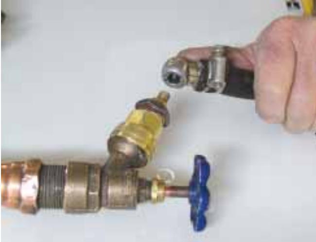
A pressure test fitting made from a Schrader valve and a female hose fitting.
