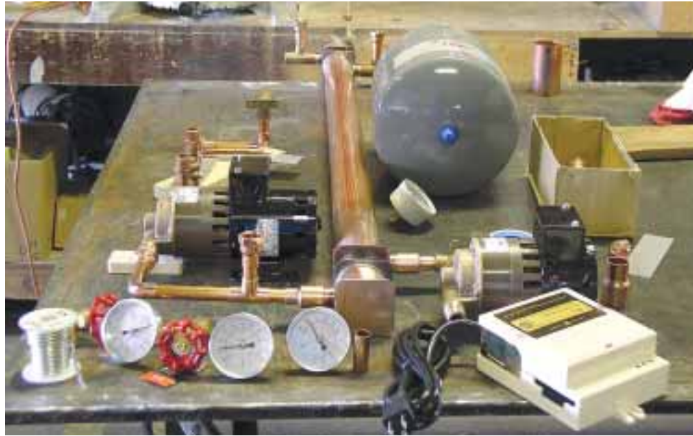
Laying out the components and plumbing parts in advance prevents headaches after the soldering begins.
