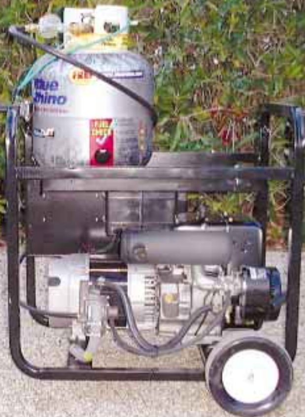
Herb Levitin's generator converted to propane, with the new tank in position.
