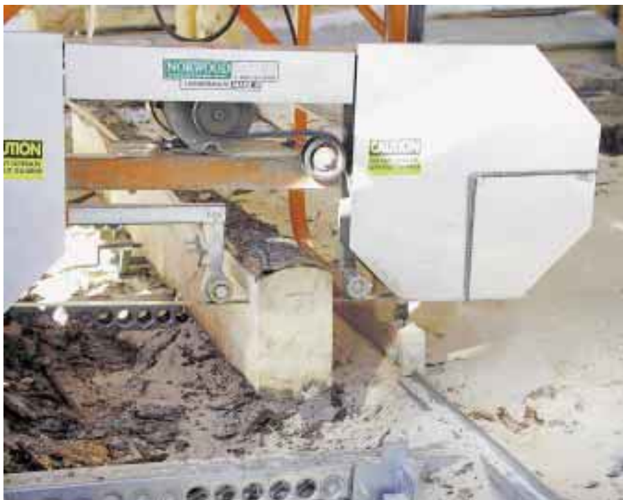
The solar-electric sawmill turns a log into lumber.
