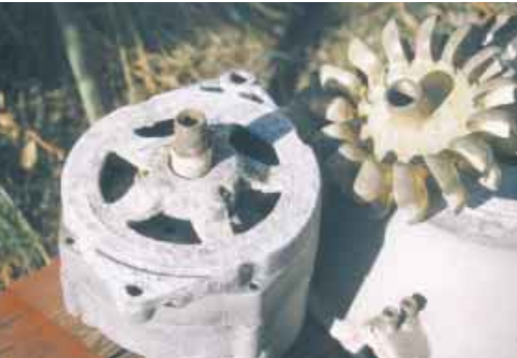
The Harris system was corroded beyond repair.
