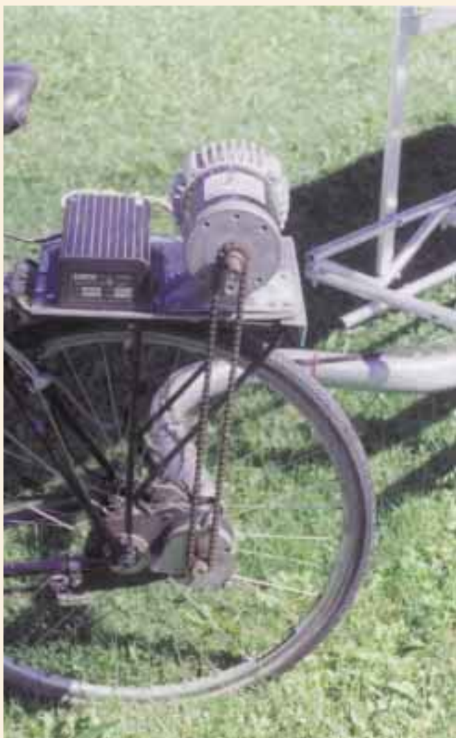
The bike's Curtis controller and Scott motor.
