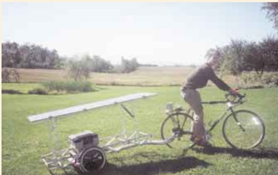
Four Solarex MSX-30 Lite PVs keep the batteries (in the plastic box) charged.
