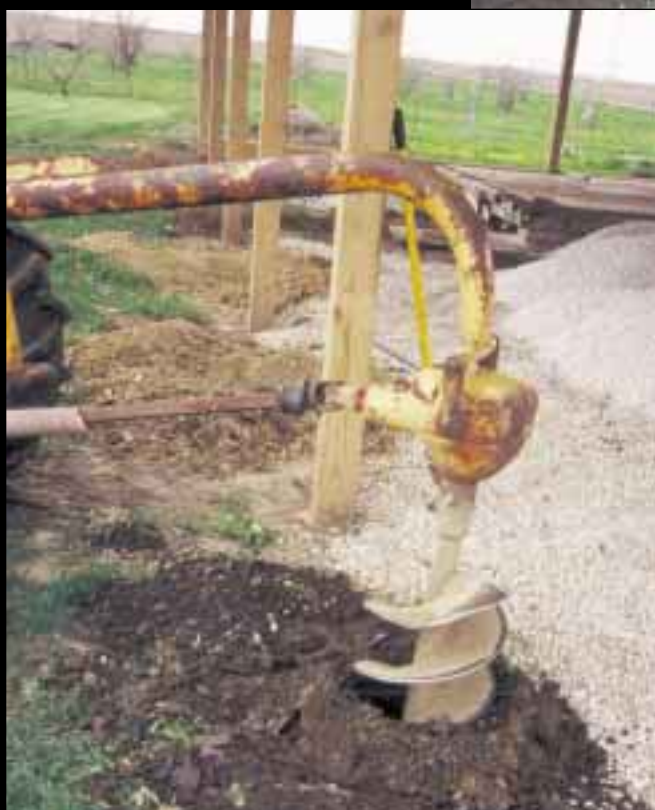
Post auger digging post holes.
