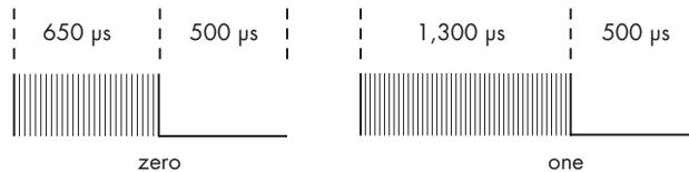
Figure 12-3: Modulated pulses in the Sony TV protocol
