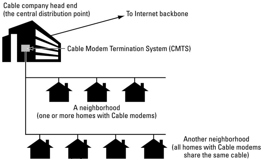
**Figure 1-4:** Cable modems provide high-speed Internet access over the cable TV network.
