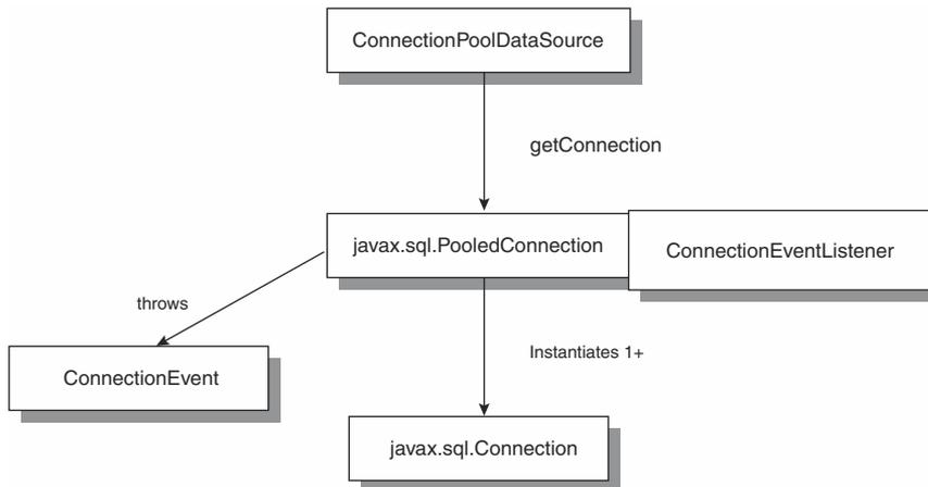
**Figure 2.6** PooledConnection/Connection classes.
