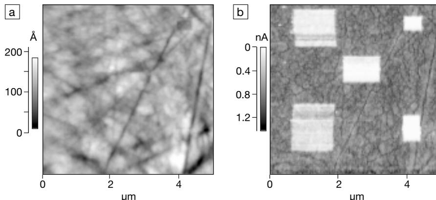
Figure 1. Atomic force microscope (AFM) images of (a) surface topography and (b) conductance of a  $\text{LiMn}_2\text{O}_4$  surface ( $5\ \mu\text{m} \times 5\ \mu\text{m}$ ) at ambient conditions recorded with the oxide poised at  $-1.0\ \text{V}$  versus the AFM tip, after surface modification of five areas produced at the opposite oxide-tip polarity.
