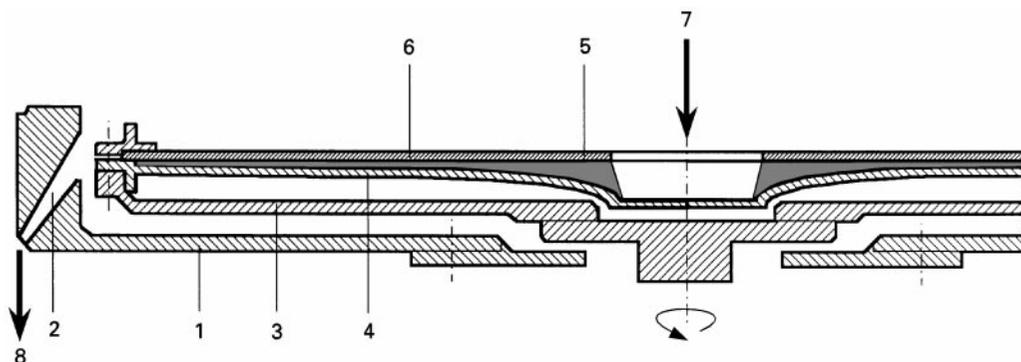
**Figure 12** Schematic diagram of preparative C-RPC. 1 = lower part of the stationary chamber, 2 = collector, 3 = motor shaft with the rotating disc, 4 = rotating planar column, 5 = stationary phase, 6 = quartz glass cover plate, 7 = mobile phase inlet, 8 = eluent outlet.
