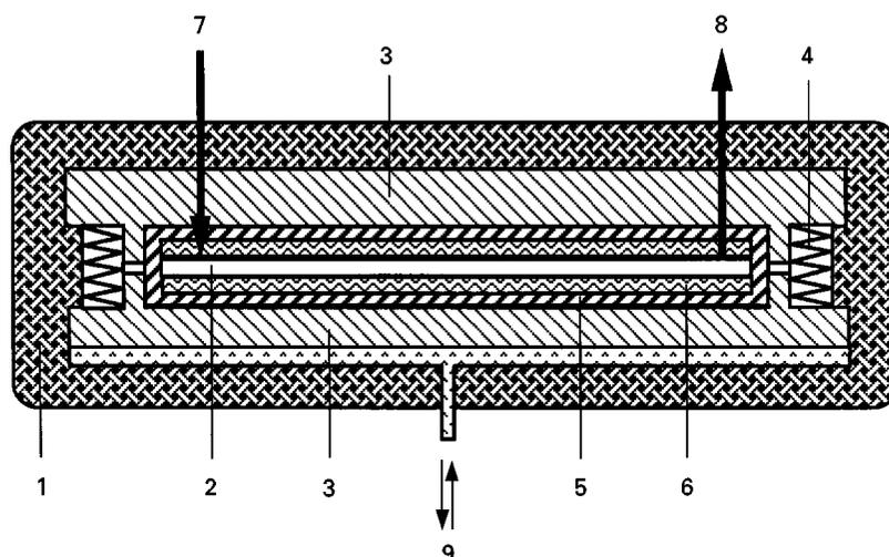
**Figure 2** Schematic diagram of online OPLC. 1, Support block; 2, chromatoplate; 3, support plate; 4, spring; 5, cassette system for fixing the chromatoplate between two Teflon layers; 6, Teflon layer; 7, Mobile phase inlet; 8, mobile phase outlet; 9, hydraulic system.
