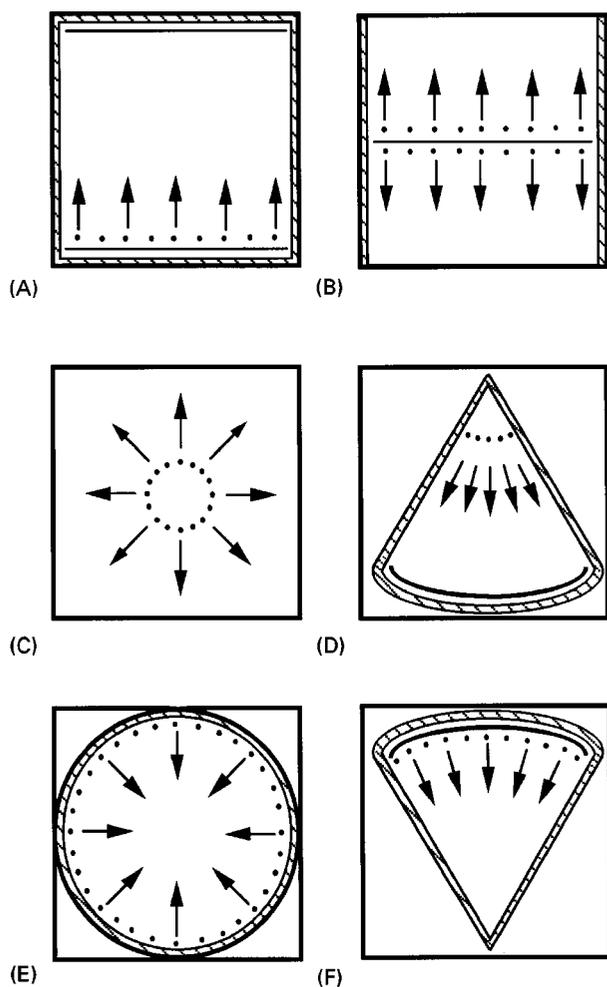
**Figure 5** Development modes in analytical OPLC using 20 cm  $\times$  20 cm HPTLC chromatographic plates. (A) Linear unidirectional; (B) linear two-directional; (C) circular with 8 cm development distance; (D) circular with 18 cm development distance, or online circular; (E) anticircular; (F) anticircular with 18 cm development distance, or online anticircular.
