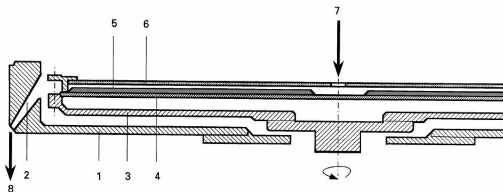
**Figure 11** Schematic diagram of preparative M-RPC. 1 = lower part of the stationary chamber, 2 = collector, 3 = motor shaft with the rotating disc, 4 = glass rotor, 5 = stationary phase, 6 = quartz glass cover plate, 7 = mobile phase inlet, 8 = eluent outlet.
