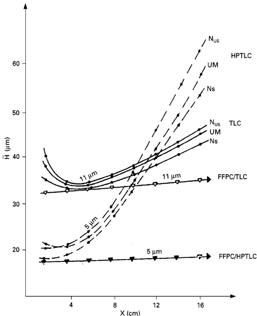
**Figure 1** Comparison of the efficiency of analytical TLC and HPTLC chromatographic plates when used with capillary action and forced-flow planar chromatography (FFPC).  $N_{US}$ , normal unsaturated chamber; UM, ultramicrochamber;  $N_S$ , normal saturated chamber.
