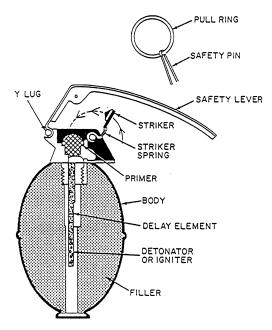
Figure 12-8.—Functioning of the fuze.
