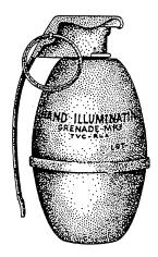
Figure 12-2.—Illuminating hand grenade, MK1.
