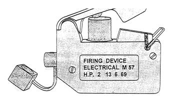
Figure 12-16.—The M57 firing device.
