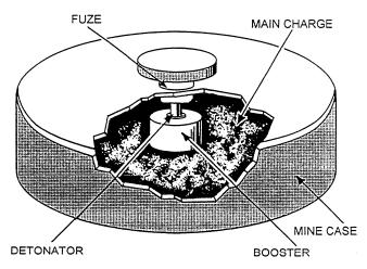
Figure 12-12.—Typical pressure type of land mine mechanism.
