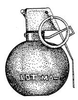
Figure 12-1.—Fragmentation hand grenade, M67.
