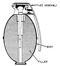
Figure 12-7.—Three main parts of the grenade.
