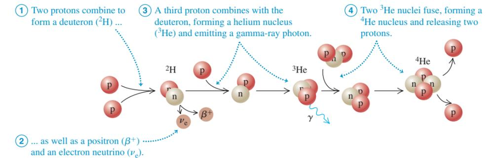
nucleon increases with  $A$  up to about  $A = 60$ , so fusion of nearly any two light nuclei to make a nucleus with  $A$  less than 60 is likely to be an exoergic reaction. In comparison to fission, we are moving toward the peak of this curve from the opposite side. Another way to express the energy relationships is that the total mass of the products is less than that of the initial particles.
