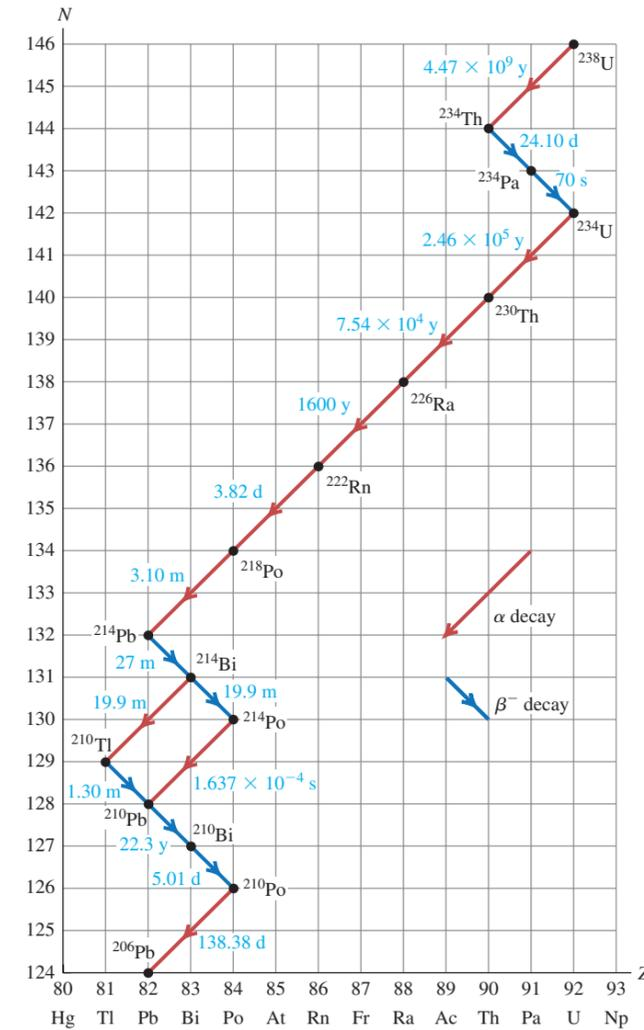
**43.8** Segrè chart showing the uranium  $^{238}\text{U}$  decay series, terminating with the stable nuclide  $^{206}\text{Pb}$ . The times are half-lives (discussed in the next section), given in years (y), days (d), hours (h), minutes (m), or seconds (s).
