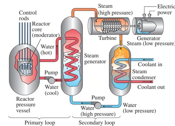
**43.16** Schematic diagram of a nuclear power plant.
