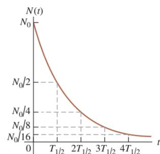
Figure 43.9 is a graph of this function, showing the number of remaining nuclei  $N(t)$  as a function of time.
