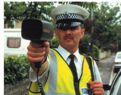
**37.18** This handheld radar gun emits a radio beam of frequency  $f_0$ , which in the frame of reference of an approaching car has a higher frequency  $f$  given by Eq. (37.25). The reflected beam also has frequency  $f$  in the car's frame, but has an even higher frequency  $f'$  in the police officer's frame. The radar gun calculates the car's speed by comparing the frequencies of the emitted beam and the doubly Doppler-shifted reflected beam. (Compare Example 16.19 in Section 16.8.)
