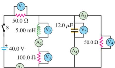
**30.64.** In the circuit shown in Fig. 30.24 the battery and the inductor have no appreciable internal resistance and there is no current in the circuit. After the switch is closed, find the readings of the ammeter (A) and voltmeters ( $V_1$  and  $V_2$ ) (a) the instant after the switch is closed and (b) after the switch has been closed for a very long time. (c) Which answers in parts (a) and (b) would change if the inductance were 24.0 mH instead?
