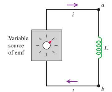
**30.6** (a) The potential difference across a resistor depends on the current. (b), (c), (d) The potential difference across an inductor depends on the rate of change of the current.
