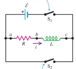
Closing switch  $S_2$  while opening switch  $S_1$  disconnects the combination from the source.
