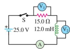
**30.65.** In the circuit shown in Fig. 30.25, switch S is closed at time  $t = 0$ . (a) Find the reading of each meter just after S is closed. (b) What does each meter read long after S is closed?
