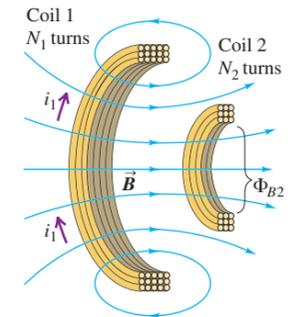
**30.2** This electric toothbrush makes use of mutual inductance. The base contains a coil that is supplied with alternating current from a wall socket. This varying current induces an emf in a coil within the toothbrush itself, which is used to recharge the toothbrush battery.
