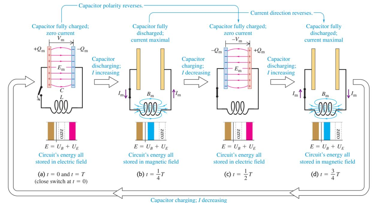
capacitor to a potential difference  $V_m$  and initial charge  $Q = CV_m$  on its left-hand plate and then close the switch. What happens?
