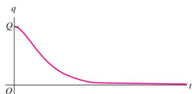
is completed. But because of  $i^2R$  losses in the resistor, the magnetic-field energy acquired by the inductor when the capacitor is completely discharged is *less* than the original electric-field energy of the capacitor. In the same way, the energy of the capacitor when the magnetic field has decreased to zero is still smaller, and so on.
