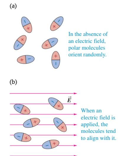
**24.19** Nonpolar molecules (a) without and (b) with an applied electric field  $\vec{E}$ .
