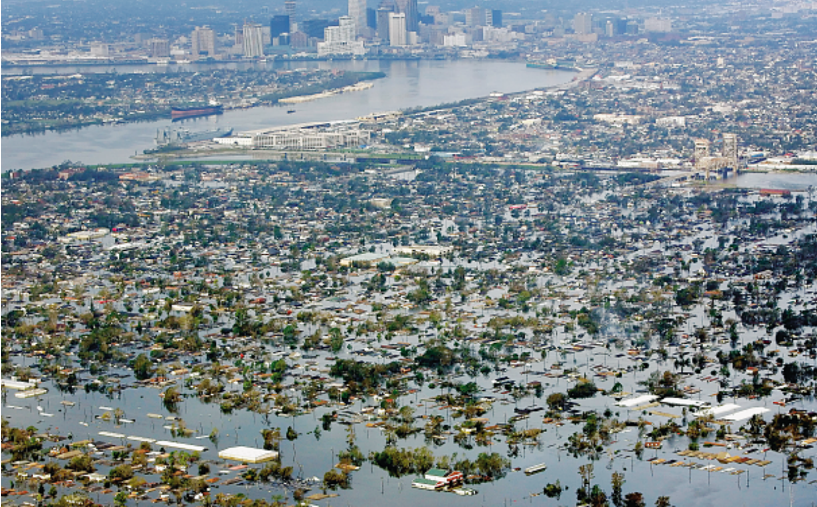
FIGURE 11-1 An estimated 80 percent of New Orleans was flooded after several levees failed in the wake of Hurricane Katrina. The storm surge caused the level of Lake Pontchartrain to rise, straining the levee system protecting the city. (AP Photo/David J. Phillip)
