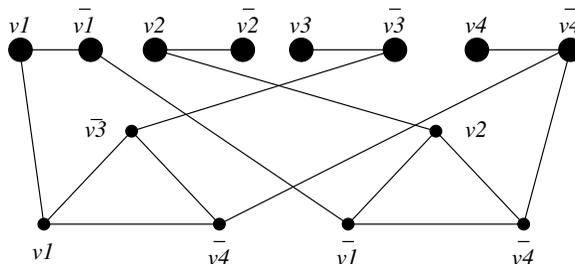
Figure 9.7: Reducing satisfiability instance  $\{\{v_1, \bar{v}_3, \bar{v}_4\}, \{\bar{v}_1, v_2, \bar{v}_4\}\}$  to vertex cover
