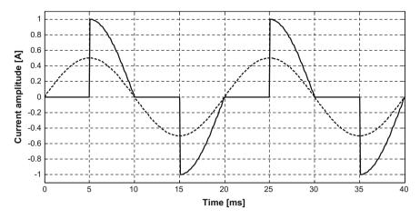
Fig. 4.32 Phase-Fired waveform test. Solid line—test waveform, dash line—reference waveform
