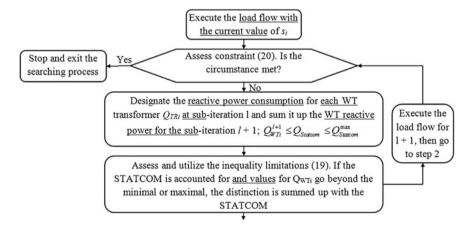
Fig. 7.4 Flowchart for the possible answer exploration process
