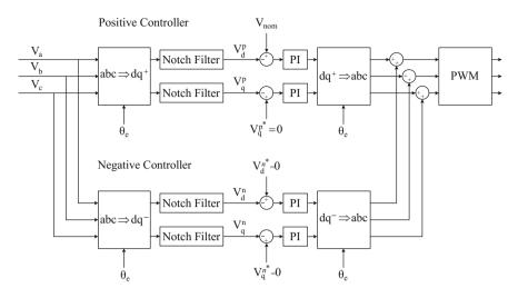
Fig. 3.14 Voltage control block diagram in dq reference frame
