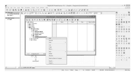
Fig. 11.20 DIgSILENT PowerFactory—introducing "General Set" to DPL command [1]
