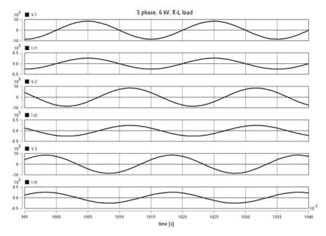
**Fig. 4.26** Time evolution of voltages and currents in circuit according Example 4.5, after compensation. From *top* to *bottom*: Voltage  $V_R$ , current  $i_R$ , voltage  $V_S$ , current  $i_S$ , voltage  $V_T$ , current  $i_T$
