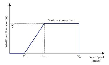
Fig. 12.4 The power curve of a wind turbine
