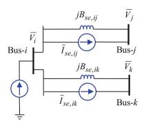
**Fig. 9.8** Voltage source model of GUPFC
