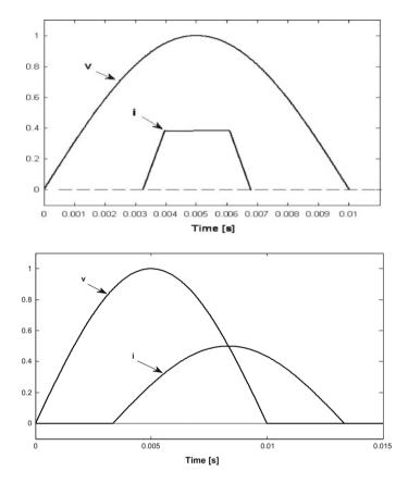
**Fig. 4.34** Example of non-ideal *PF*. Zero displacement between voltage and current fundamental component (top), but higher harmonic in current  $(\cos(\varphi_1) = 0, DF \neq 0)$ . Zero current harmonic content (bottom), but nonzero phase shift  $(\cos(\varphi_1) \neq 0, DF = 0)$
