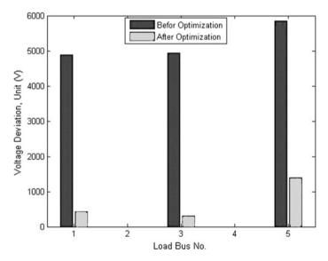
Fig. 10.20 Voltage deviation for 6-bus power system using genetic pattern search algorithm
