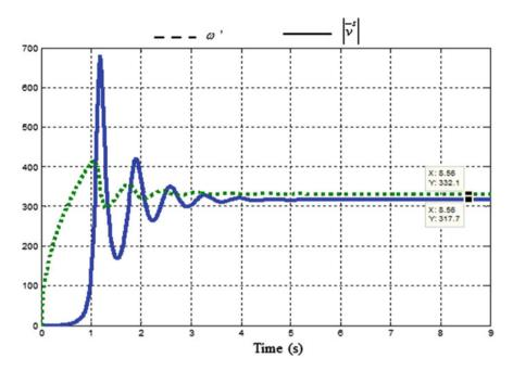
**Fig. 13.4** Variations of  $\omega'$  and  $|\bar{v}^s|$  at SEIG startup
