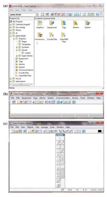
Fig. 15.19 a Screen of citect explorer. b Screen of project editor. c Screen of graphics builder d Screen of cicode editor. c Scheme of the CitectSCADA project
