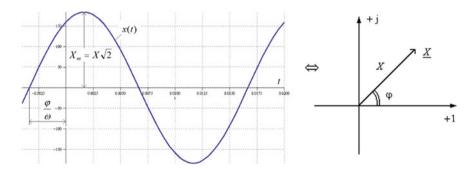
Fig. 2.3 Complex representation of sinusoidal and complex signals
