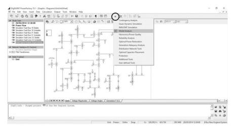
Fig. 11.40 DIgSILENT PowerFactory—Modal Analysis tool
