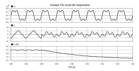
**Fig. 4.7** Time evolution of voltage (*top*), current from source (*middle*) and effective current from source for uncompensated (time <0.44) and compensated circuit (time > 0.44)
