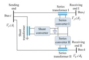
**Fig. 9.6** Voltage source model of GUPFC
