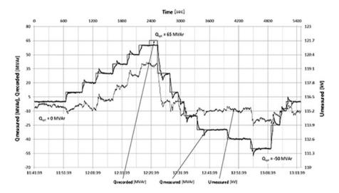
Fig. 6.13 Q-V diagram with imposed Q
