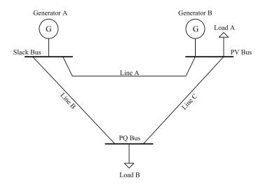
Fig. 10.1 Three-bus power system
