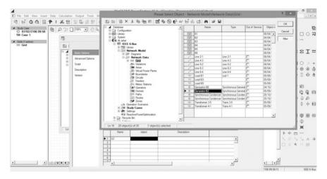
Fig. 11.23 DIgSILENT PowerFactory—defining external variables to the DPL [1]
