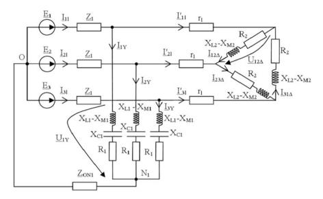
Fig. 1.7 Equivalent three-phase circuit
