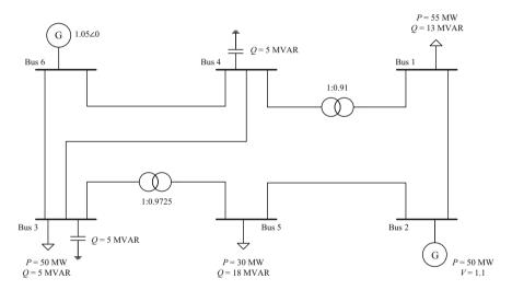
Fig. 10.29 Single-line diagram of IEEE 6-bus standard power system
