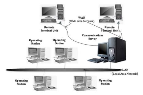
Fig. 15.7 Second generation of SCADA systems
