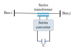
**Fig. 3.6** Unified Power Flow Controller (UPFC)
