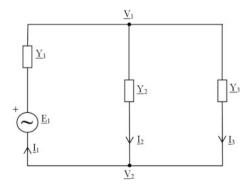
Fig. 2.30 Resistive-inductive AC circuit
