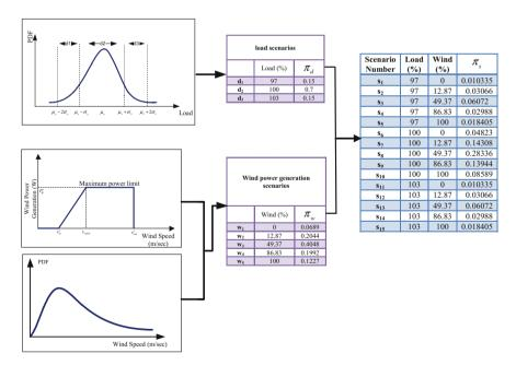
Fig. 12.5 Illustration of scenario generation procedure
