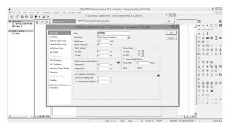
Fig. 11.13 DIgSILENT PowerFactory—adjusting tap settings of transformers [1]
