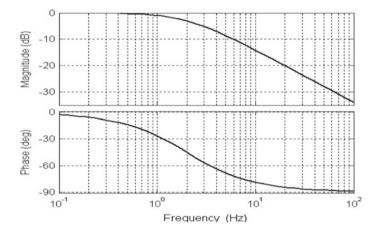
Fig. 4.29 Magnitude and phase response of low-pass filter 1st order with cutoff frequency 2 Hz
