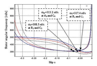
**Fig. 13.11** Tilting from  $R_0$  = 111 Ω and  $C_0$  = 87.5 μF to  $(R_2$  = 86 Ω,  $C_2$  = 95.5 μF) and  $(R_1$  = 132 Ω,  $C_1$  = 83 μF)
