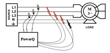
Fig. 1.26 Wiring diagram for U, I, f measurements
