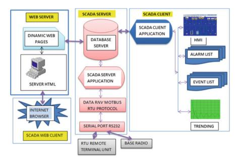
Fig. 15.9 SCADA software architecture
