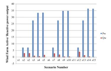
Fig. 12.12 Active/reactive power output of wind farm (located at bus 20) in all scenarios (in MW and MVAR) - (Case-I)
