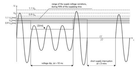
Fig. 1.24 Exemplification of a voltage dip and a short supply interruption, classified according to EN 50160;  $U_n$ —nominal voltage of the supply system (rms),  $U_A$ —amplitude of the supply voltage, U (rms)—the actual rms value of the supply voltage [3]
