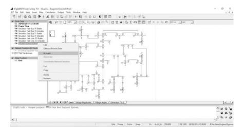
Fig. 11.39 DIgSILENT PowerFactory—activating Small Signal Analysis study case
