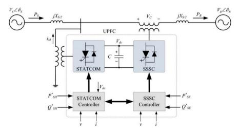
Fig. 8.28 The block diagram of UPFC
