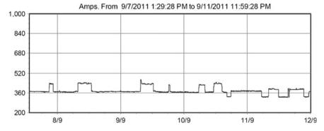
Fig. 2.27 The current variation on the consumer's most loaded phase taken on a monitor interval
