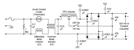
Fig. 4.35 Example of passive PFC [70, 71]
