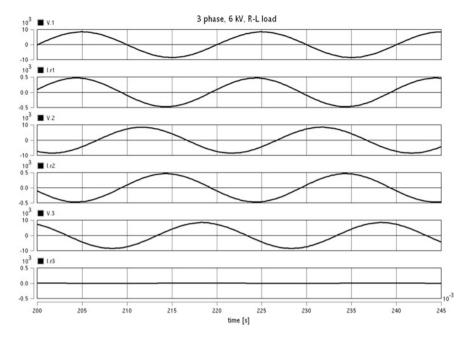
Fig. 4.25 Time evolution of voltages and currents in circuit according Example 4.5, before compensation. From *top* to *bottom*: Voltage  $V_R$ , current  $i_R$ , voltage  $V_S$ , current  $i_S$ , voltage  $V_T$ , current  $i_T$
