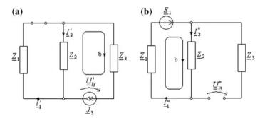
Fig. 2.12 Superposition principle
