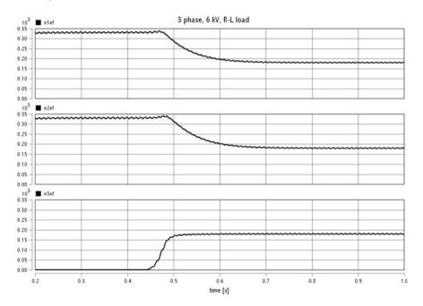
Fig. 4.27 Time evolution of RMS currents in circuit according Example 4.4, before and after compensation. Compensation parts are connected in time  $\geq 0.44$ . From *top* to *bottom*: RMS currents  $i_R$ ,  $i_S$ ,  $i_T$
