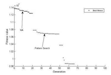
$\textbf{Fig. 10.24} \ \ \text{Reactive power optimization trend for 14-bus power system using genetic pattern search algorithm}$
