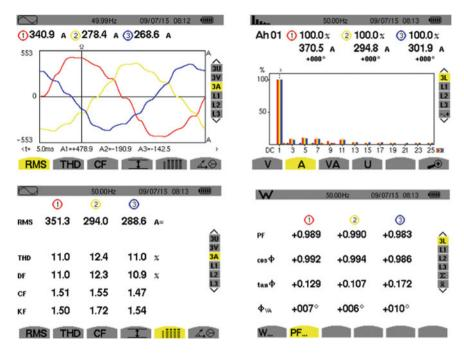
Fig. 1.29 Current signals, harmonics and various PQ parameters measured for a low-voltage industrial load
