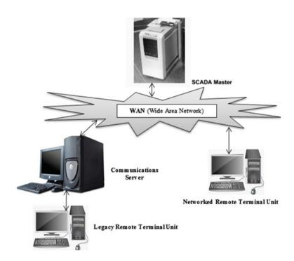
Fig. 15.8 Third Generation of SCADA systems
