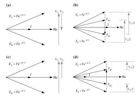
Fig. 8.10 Phasor diagram of ideal series reactive compensator;  $\mathbf{a}$  capacitive operation without compensation,  $\mathbf{b}$  capacitive operation with compensation,  $\mathbf{c}$  reactive operation without compensation,  $\mathbf{d}$  reactive operation with compensation
