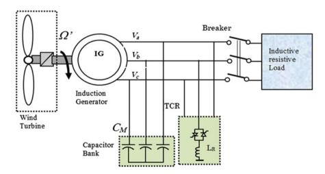
Fig. 13.1 Global diagram configuration of an isolated SEIG
