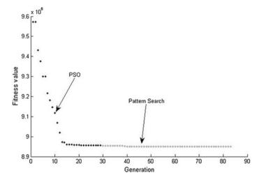
$\textbf{Fig. 10.15} \ \ \text{Reactive power optimization trend for 6-bus power system using particle swarm} \\ \text{pattern search algorithm}$
