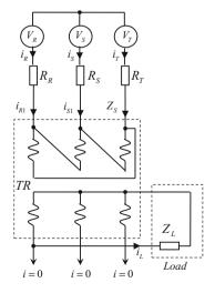
Fig. 4.18 Three-phase network with transformer TR ( $\Delta$  to Y connection) with unbalanced load and compensation circuit
