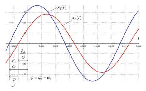
Fig. 2.2 The phase-shift between two sinusoidal signals
