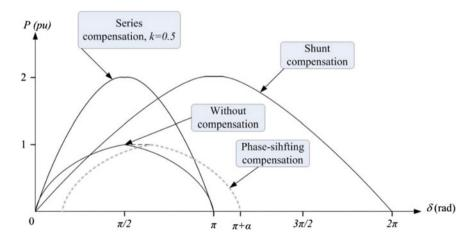
Fig. 8.11 Power transfer characteristics for several compensation cases
