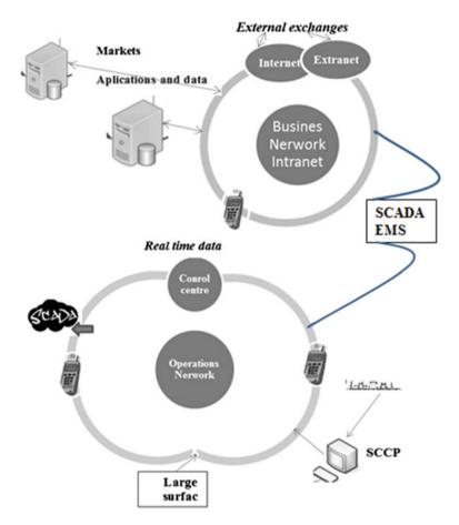
Fig. 15.11 SCADA energy management system
