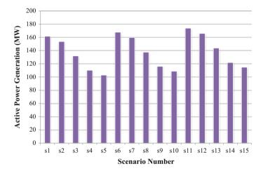
Fig. 12.17 Active power generation in slack bus (bus 1) in all scenarios (in MW)-(Case-II)
