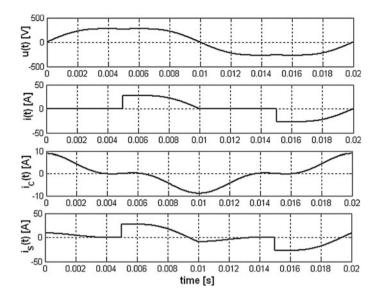
**Fig. 4.10** Voltage and currents in nonlinear circuit. From *top* to *bottom*: Power source voltage, current through the load, current through compensation capacitor and current from source after compensation (Example 4.3)
