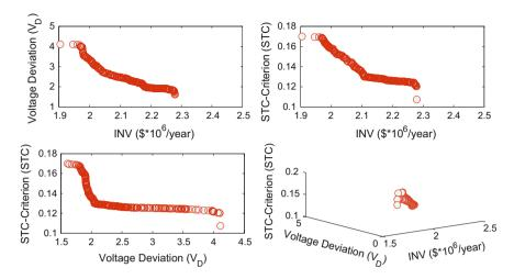
$\textbf{Fig. 9.19} \ \ \text{The Pareto archive in two-dimensional and three-dimensional objective area based on framework } 3$
