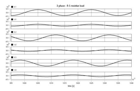
**Fig. 4.23** Time evolution of voltages and currents in circuit according Example 4.4, after compensation. From *top* to *bottom*: Voltage  $V_R$ , current  $i_R$ , voltage  $V_S$ , current  $i_S$ , voltage  $V_T$ , current  $i_T$
