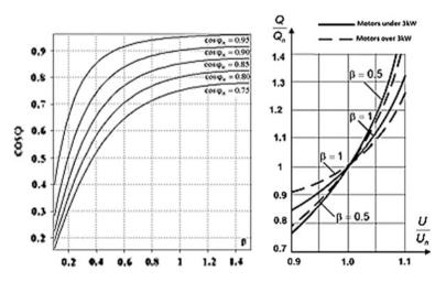
Fig. 2.17 Power factor variation function of asynchronous motor's loading and the reactive power consumption for small and big power motors function of the relative power voltage
