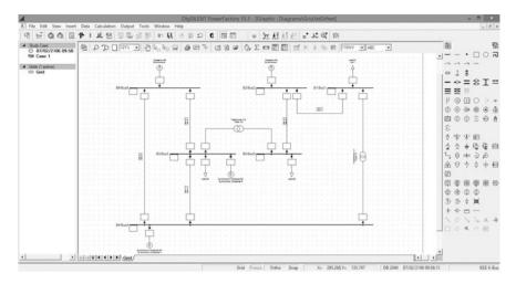
Fig. 11.5 DIgSILENT PowerFactory—IEEE 6-bus power grid [1]
