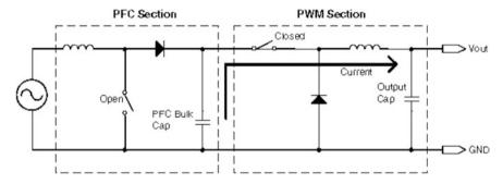
Fig. 4.42 Powering the Output [85]
