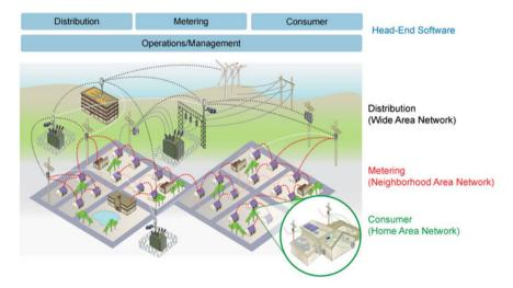
Fig. 14.4 Mesh Networking in Smart Grid Application [12]
