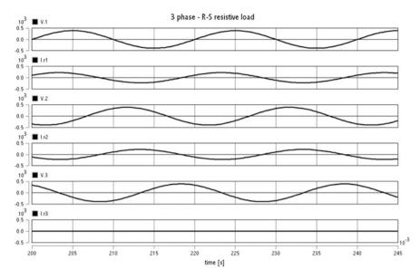
Fig. 4.22 Time evolution of voltages and currents in circuit according Example 4.4, before compensation. From *top* to *bottom*: Voltage  $V_R$ , current  $i_R$ , voltage  $V_S$ , current  $i_S$ , voltage  $V_T$ , current  $i_T$
