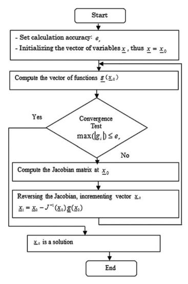
Fig. 13.9 Flowchart of the iterative method of Newton-Raphson
