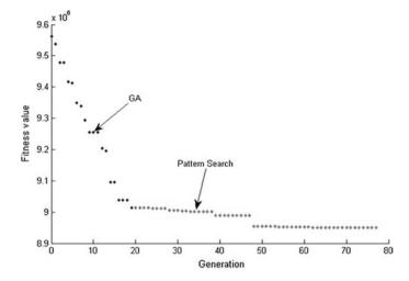
$\textbf{Fig. 10.18} \ \ \text{Reactive power optimization trend for 6-bus power system using genetic pattern search algorithm}$
