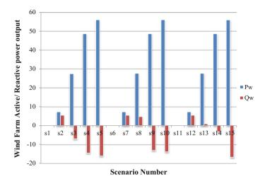
Fig. 12.18 Active and reactive power output of wind farm (located at bus 20) in all scenarios (in MW and MVAR)—(Case-II)
