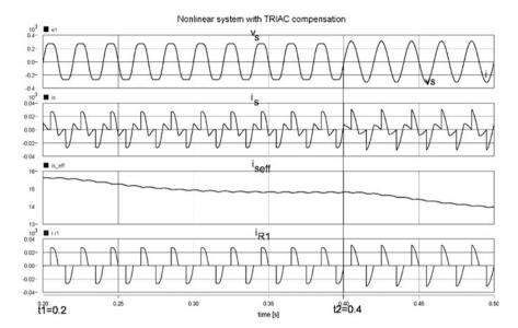
**Fig. 4.11** Time diagram of voltage and currents in nonlinear circuit during the automatic compensation. From *top* to *bottom*: Voltage of power source, supply current  $i_5$ , effective value of supply current, current through the load. Compensation start in time t = 0.2. Source voltage is changed in t = 0.4 to pure sinusoidal. The time slice is  $\langle 0.20 \div 0.50 \rangle$  (Example 4.3)
