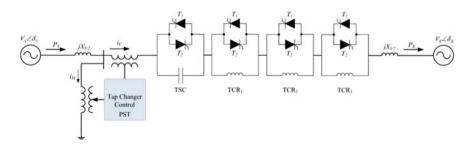
Fig. 8.29 The block diagram of DPFC
