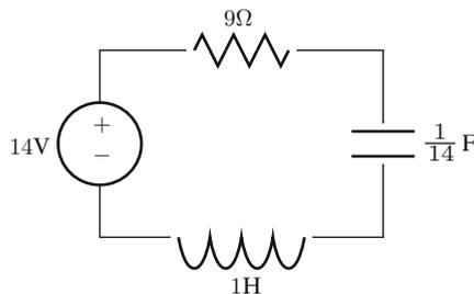
Find the charge on the capacitor at time  $t$  if the initial charge and initial current are 0. In the long term, what will be the charge on the capacitor and the current in the circuit.
