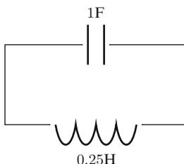
There is no voltage supply. Suppose the capacitor has a capacitance of 1 F and initial charge of  $q(0) = 0.2$  C. Suppose the inductor has inductance 0.25 H. If there is no initial current find the current,  $I(t)$ , at time  $t$ . What is the system frequency, amplitude, and phase angle? What is the charge on the capacitor at time  $t = \pi/4$ .
