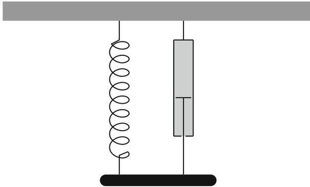
We assume the body only moves vertically without any twisting. Our goal is to determine the motion of the body in such a system. Various forces come into play. These include the force of gravity, the restoring force of the spring, the damping force of the dashpot, and perhaps an external force. Let us examine each of these forces and how they contribute to the overall motion of the body.
