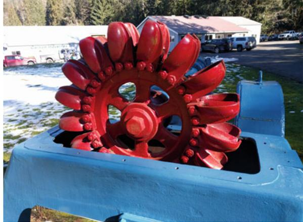
**Fig. 6.22** A 25 kW AC-coupled MHP system using a two-jet Pelton turbine (courtesy of the author)
