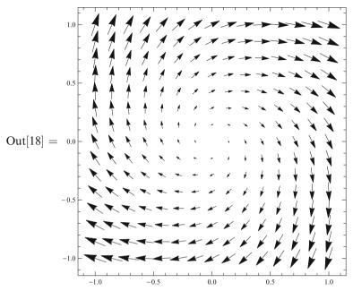
$In[19] := StreamPlot[\{y+0.5*x, -x+0.5*y\}, \{x, -1, 1\}, \{y, -1, 1\}]$
