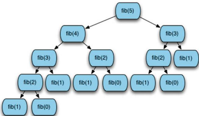
**Fig. 5.16** Calls to Calculate fib(5)
