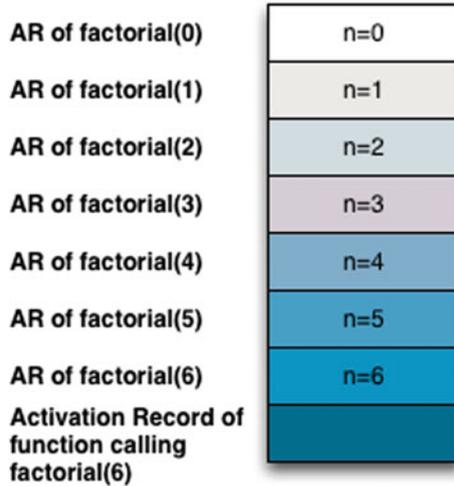
**Fig. 5.27** The run-time stack when factorial(6) is called at its deepest point
