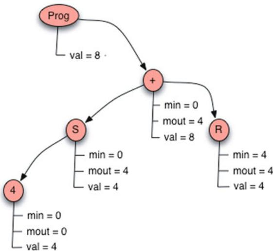
**Fig. 7.11** Annotated AST for + S 4 R
