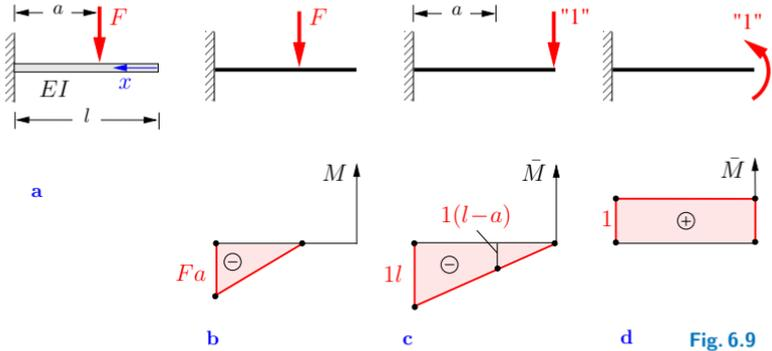
To illustrate the method we consider the cantilever beam subjected to a force  $F$  as depicted in Fig. 6.9a. We will calculate the deflection and the angle of slope at the free end. If we use the coordinate  $x$  shown in Fig. 6.9a, the bending moment caused by the given force  $F$  is (Fig. 6.9b)
