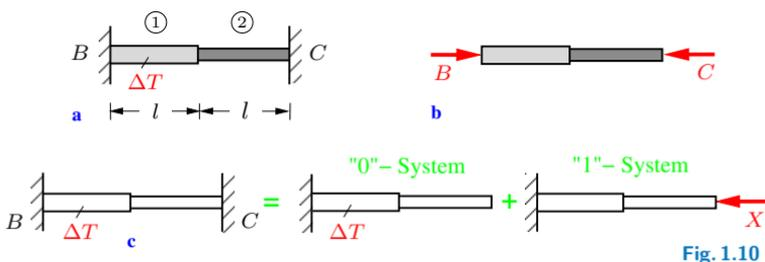
Therefore we have to take into account the deformation of the bar. The elongations in the regions ① and ② are given by (1.16) with  $N = -B = -C$ :
