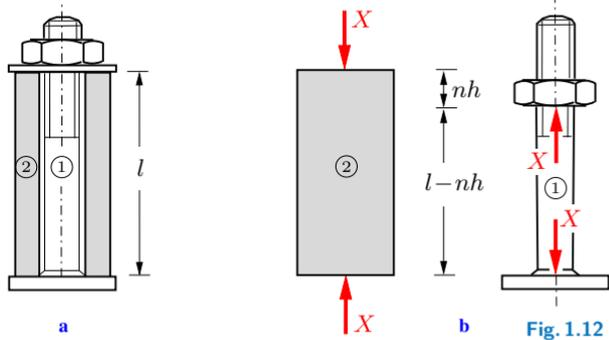
**Solution** After the nut has been turned it exerts a compressive force  $X$  on the tube which causes a shortening of the tube. According to Newton's third axiom (action = reaction) a force of equal magnitude and opposite direction acts via the nut on the bolt which elongates. The free-body diagrams of bolt and tube are shown in Fig. 1.12b.
