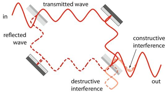
**Fig. 1.5** Classical waves in a Mach–Zehnder interferometer. Waves appearing from the second beam splitter with opposite phase cause destructive interference, resulting in a complete absence of light in that output beam. All the light appears in the output with the constructive interference. The amplitude of the wave is the square root of the intensity
