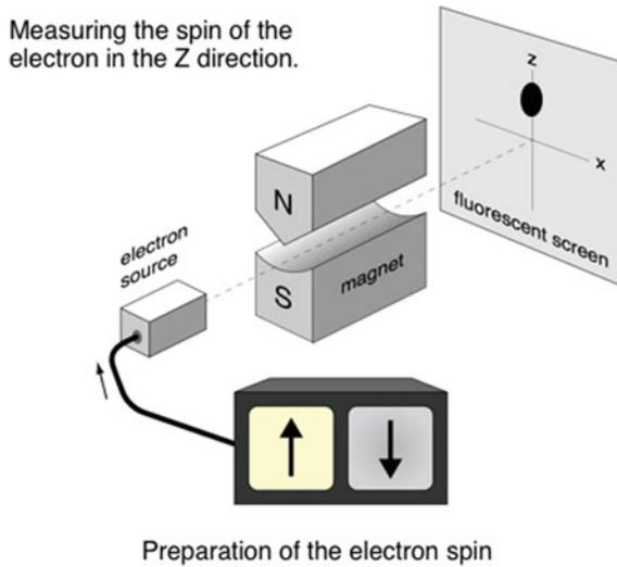
**Fig. 3.1** A Stern–Gerlach apparatus. The “up” and “down” regions on the screen where the electron is detected define the electron spin states  $|\uparrow\rangle$  and  $|\downarrow\rangle$ . The interactive figure is available online (see supplementary material 1)
