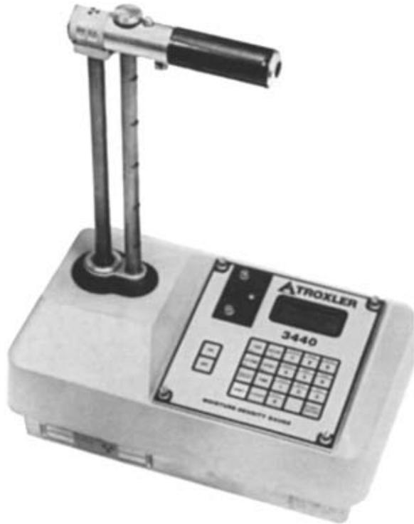
can then be found by subtracting this moisture result from the wet unit weight previously determined. Figure 4-19 illustrates several modes for using a nuclear apparatus. This method for determining *in situ* dry unit weight is known as *unit weight of soil and soil-aggregate in-place by nuclear methods* and is designated as ASTM D 2922.
