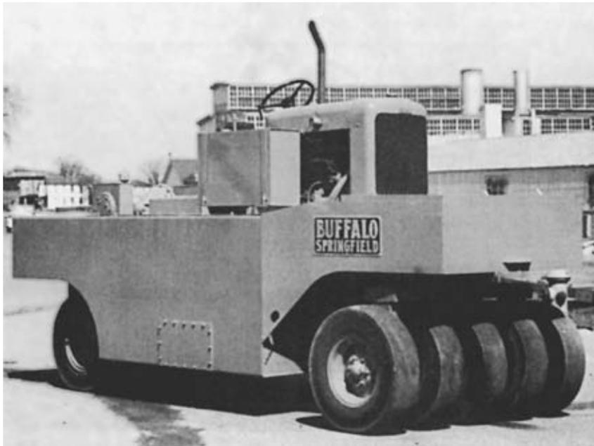
**FIGURE 4-8** Pneumatic roller.
