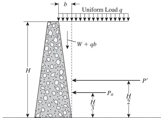
Example 12-8, which follows, illustrates the computation of pressure due to a surcharge in the form of a uniform load. Example 12-11 in Section 12-6 illustrates the treatment (graphic solution) of a surcharge in the form of a concentrated load.
