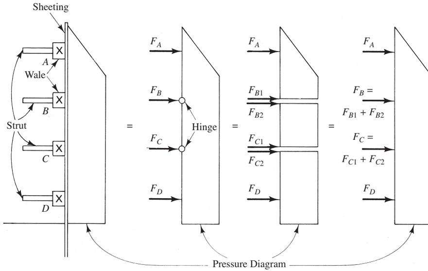
**FIGURE 12-35** Forces on struts in braced sheeting.
