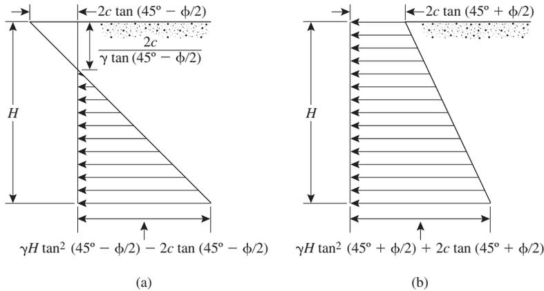
**FIGURE 12-15** Lateral earth pressure distribution for soils with cohesion and friction (Rankine theory): (a) active earth pressure; (b) passive earth pressure.
