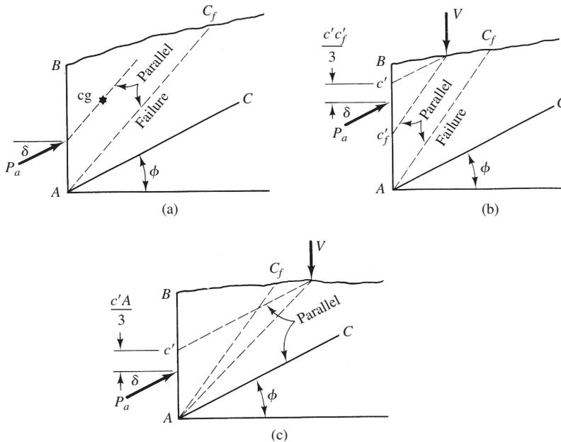
**FIGURE 12-19** Procedures for location of point of application of  $P_a$ : (a) irregular backfill; (b) concentrated or line load inside failure zone; (c) concentrated or line load outside failure zone (but inside zone ABC).
