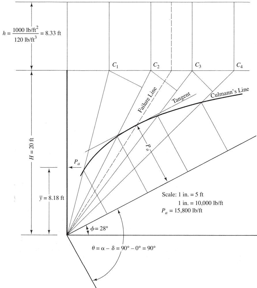
**FIGURE 12-30** Culmann's graphic solution for Example 12-10. Note: Original drawing reduced by 25%.
