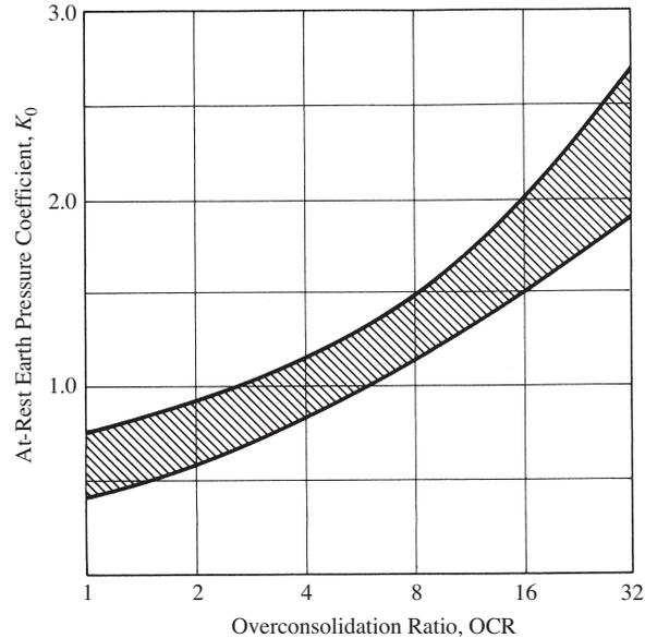
where  $PI$  is the soil's plasticity index. For overconsolidated clays, values of  $K_0$  tend to be larger than those of normally consolidated clays. Figure 12-6 gives an empirical relationship for determining  $K_0$  as a function of the overconsolidation ratio (OCR) (see Section 8-5).
