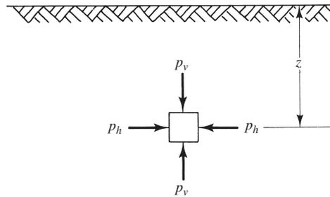
basement walls. With virtually no wall movement, soil in contact with the wall does not undergo lateral strain and does not therefore develop its full shearing resistance. In this case, the magnitude of earth pressure on the wall (i.e., the earth pressure at rest) falls somewhere between the active and passive pressures.
