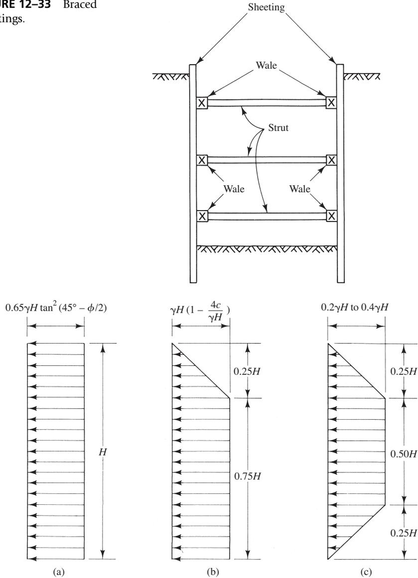
**FIGURE 12–34** Diagrams of lateral pressure against braced sheetings: (a) sand; (b) soft to medium clay; (c) stiff-fissured clay.
