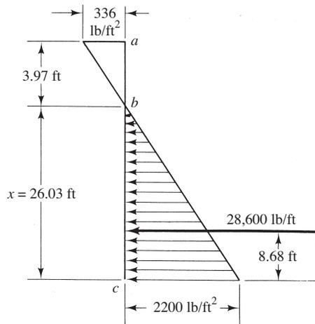
The active earth pressure diagram, based on the preceding computed values, is shown in Figure 12-17.
