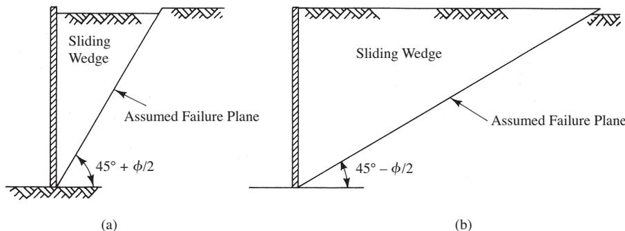
**FIGURE 12-10** Assumed failure plane for Rankine theory: (a) Rankine active state; (b) Rankine passive state.
