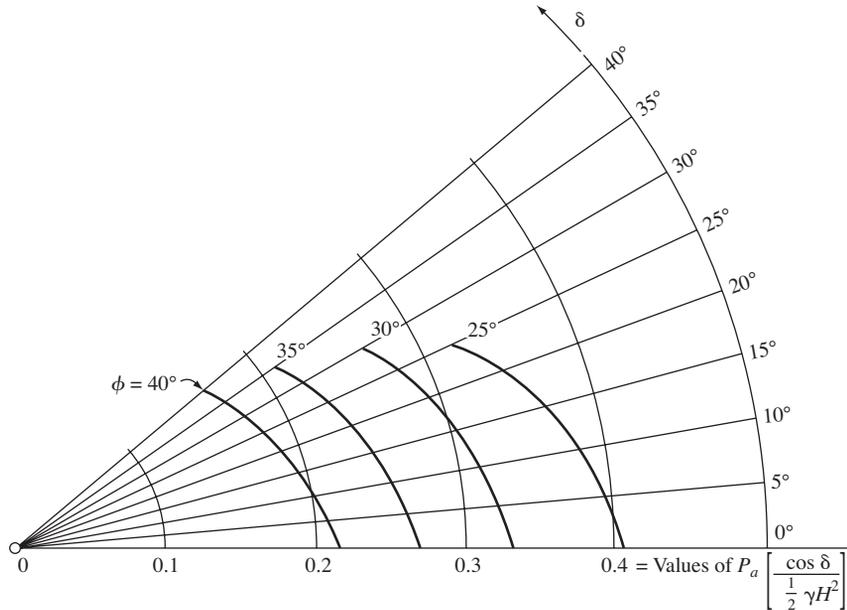
**FIGURE 12-21** Coefficients for computation of active earth pressure for vertical walls supporting cohesionless backfill with a horizontal surface.
