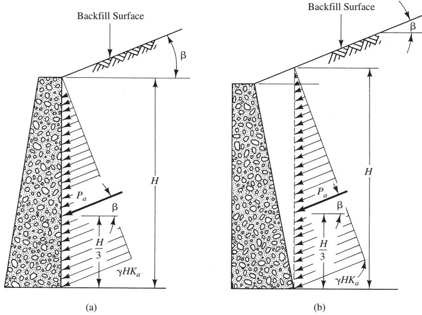
**FIGURE 12-11** Lateral earth pressure for Rankine theory: (a) back side vertical; (b) back side inclined.
