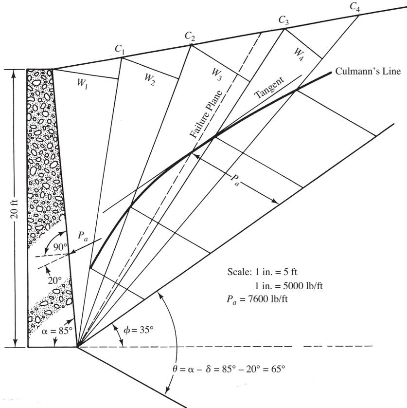
**FIGURE 12-28** Culmann's graphic solution for Example 12-9. Note: Original drawing reduced by 25%.
