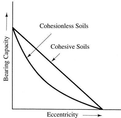
**FIGURE 9–22** Eccentric load reduction factors.
