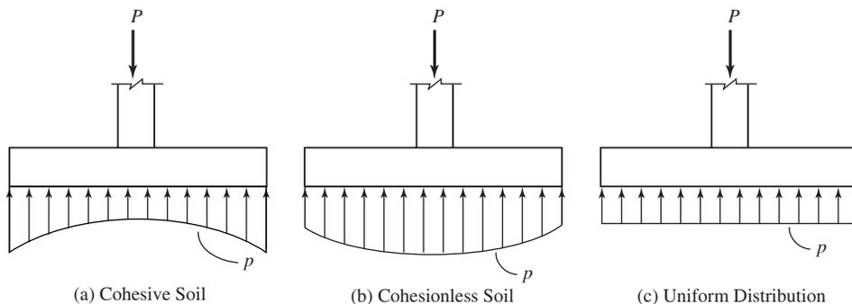
**FIGURE 9-30** Pressure distributions beneath rigid footings.
