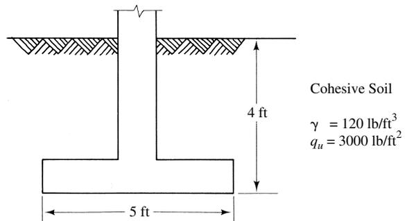
3. The subsoil consists of a thick deposit of stiff cohesive soil, with unconfined compressive strength ( $q_u$ ) equal to 3000 lb/ft<sup>2</sup>.
