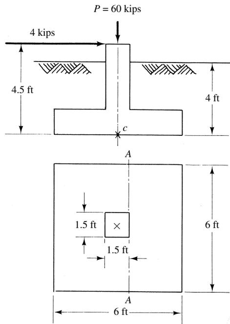
3. Factor of safety against sliding if the coefficient of friction between the footing base and the supporting soil is 0.40.
