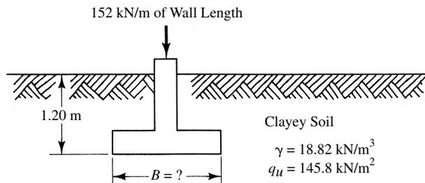
If we use  $c > 0, \phi = 0$  analysis for cohesive soil, when  $\phi = 0$ , Figure 9–7 gives
