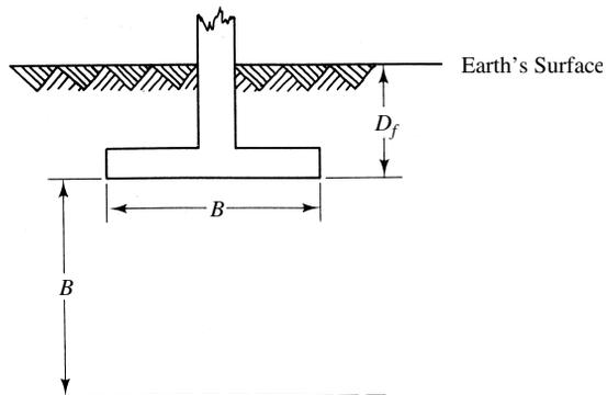
considered to vary linearly from the submerged unit weight at the footing's base to the full unit weight at distance  $B$  below the footing's base.)
