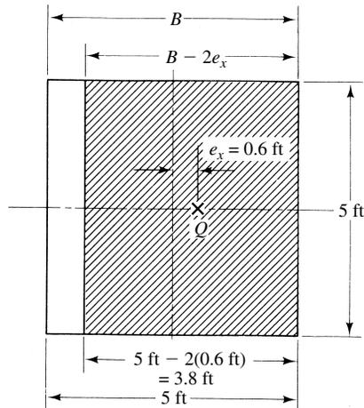
$$\begin{aligned}\gamma_1 &= \gamma_2 = 0.130 \text{ kip/ft}^3 \\ B &= \text{Useful width} = 3.8 \text{ ft} \\ q_{\text{ult}} &= (1.2)(2.0 \text{ kips/ft}^2)(5.14) + (0.130 \text{ kip/ft}^3)(4 \text{ ft})(1.0) \\ &\quad + (0.4)(0.130 \text{ kip/ft}^3)(3.8 \text{ ft})(0) = 12.9 \text{ kips/ft}^2 \\ \text{Factor of safety} &= \frac{12.9 \text{ kips/ft}^2}{\left(\frac{75 \text{ kips}}{3.8 \text{ ft} \times 5 \text{ ft}}\right)} = 3.27\end{aligned}$$
