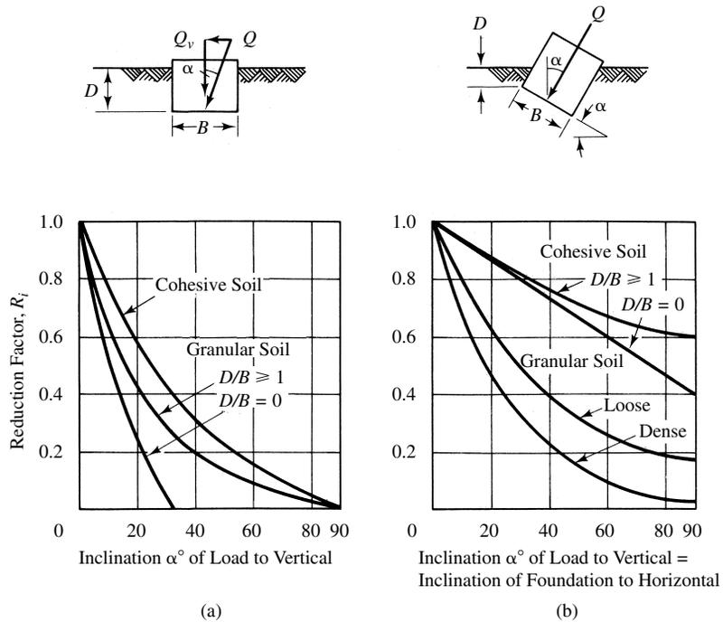
**FIGURE 9-18** Inclined load reduction factors: (a) horizontal foundation; (b) inclined foundation (Meyerhof, 1953).
