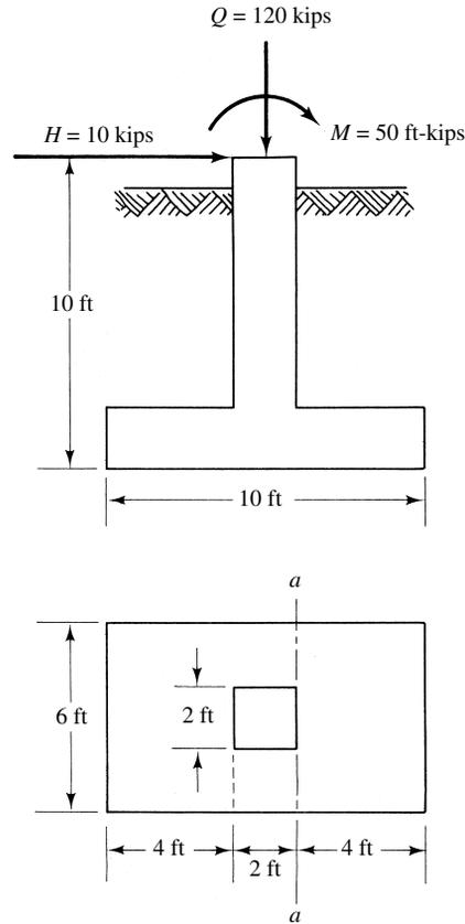
load is 10 kips, and a moment of 50 ft-kips (clockwise) is also imposed on the foundation.
