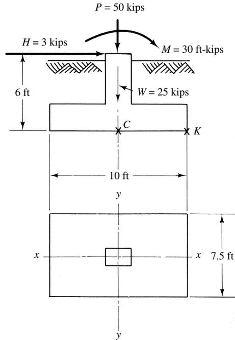
$$Q = 50 \text{ kips} + 25 \text{ kips} = 75 \text{ kips}$$
