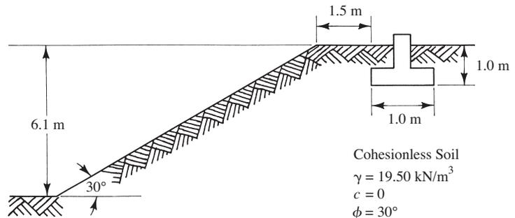
$$\frac{D_f}{B} = \frac{1.0 \text{ m}}{1.0 \text{ m}} = 1.0 \text{ (use the dashed line)}$$
