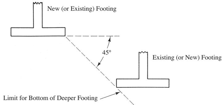
or lowering of the water table. After new foundations have been constructed, the (new) load they place on the soil may cause settlement of previously existing structures as a result of new stress patterns in the surrounding soil.
