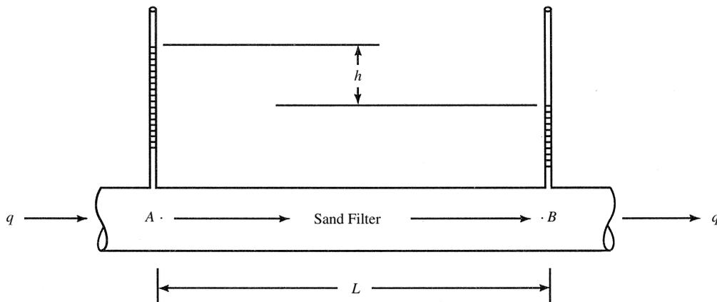
**FIGURE 5-1** Illustration of Darcy's experiment.
