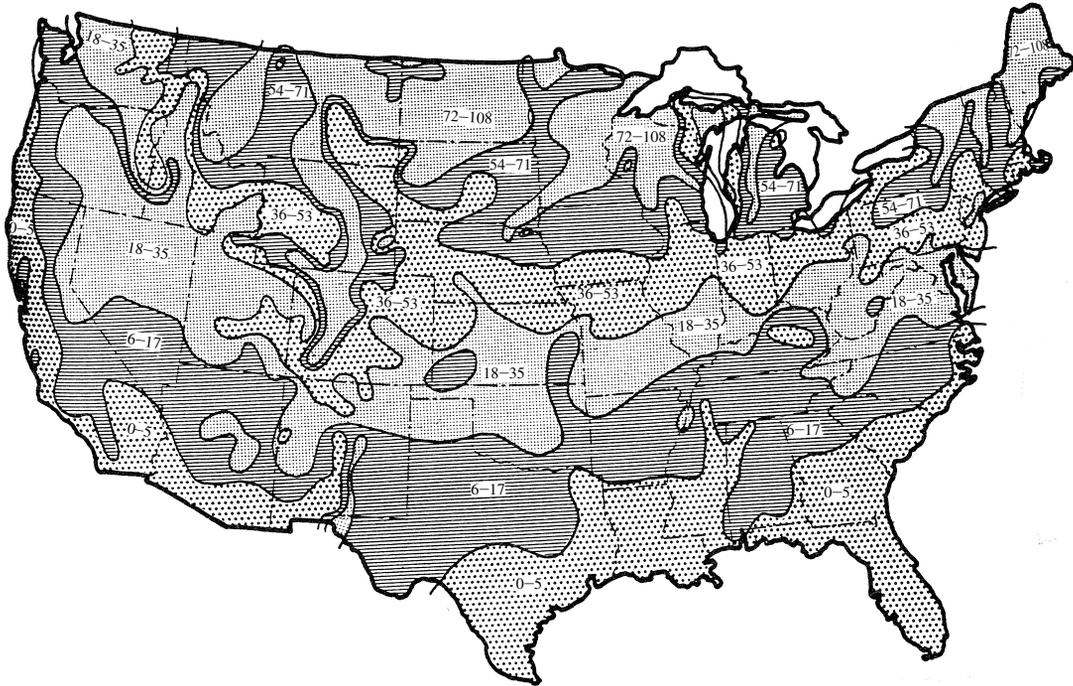
**FIGURE 5-9** Maximum depth of frost penetration in the United States.
