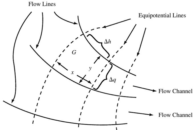
Consider one square in a flow net—for example, the one labeled  $G$  in Figure 5-12. Let  $\Delta q$  and  $\Delta h$  denote the flow rate and drop in head (energy), respectively, for this square. Because each square is  $x$  units wide and  $y$  units long and has a unit width perpendicular to the figure, term  $i$  in Eq. (5-2) is given by  $\Delta h/x$ , and term  $A$  is equal to  $y$ . Hence,
