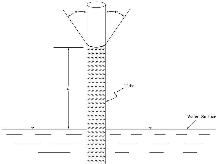
FIGURE 5-8 Capillary rise of water in a tube.
