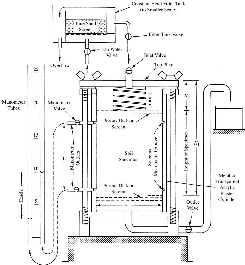
**FIGURE 5-2** Constant-head permeameter.
