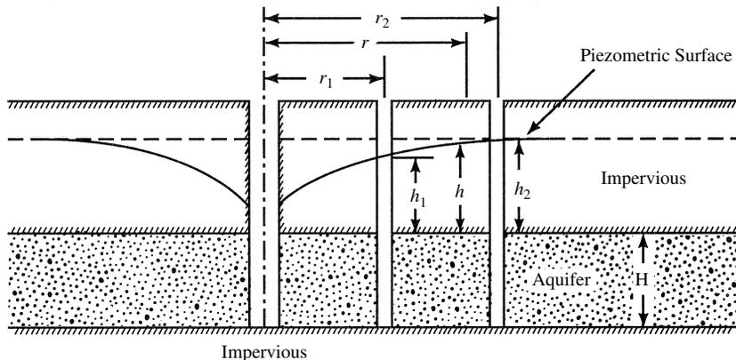
**FIGURE 5-4** Flow of water toward pumping well (confined aquifer).
