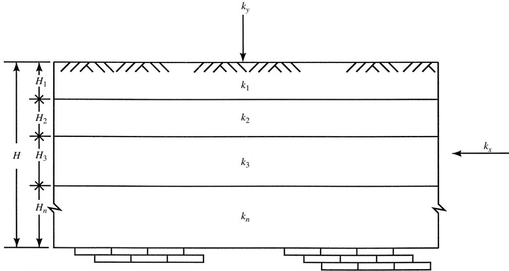
**FIGURE 5-6** Stratified soil consisting of layers with various permeabilities.
