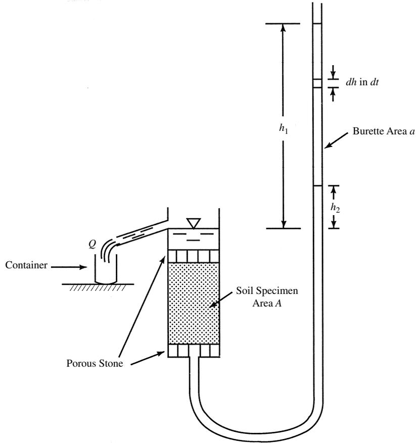
**FIGURE 5-3** Schematic of the falling-head permeability setup.
