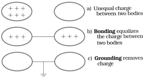
Figure 12-3. Grounding compared with bonding.
