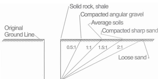
Figure 10-12. Slopes of sides of excavations recommended by OSHA.
