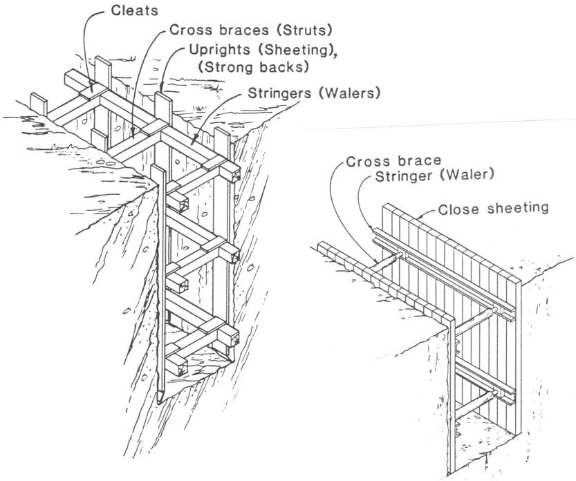
Figure 10-10. Examples of trench shoring and the components involved.
