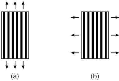
**FIGURE 11.13** Patterns of loading continuously aligned fiber-reinforced composites: (a) loading parallel to fibers and (b) loading perpendicular to fibers.
