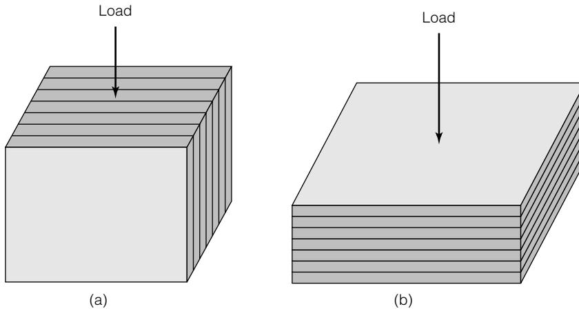
**FIGURE 10.18** Axis convention used for defining loading conditions for Laminated Veneer Lumber.
