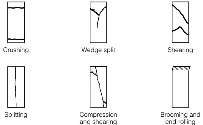
**FIGURE 10.12** Types of failure in the compression-parallel-to-grain test. (ASTM D143). Reprinted with permission of ASTM.
