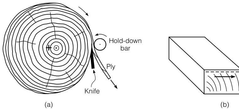
**FIGURE 10.14** Cutting of plies for plywood and glulam: (a) rotary cutting and (b) slicing (© Pearson Education, Inc. Used by permission.)
