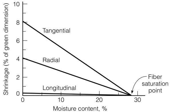
**FIGURE 10.5** Relation between shrinkage and moisture content.
