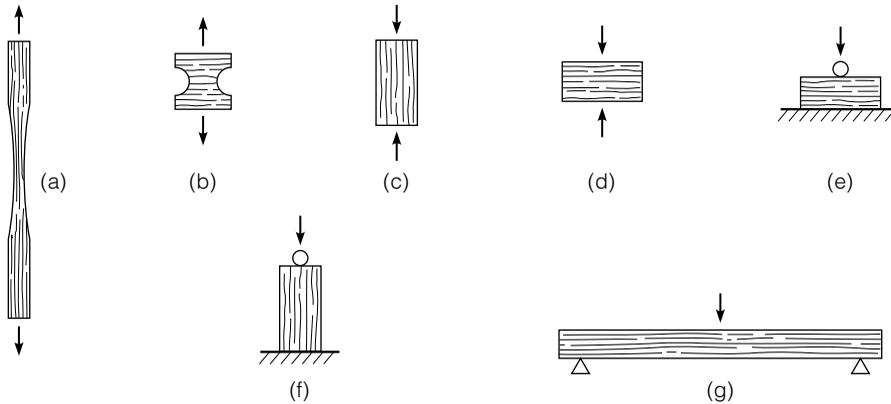
**FIGURE 10.10** Test specimens of wood: (a) tension parallel to grains, (b) tension perpendicular to grains, (c) compression parallel to grains, (d) compression perpendicular to grains, (e) hardness perpendicular to grains, (f) hardness parallel to grains, and (g) bending. (© Pearson Education, Inc. Used by permission.)
