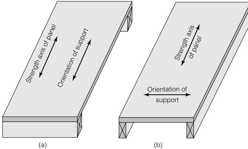
FIGURE 10.16 Strength axis of plywood.
