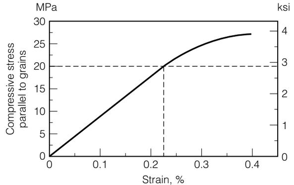
**FIGURE 10.9** Typical stress strain relationship for wood.
