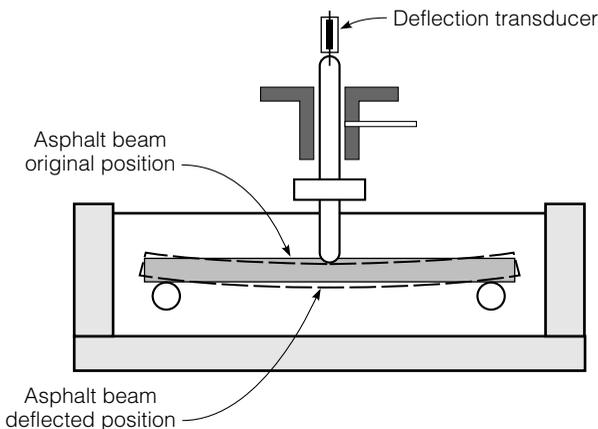
**FIGURE 9.17** Schematic of the bending beam rheometer.
