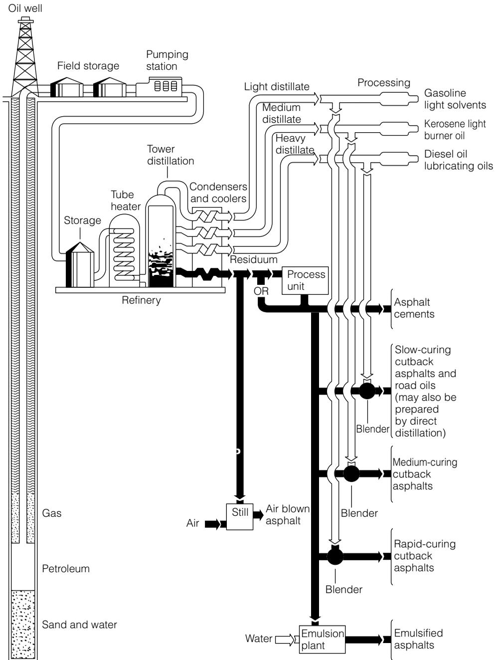
FIGURE 9.2 Distillation of crude petroleum. (The Asphalt Institute 1989).
