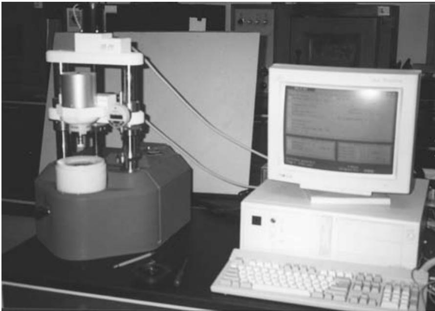
**FIGURE 9.16** Dynamic shear rheometer apparatus.
