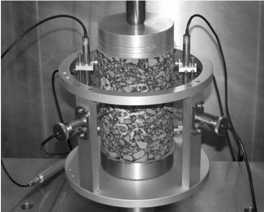
FIGURE 9.28 Superpave simple performance test assembly.
