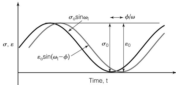
FIGURE 9.29 Stress and strain pulses for the dynamic modulus test.
