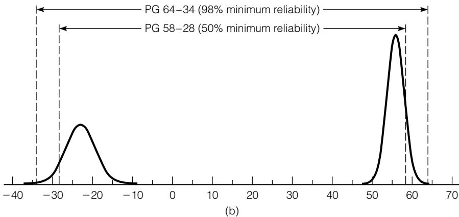
**FIGURE 9.22** Example of the distribution of design pavement temperatures and selection of binder grades: (a) distribution of high and low design pavement temperatures, and (b) binder grade selection.
