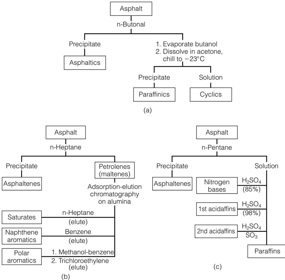
**FIGURE 9.11** Schematic diagrams of three asphalt fractionation schemes: (a) partitioning with partial solvents, (b) selective-adsorption-desorption, and (c) chemical precipitation (Peterson 1984).
