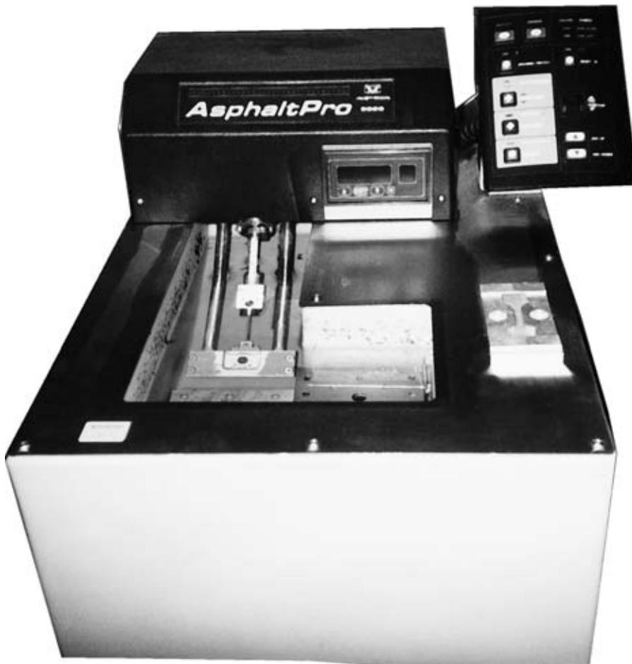
**FIGURE 9.18** Direct tension test apparatus.
