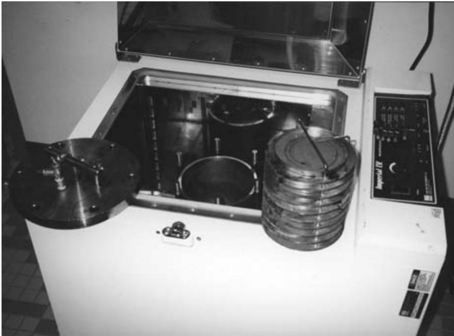
**FIGURE 9.13** Pressure aging vessel apparatus.
