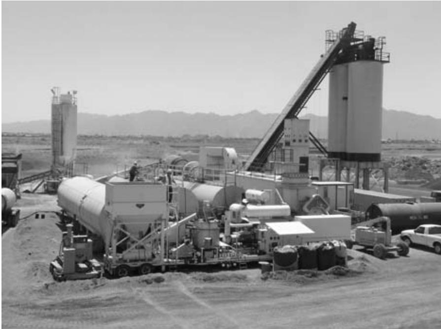
FIGURE 9.38 Continuous (drum) mix asphalt concrete plant.
