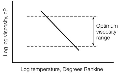
**FIGURE 9.7** Typical relation between asphalt viscosity and temperature.
