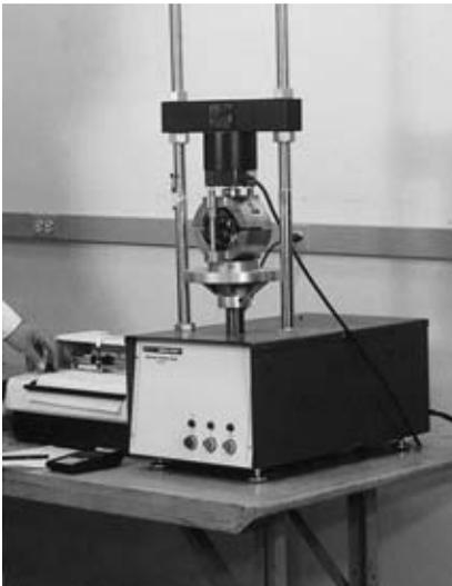
FIGURE 9.32 Marshall stability machine.
