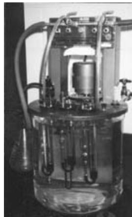
FIGURE 9.20 Absolute viscosity test apparatus.
