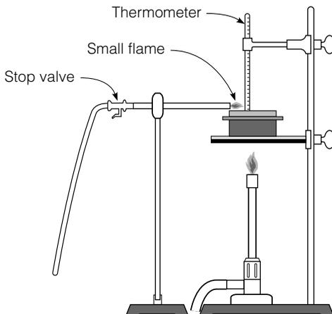
**FIGURE 9.14** Cleveland open cup flash point test apparatus.
