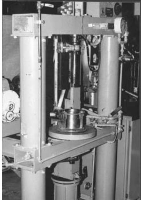
**FIGURE 9.25** California kneading compactor.
