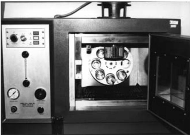
**FIGURE 9.12** Rolling thin film oven test apparatus.
