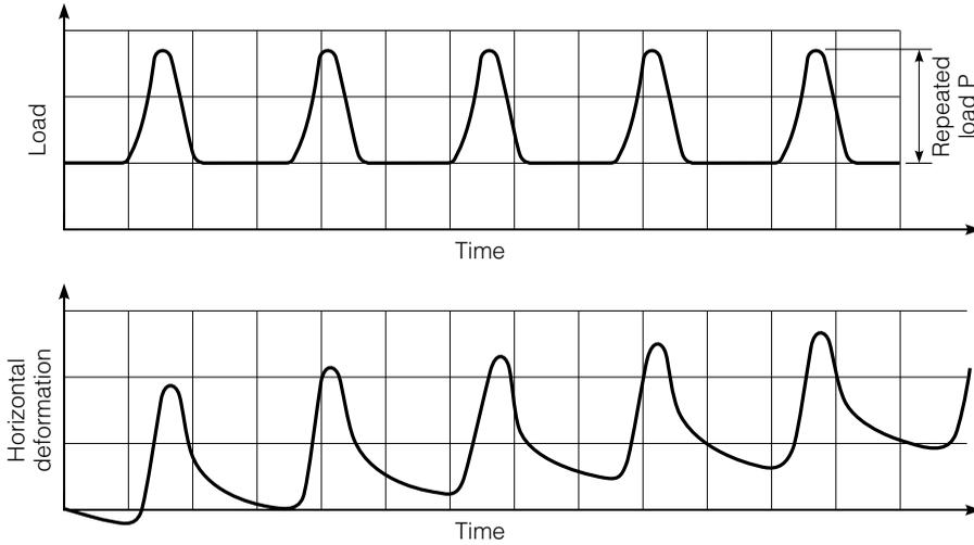
**FIGURE 9.37** Typical load and horizontal deformation versus time during the resilient modulus test.
