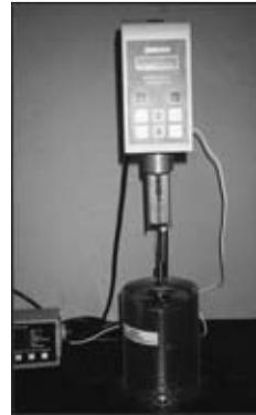
**FIGURE 9.15** Rotational viscometer.
