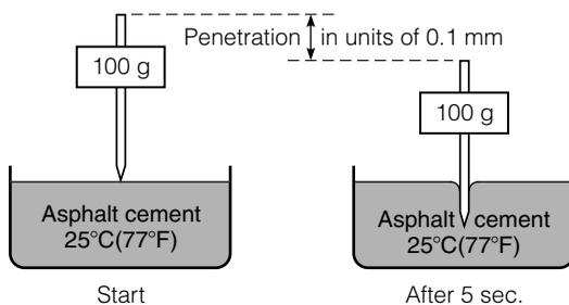
FIGURE 9.19 Penetration test.
