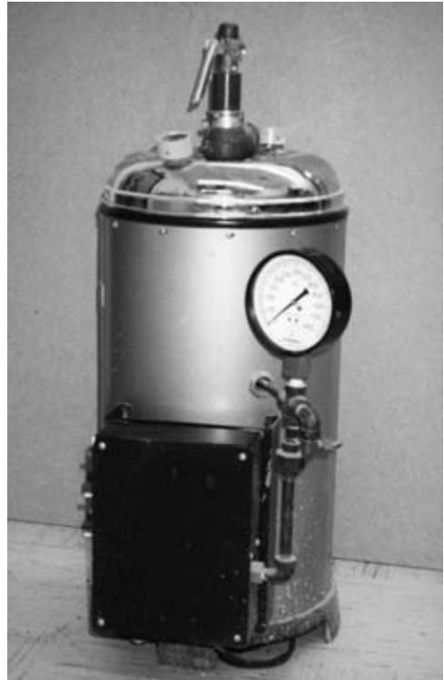
**FIGURE 6.6** Cement autoclave expansion apparatus.
