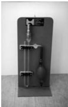
FIGURE 6.2 Blaine air permeability apparatus.
