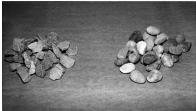
**FIGURE 5.4** Angular and rounded aggregates.
