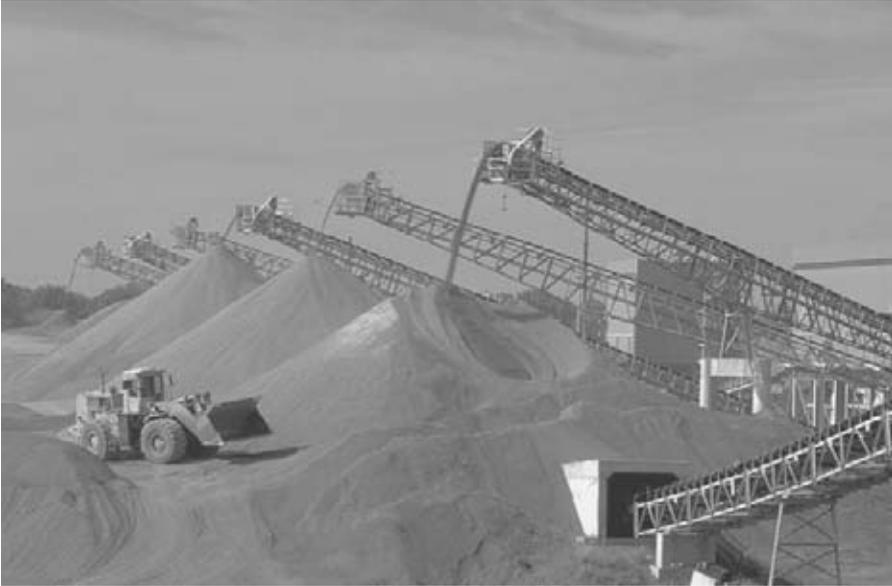
FIGURE 5.1 Aggregate stockpiling.
