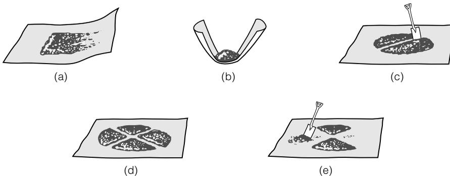
**FIGURE 5.18** Steps for reducing the sample size by quartering: (a) mixing by rolling on blanket, (b) forming a cone after mixing, (c) flattening the cone and quartering, (d) finishing quartering, (e) retaining opposite quarters (the other two quarters are rejected). (ASTM C702). Copyright ASTM. Reprinted with permission.
