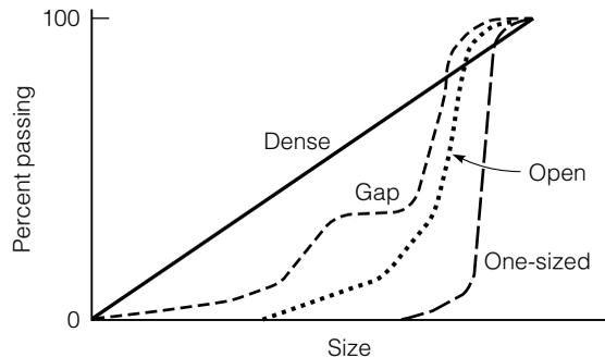
**FIGURE 5.13** Types of aggregate grain size distributions plotted on a 0.45 gradation chart.
