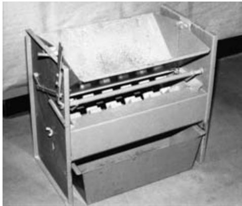
**FIGURE 5.17** Aggregate sample splitter.
