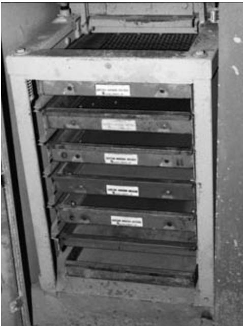
**FIGURE 5.10** Sieve shaker for large samples of aggregates.
