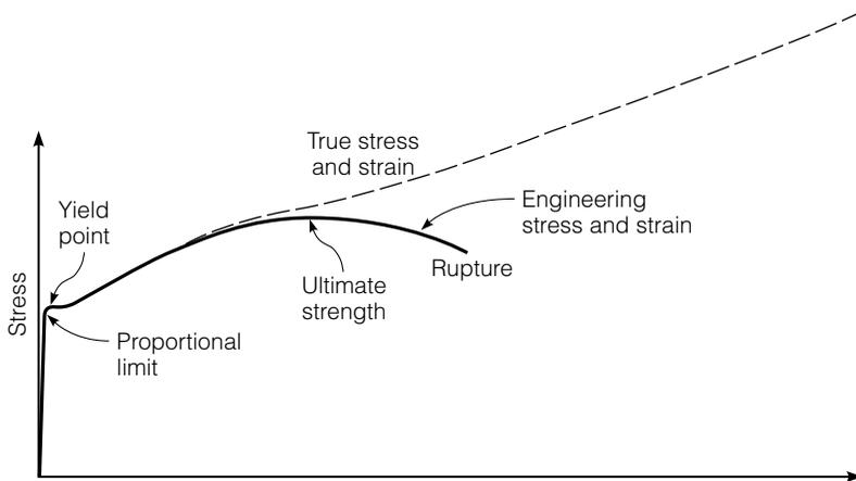
**FIGURE 3.13** Typical stress-strain behavior of mild steel.
