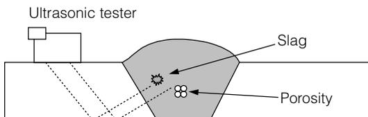
**FIGURE 3.23** Ultrasonic test of welds.
