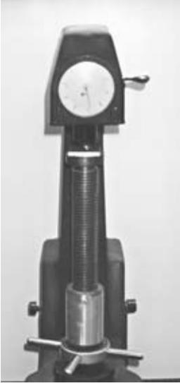
**FIGURE 3.22** Rockwell hardness test machine.
