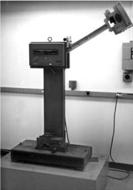
**FIGURE 3.19** Charpy V notch impact testing machine.
