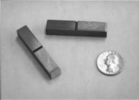
**FIGURE 3.18** Charpy V notch specimens.
