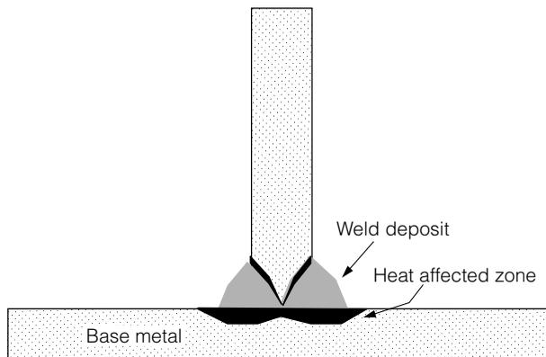
**FIGURE 3.27** Heat affected zone produced during welding.
