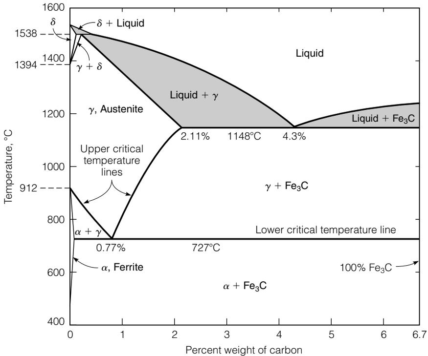
**FIGURE 3.4** The iron–iron carbide phase diagram.
