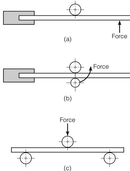
**FIGURE 3.21** Schematic fixtures for semi-guided bend test (ASTM E290). Copyright ASTM. Reprinted with permission.
