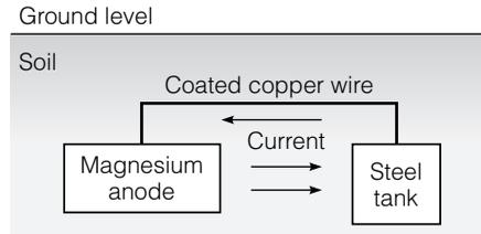
3. *Sacrificial primers (cathodic protection)* contain pigments such as elemental zinc. Since zinc is higher than iron in the galvanic series, when corrosion conditions exist the zinc gives up electrons to the steel, becomes the anode, and corrodes to protect the steel. There should be close contact between the steel and the sacrificial primer in order to have an effective corrosion protection.
