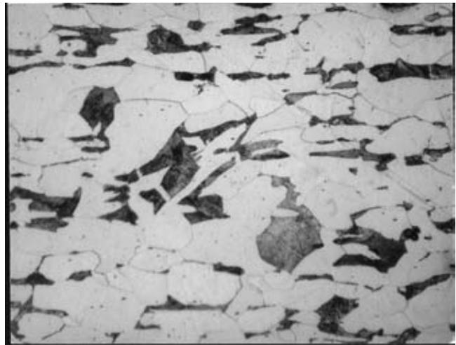
**FIGURE 3.6** Optical photomicrograph of hot rolled mild steel plate (magnification: 400x).
