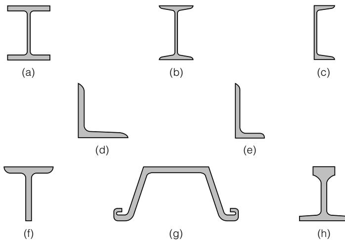
**FIGURE 3.9** Shapes commonly used in structural applications: (a) wide-flange (W, HP, and M shapes), (b) I-beam (S shape), (c) channel (C and MC shapes), (d) equal-legs angle (L shape), (e) unequal-legs angle (L shape), (f) tee, (g) sheet piling, and (h) rail.
