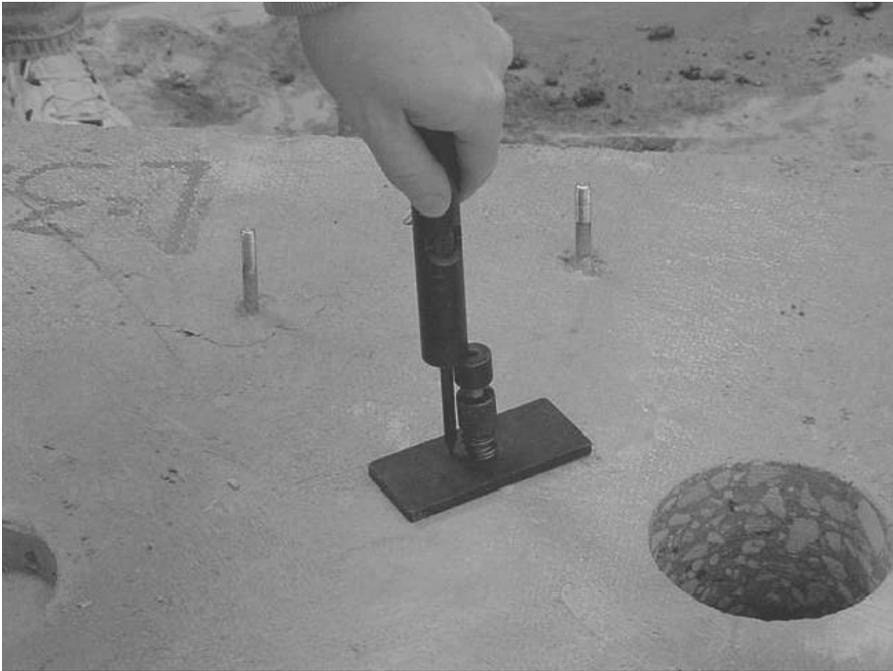
FIGURE A.45 Measuring penetration of one probe.
