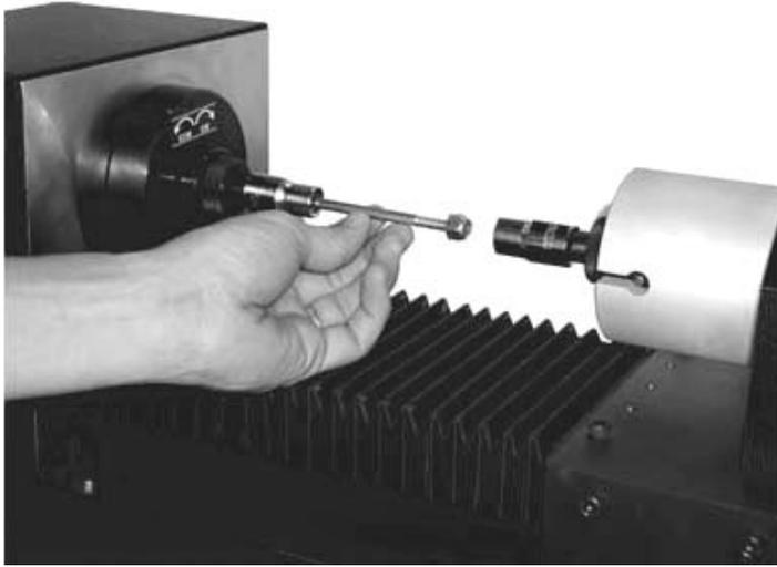
**FIGURE A.11** Placing specimen in torsion machine.
