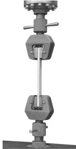
**FIGURE A.67** Tension test on a plastic specimen.
