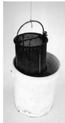
**FIGURE A.23** Wire basket and water tank used to determine bulk specific gravity and absorption of coarse aggregate.
