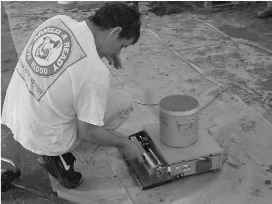
**FIGURE A.30** Weighing concrete inside the measure.
