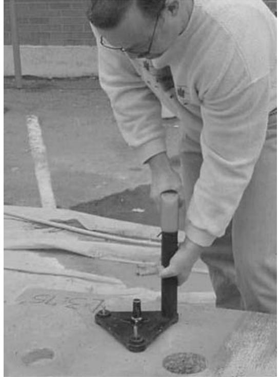
**FIGURE A.43** Firing and driving Windsor probe into concrete using triangular positioning device.
