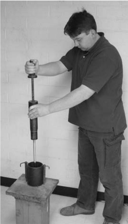
**FIGURE A.56** Compacting an HMA specimen using a manual Marshall hammer.
