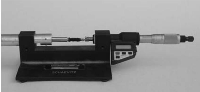
**FIGURE A.5** Calibrating an LVDT with a micrometer using a calibration device.
