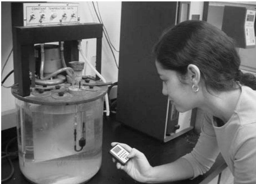
FIGURE A.51 Measuring flow time using a stop watch.
