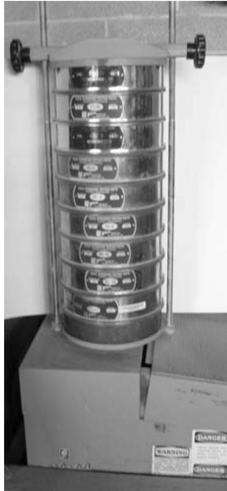
**FIGURE A.17** Table-top sieve shaker and sieves.
