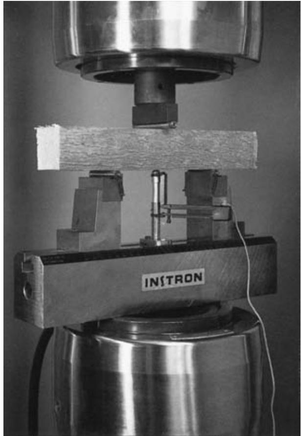
**FIGURE A.63** Wood specimen during static bending test.
