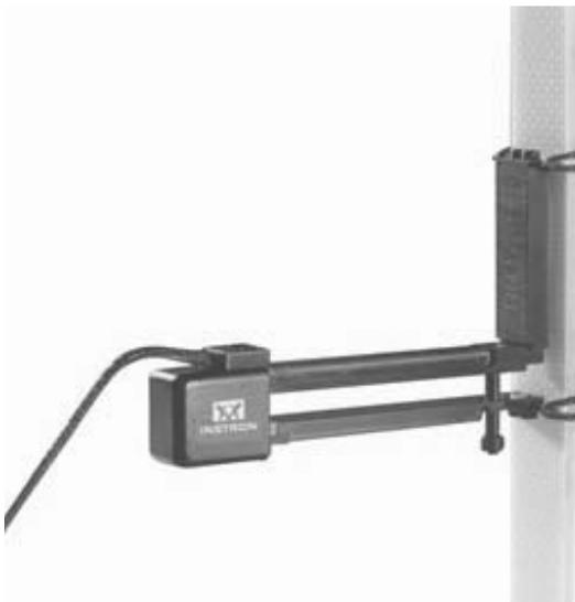
**FIGURE A.66** Extensometer on plastic specimen.
