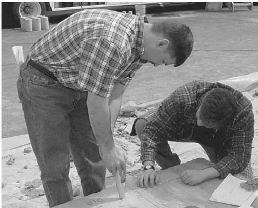
**FIGURE A.42** Testing concrete slab with a rebound hammer.
