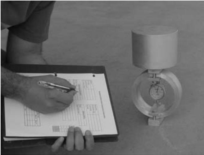
**FIGURE A.3** Calibrating a proving ring using a known-weight object.
