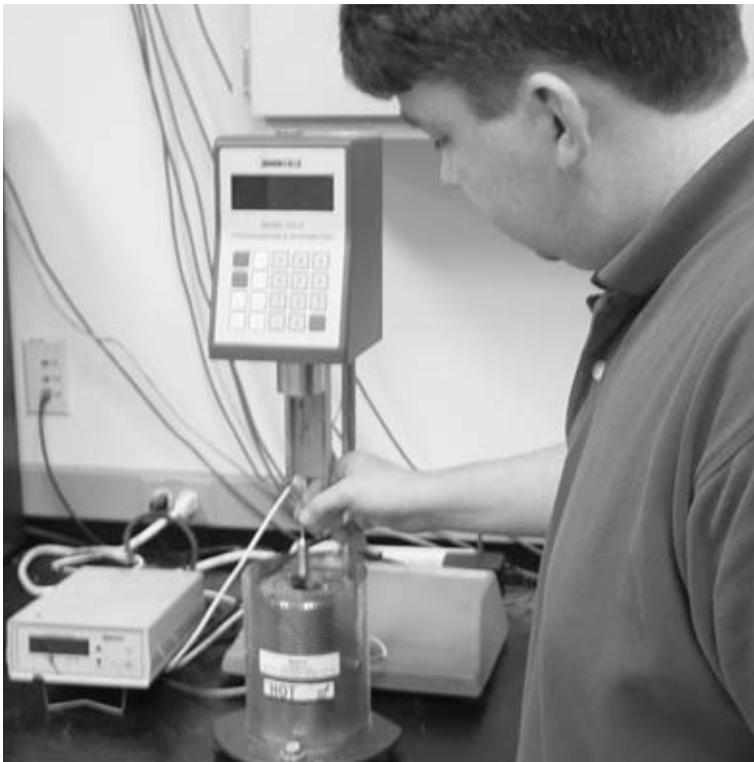
**FIGURE A.47** Inserting the spindle into chamber before the rotational viscometer test.
