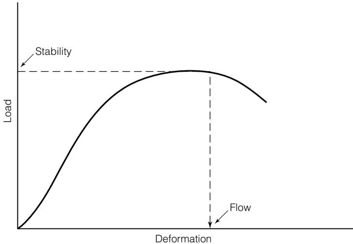
**FIGURE A.62** Typical plot of load versus deformation during the Marshall stability test showing the stability and flow.
