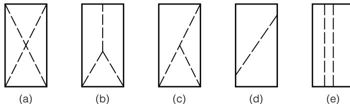
**FIGURE A.40** Types of fracture of concrete cylinders: (a) cone, (b) cone and split, (c) cone and shear, (d) shear, and (e) columnar.
