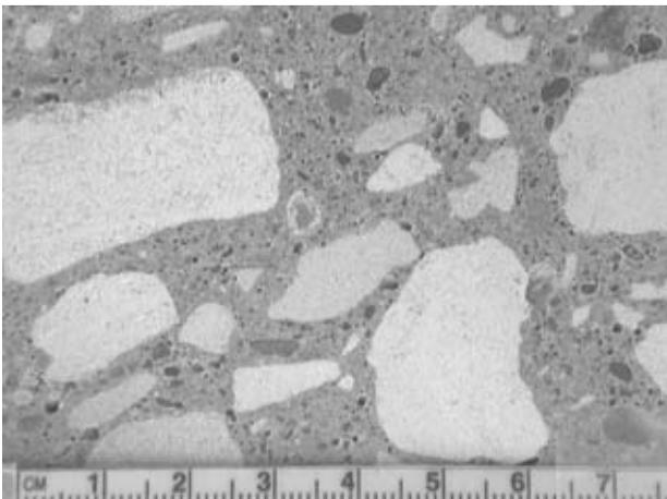
**FIGURE A.15** Concrete microstructure using optical microscope.
