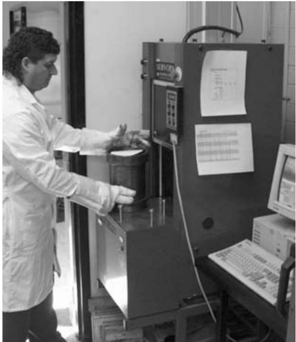
**FIGURE A.53** Placing the mold in the gyratory compactor.
