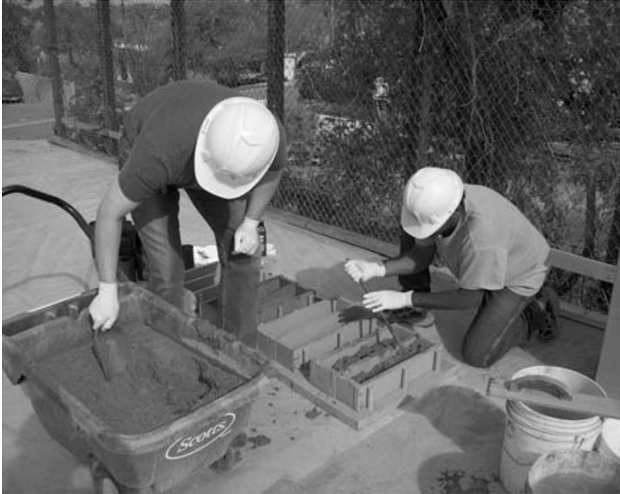
**FIGURE A.34** Filling and rodding concrete in beams.
