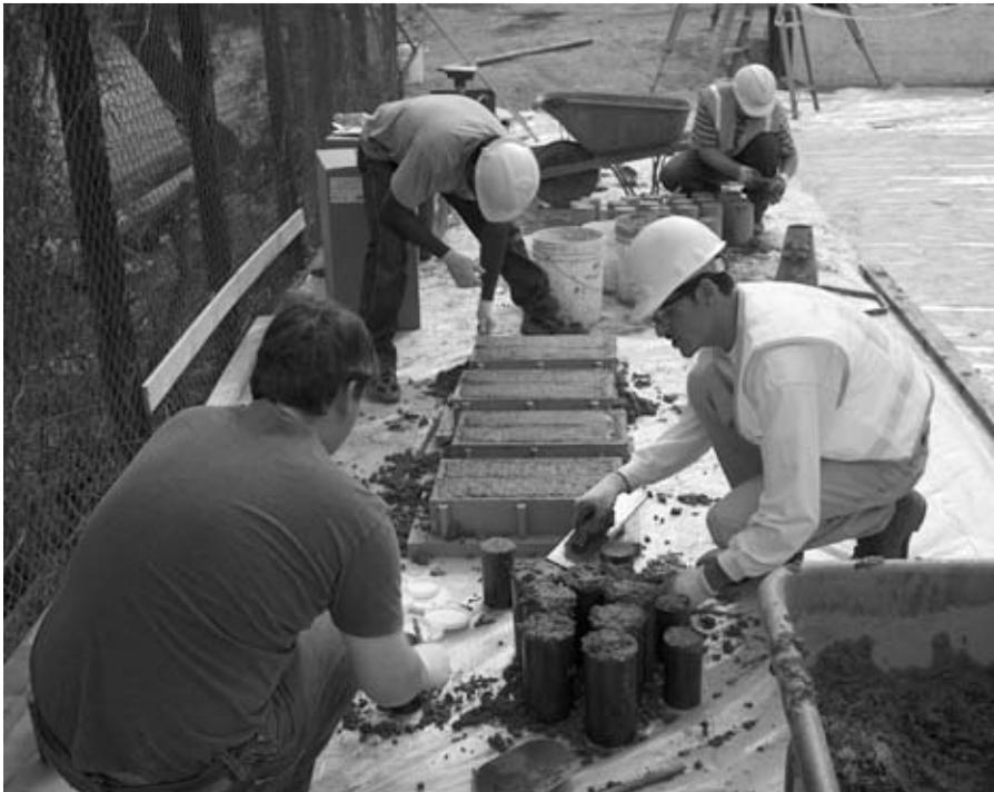
**FIGURE A.33** Making concrete cylinders and beams.
