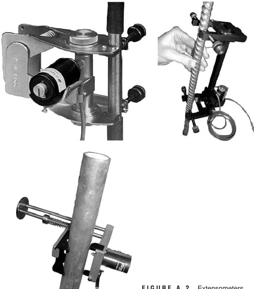
FIGURE A.2 Extensometers.
