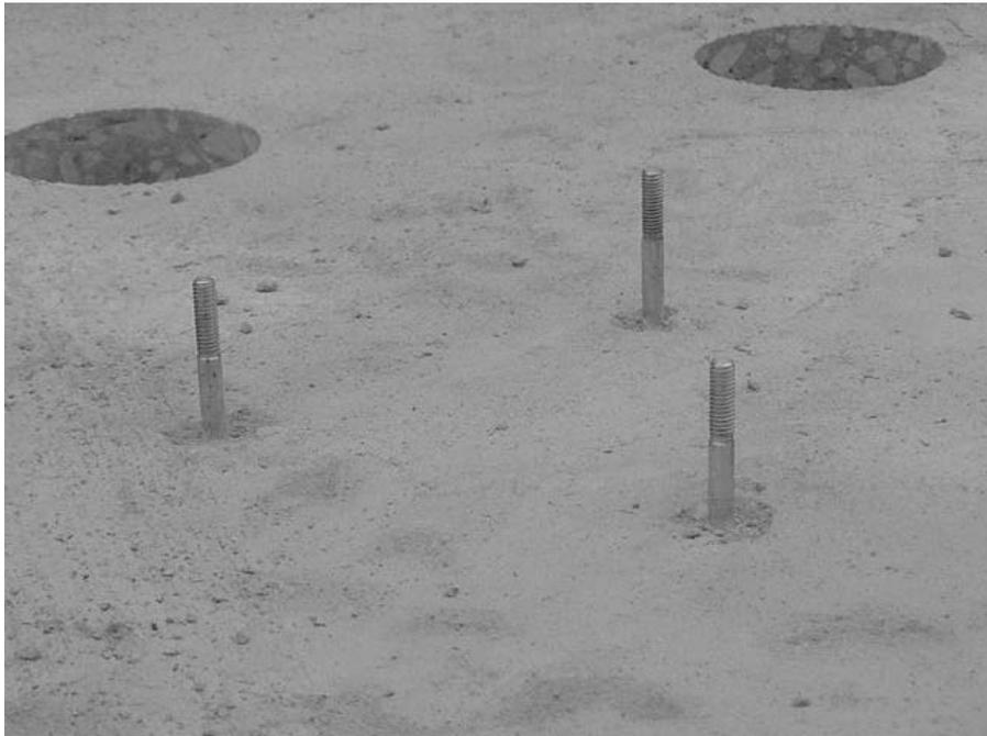
**FIGURE A.44** Three probes driven into concrete.
