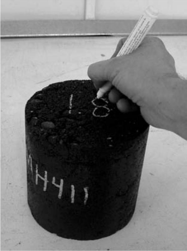
**FIGURE A.54** Specimen prepared with gyratory shear compactor
