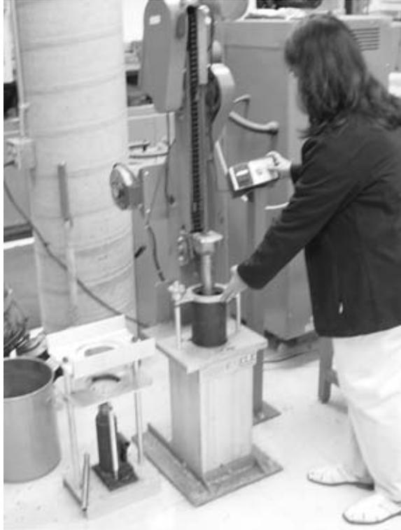
**FIGURE A.57** Compacting an HMA specimen using a mechanical Marshall hammer.
