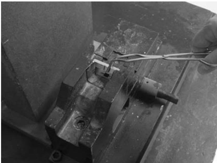
**FIGURE A . 14** Placing specimen in Charpy machine.
