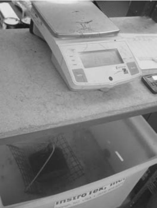
**FIGURE A.60** Weighing HMA specimen in water.
