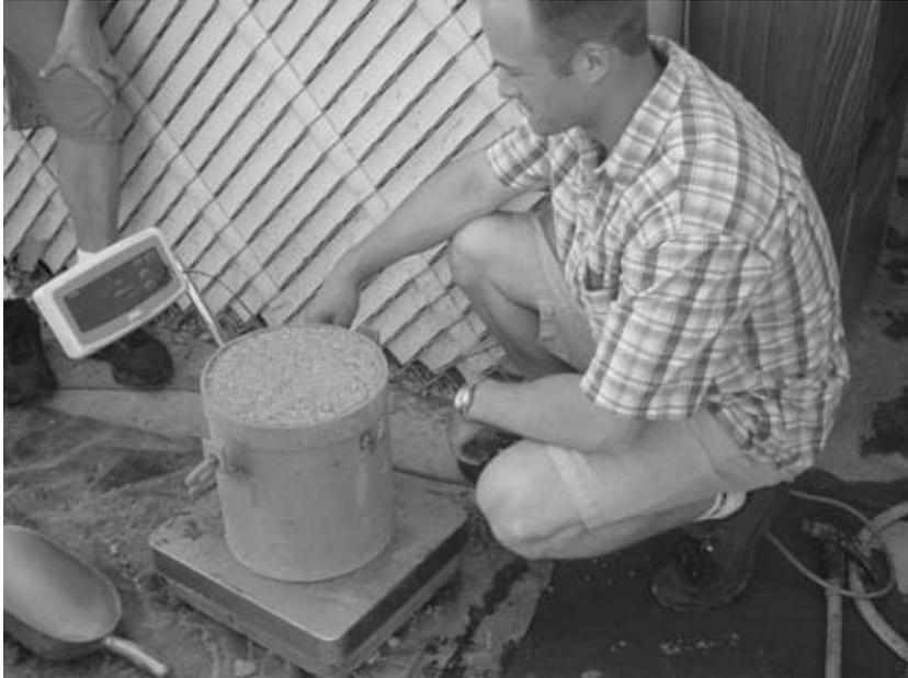
FIGURE A.26 Weighing the aggregate.
