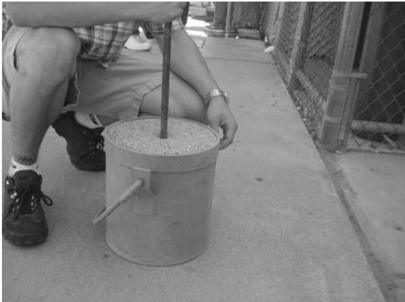
**FIGURE A.25** Rodding aggregate in the measure.
