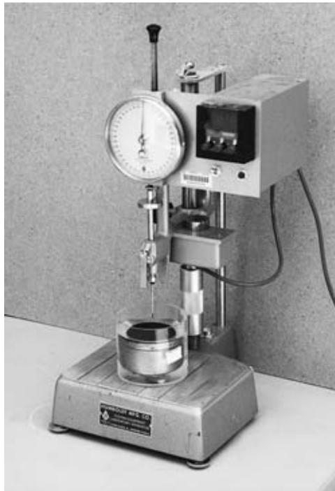
**FIGURE A.50** Apparatus for penetration test of asphalt binder.
