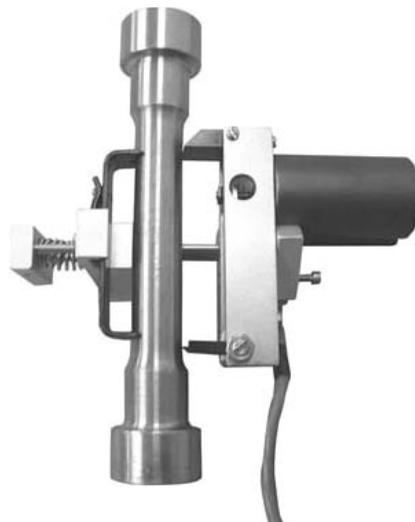
**FIGURE A.7** Extensometer attached to a steel specimen.
