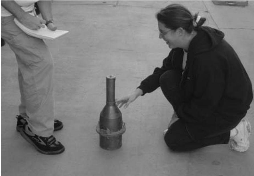
FIGURE A.32 Reading air meter.
