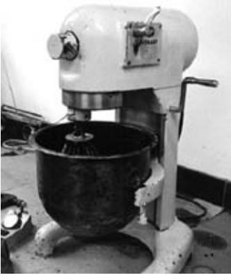
**FIGURE A.55** Mixing HMA using a mechanical mixer.
