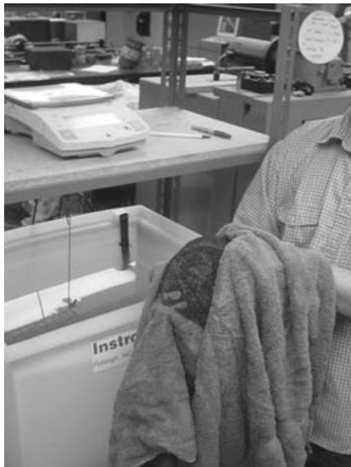
**FIGURE A.61** Removing surface water of HMA specimen with a damp towel.
