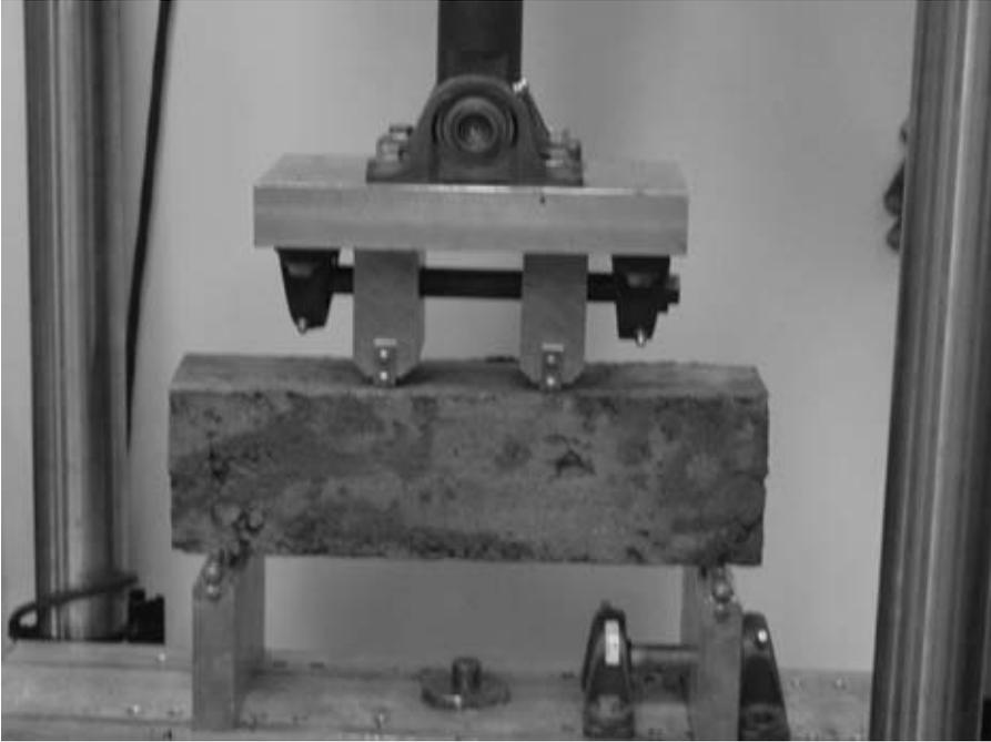
**FIGURE A.41** Testing concrete beam in the flexure testing machine.
