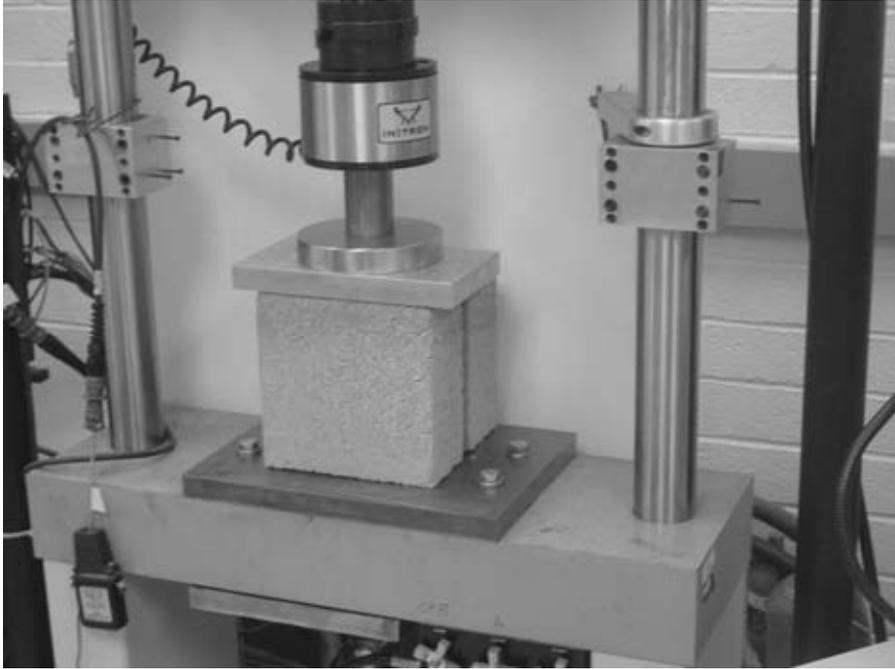
**FIGURE A.46** Compression testing of a concrete masonry unit.
