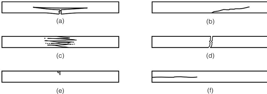
**FIGURE A.64** Types of failure in static bending: (a) simple tension (side view), (b) cross-grain tension (side view), (c) splintering tension (view of tension surface), (d) brash tension (view of tension surface), (e) compression (side view), and (f) horizontal shear (side view).
