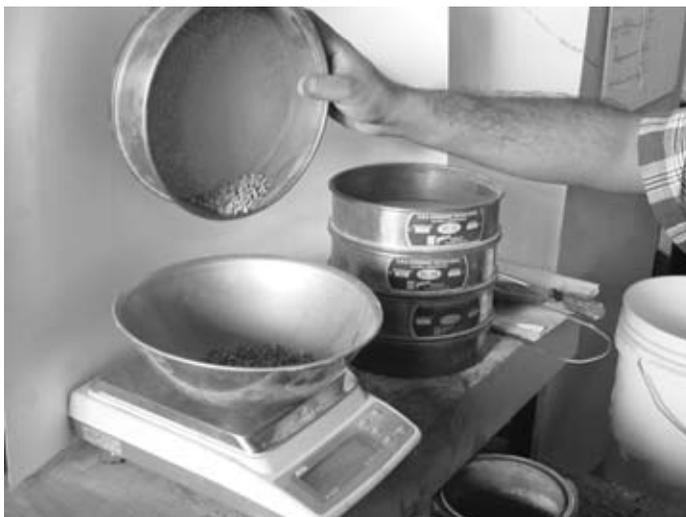
**FIGURE A.20** Weighing aggregate retained in sieves.
