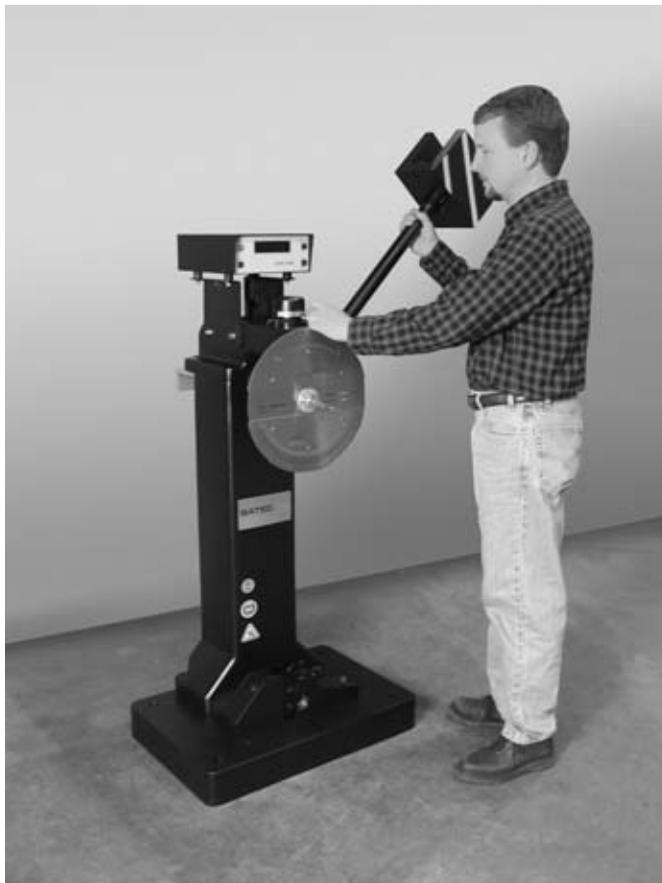
**FIGURE A.12** Charpy V notch impact testing machine.
