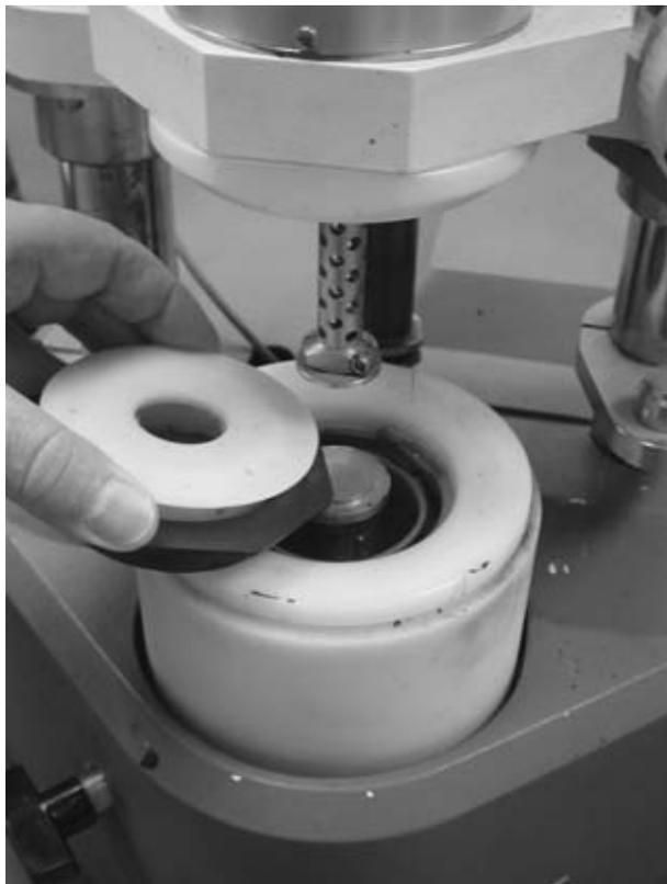
**FIGURE A.49** Water bath for controlling specimen temperature during testing.
