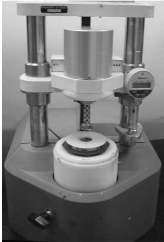
**FIGURE A.48** Dynamic shear rheometer apparatus.
