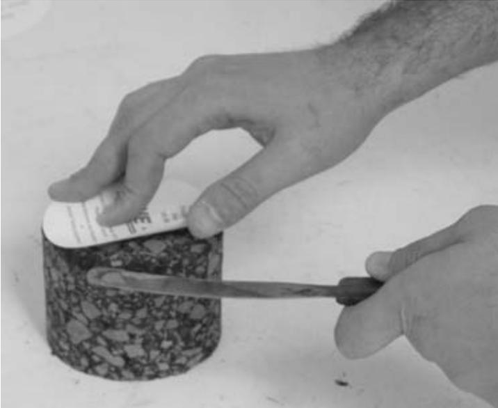
**FIGURE A.58** Removing paper disk from a Marshall plug.
