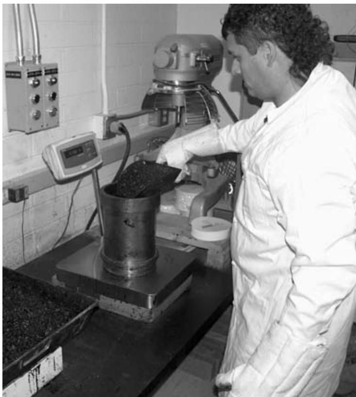
**FIGURE A.52** Placing HMA in mold.
