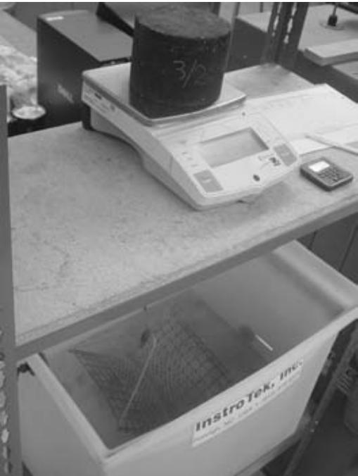
**FIGURE A.59** Weighing HMA specimen in air.
