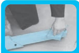
**STEP 3** Many pads at the end of the hoist arms can be rotated to allow for many different types of vehicle construction.
