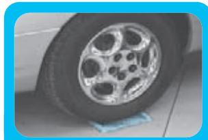
**STEP 2** Most vehicles will be correctly positioned when the left front tire is centered on the tire pad.
