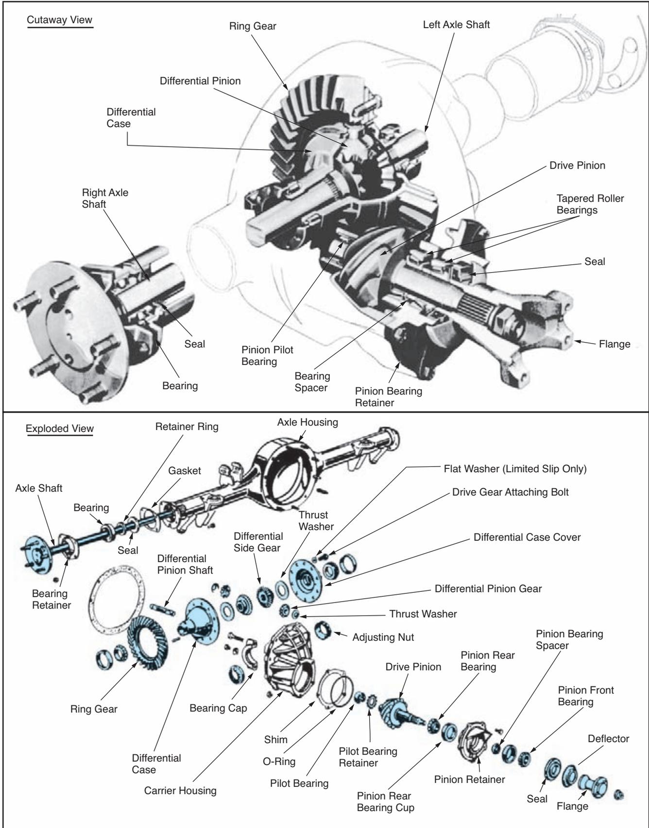
**FIGURE 11-9** Cutaway and exploded views of a removable carrier axle. (Courtesy of Ford Motor Company)
