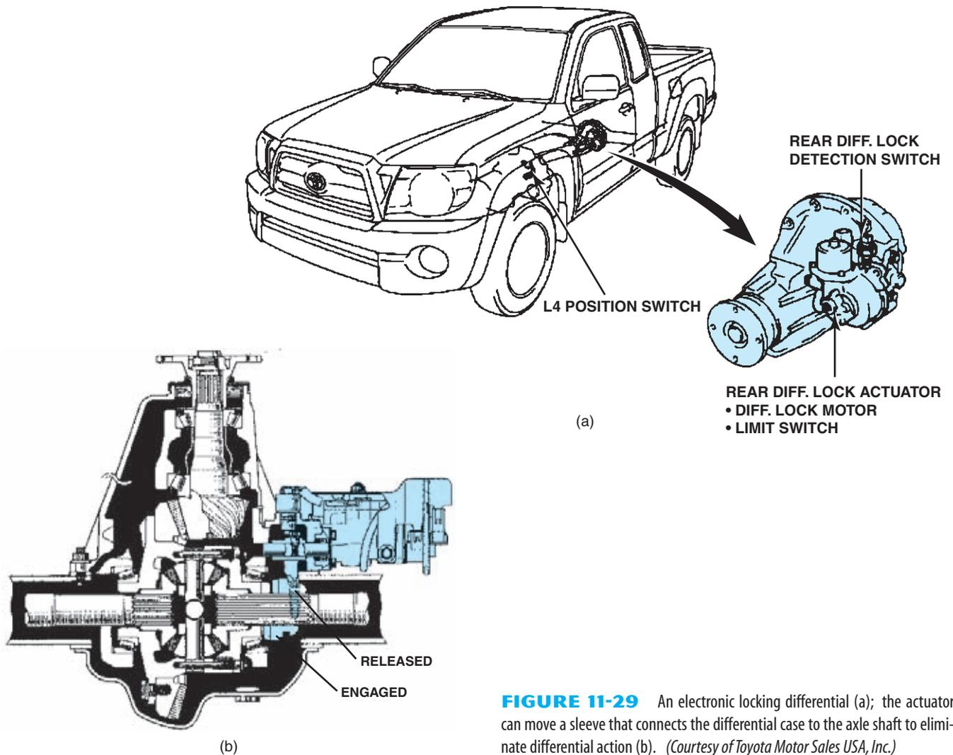
**FIGURE 11-29** An electronic locking differential (a); the actuator can move a sleeve that connects the differential case to the axle shaft to eliminate differential action (b). (Courtesy of Toyota Motor Sales USA, Inc.)
