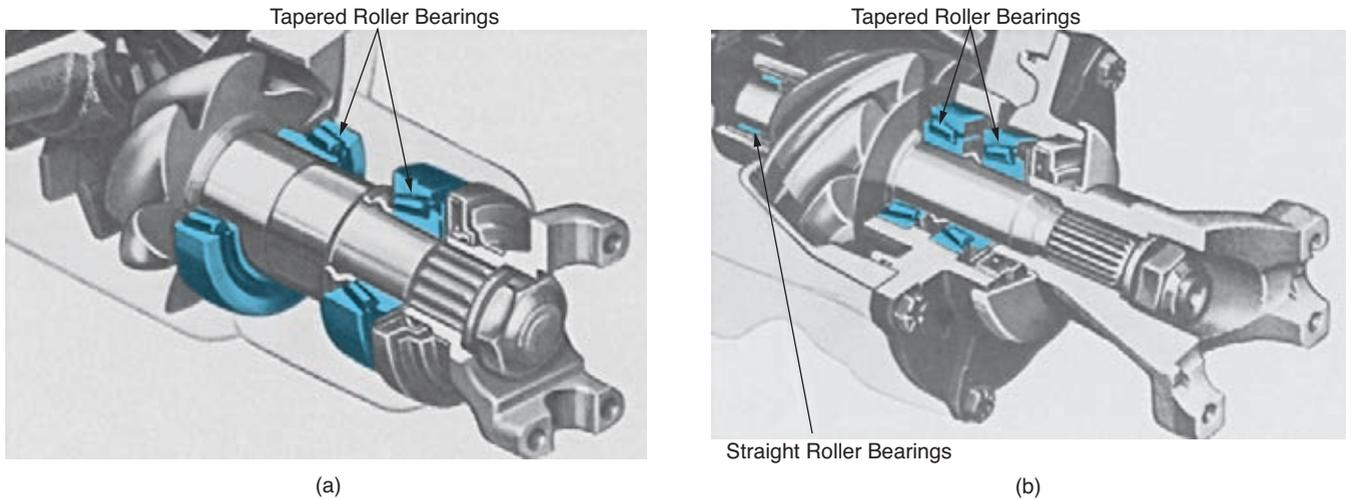
**FIGURE 11-10** An overhung-mounted pinion gear uses a pair of tapered roller bearings and locates them several inches apart (a). A straddle-mounted pinion gear uses a straight roller bearing in addition to the pair of tapered roller bearings (b). (Courtesy of Ford Motor Company)
