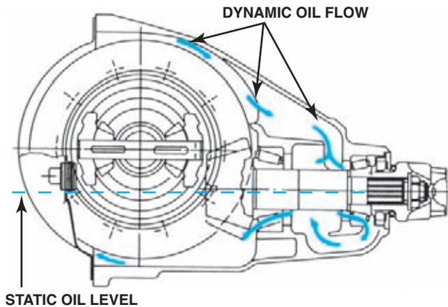
**FIGURE 11-35** In most axles the gear oil level is at the bottom of the filler opening. When the axle operates, the ring gear will produce a dynamic oil flow to lubricate all the parts. (Courtesy of DaimlerChrysler Corporation)
