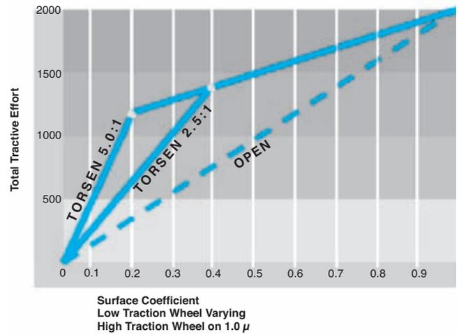
**FIGURE 11-18** This curve shows the torque bias ratio, the increased amount of torque that can be sent to the tire with good traction. (Courtesy of Zexel Torsen, Inc.)
