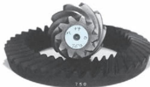
**FIGURE 11-4** Hypoid ring and pinion gear set; the 750 etched on each gear indicates a matched gear set. This pinion gear will operate properly only with this ring gear. (Courtesy of Dana Corporation)
