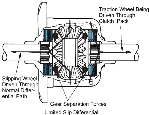
**FIGURE 11-20** A limited slip differential transfers most of the torque through the pinion shaft and gears like a conventional differential. Some torque is also transferred through the clutch pack going from the case through the clutch to the side gear (right).
