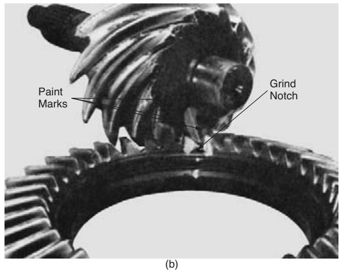
**FIGURE 11-7** In this nonhunting gear set (4:1 ratio), one pinion gear tooth will contact the same four teeth on the ring every revolution (a). These gear sets have timing marks so that the gear teeth can be located correctly (b). (b is courtesy of Ford Motor Company)
