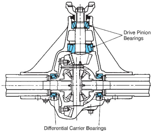
**FIGURE 11-8** A pair of tapered roller bearings called carrier bearings are used to locate the drive pinion gear and the differential case and ring gear. Another pair of bearings locates the drive pinion gear. (Courtesy of Dana Corporation)
