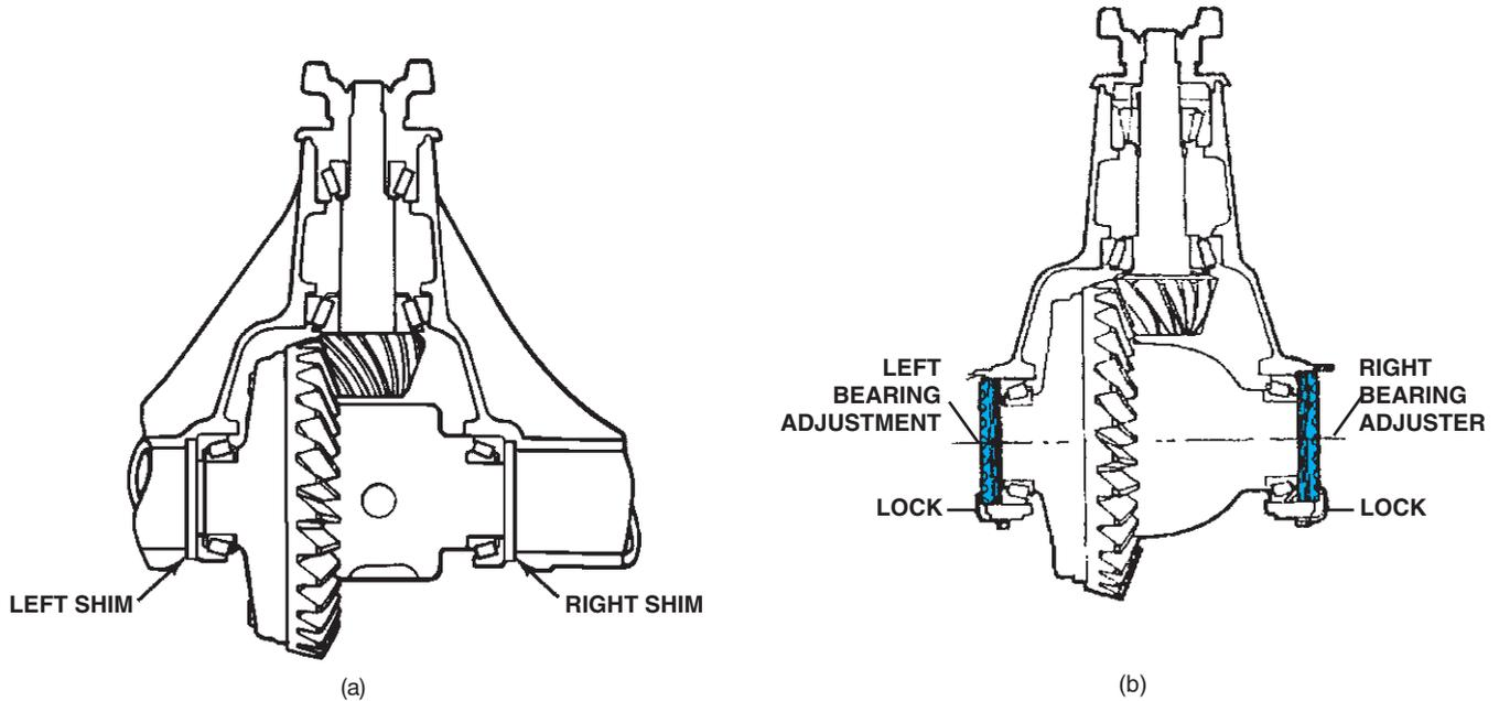
**FIGURE 11-14** Reducing the size of the left shim and increasing the size of the right shim will move the ring gear away from the pinion and increase backlash (a). Turning the left adjuster outward and the right adjuster inward will do the same thing (b). (Courtesy of Ford Motor Company)
