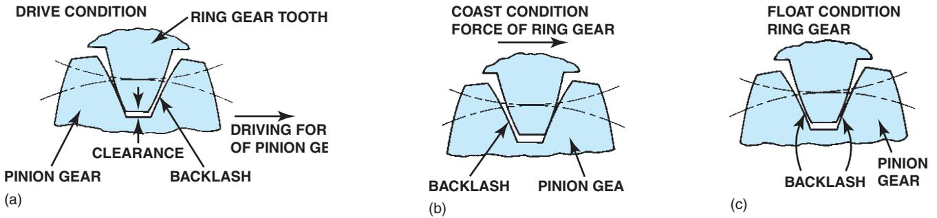
**FIGURE 11-6** During a drive condition, the pinion gear is driving the ring gear, and there is backlash at the coast side of the ring gear tooth (a). During a coast condition, this action is reversed (b); and during a float condition, lash is split between both sides of the tooth (c).
