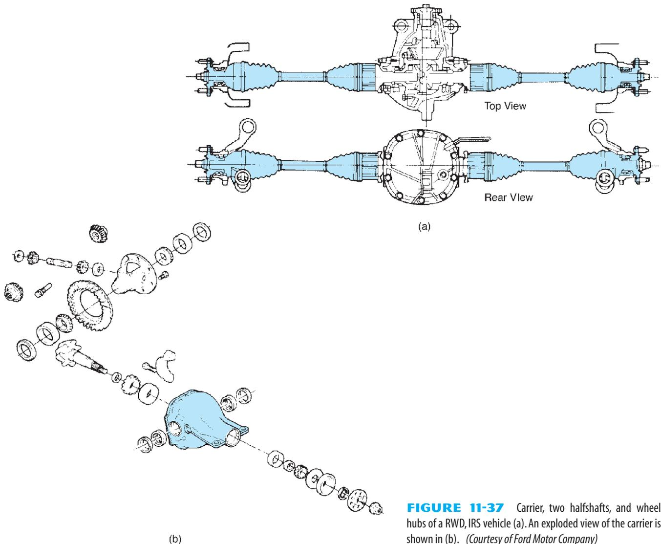
**FIGURE 11-37** Carrier, two halfshafts, and wheel hubs of a RWD, IRS vehicle (a). An exploded view of the carrier is shown in (b). (Courtesy of Ford Motor Company)
