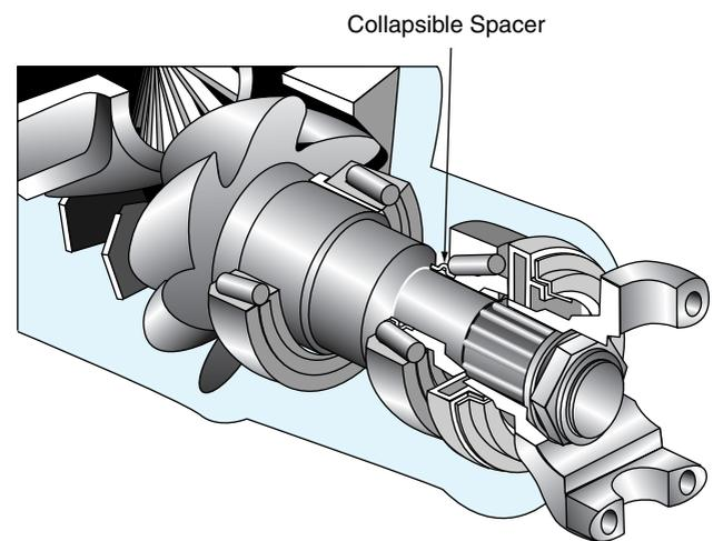
**FIGURE 11-12** The collapsible spacer is compressed during the drive pinion bearing preload adjustment to get the correct amount of preload on the bearings. Some axles use solid spacers and shims for this adjustment. (Courtesy of Ford Motor Company)
