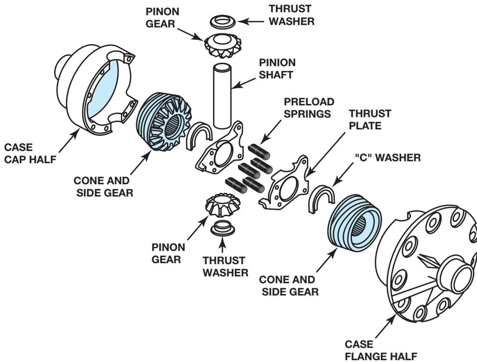
**FIGURE 11-23** Exploded view of a limited slip differential using cone-type clutches.
