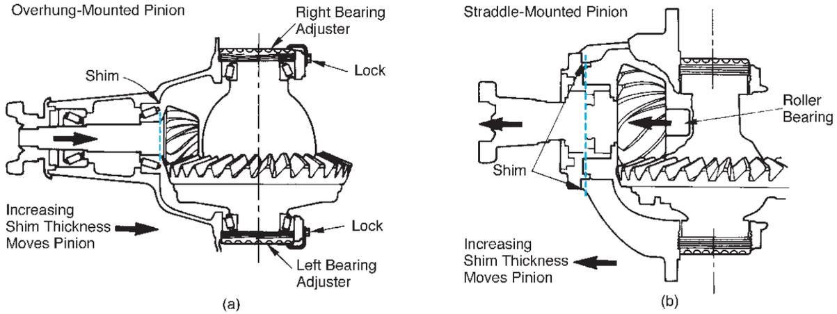
**FIGURE 11-13** The shim used to adjust pinion depth is located between the pinion gear and rear bearing in most axles (a) and between the pinion retainer and carrier in some axles (b). (Courtesy of Ford Motor Company)
