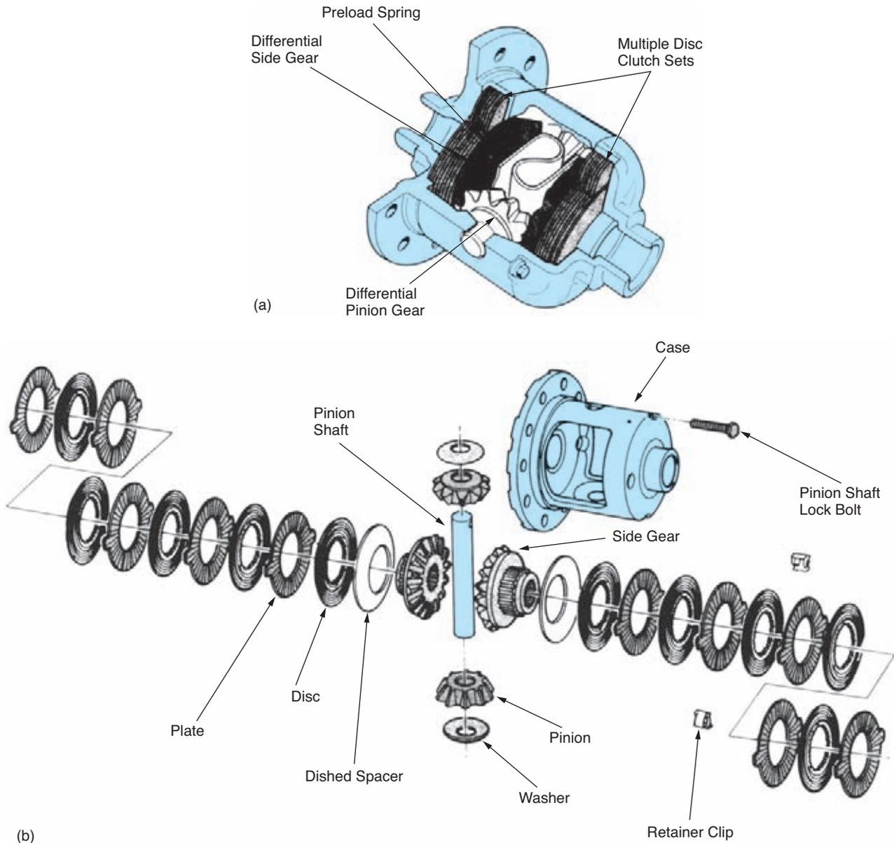
**FIGURE 11-21** Cutaway (a) and exploded (b) views of a limited slip differential using clutch plates. (Courtesy of Ford Motor Company)
