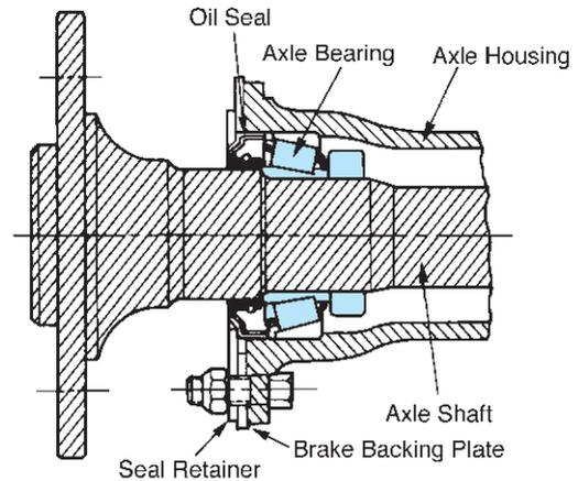
**FIGURE 11-33** This bearing-retained axle is held in the axle housing by the seal retainer.
