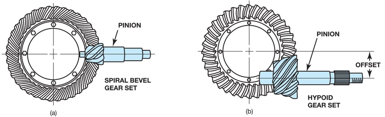
**FIGURE 11-2** Spiral bevel (a) and hypoid (b) gear sets; hypoid gears are used in most drive axles. Offset is a design factor.
