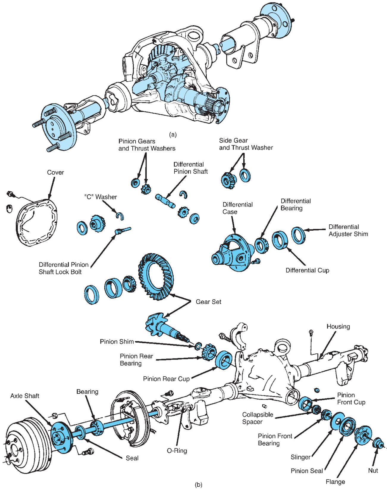
**FIGURE 11-1** Cutaway (a) and exploded (b) views of a rear axle assembly. (Courtesy of Ford Motor Company)
