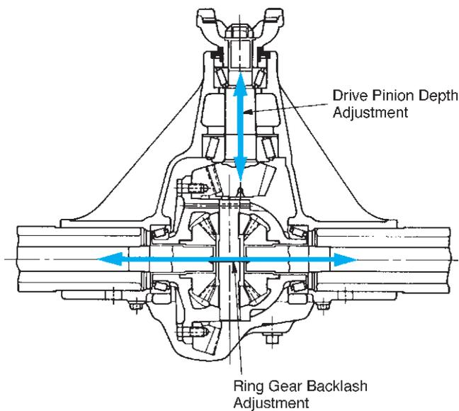
**FIGURE 11-11** When a hypoid gear set is assembled, pinion depth and ring gear backlash, as well as bearing preload on each bearing set, must be adjusted.
