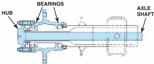
**FIGURE 11-32** Cutaway view of a full-floating axle and hub. Note the bearings supporting the hub and the axle attachment. (Courtesy of Daimler-Chrysler Corporation)
