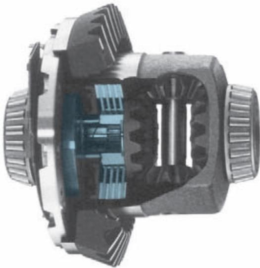
**FIGURE 11-27** A Vari-Lock (Hydra-Lok) differential includes a gerotor oil pump that is driven when the axles operate at different speeds. If there is too much speed differential, the fluid pressure can apply the internal clutch to reduce wheel spin. (Courtesy of DaimlerChrysler Corporation)
