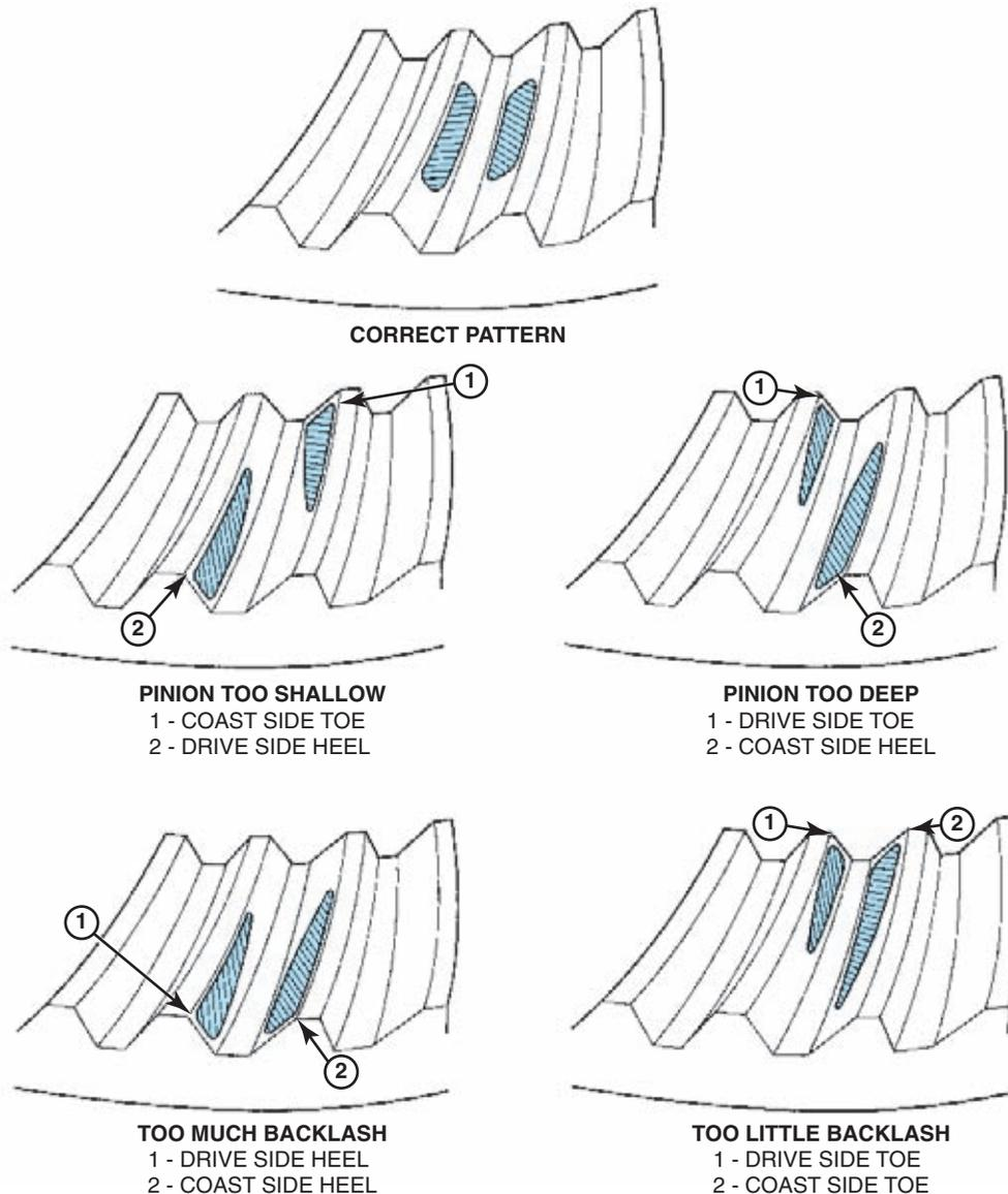
**FIGURE 11-15** Good ring gear contact pattern (top) and patterns that require further adjustment. The location of the gear contact shows the technician what adjustment is needed. (Courtesy of DaimlerChrysler Corporation)
