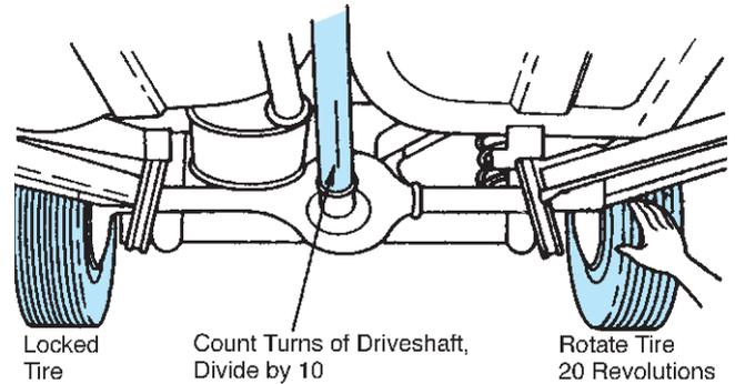
**FIGURE 11-39** The quickest and most accurate method of determining a rear axle ratio is shown here. If the driveshaft rotates  $37 \frac{1}{3}$  turns while the free tire rotates 20 turns, the ratio is 3.73:1.
