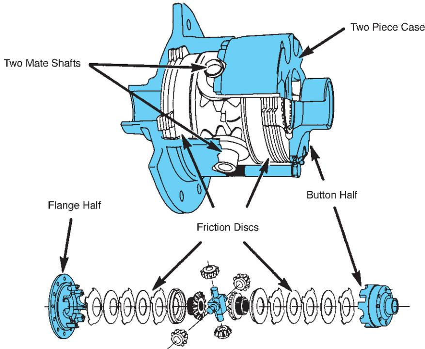
**FIGURE 11-25** This limited slip differential uses the action of the pinion mate shafts and ramps in the differential case to apply pressure on the clutch pack and send torque to the wheel with traction. (Courtesy of DaimlerChrysler Corporation)
