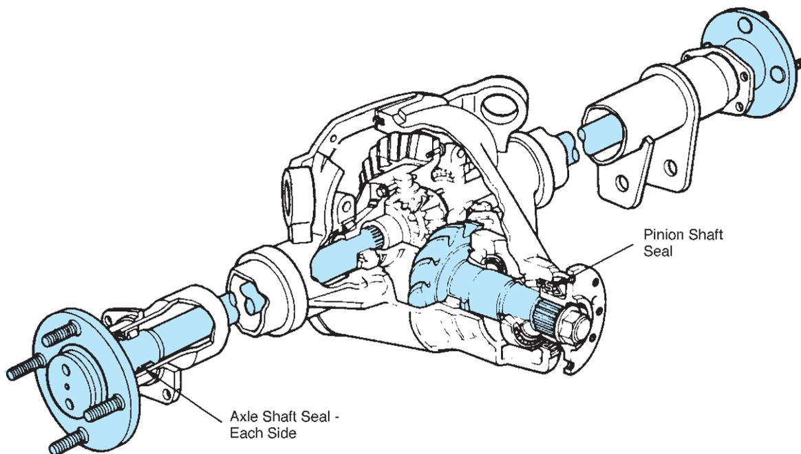
**FIGURE 11-36** The gear oil is kept in the housing by seals at each axle shaft, the drive pinion shaft, and gaskets or sealant at each cover. (Courtesy of Ford Motor Company)
