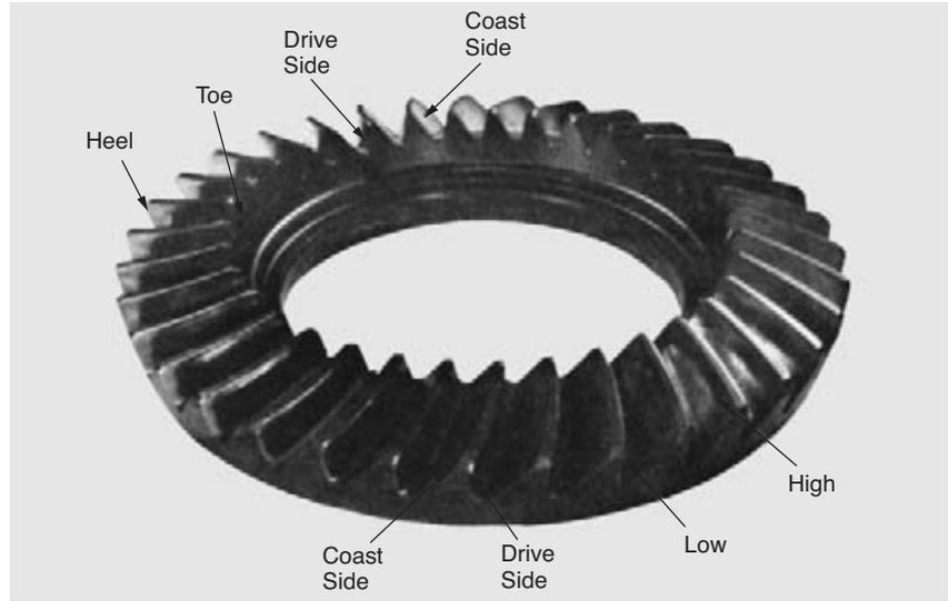
**FIGURE 11-5** Ring gear showing the terms used to identify certain sections of the gear. (Courtesy of Ford Motor Company)
