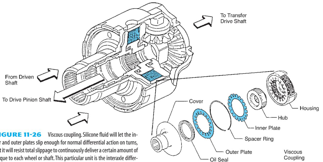
**FIGURE 11-26** Viscous coupling. Silicone fluid will let the inner and outer plates slip enough for normal differential action on turns, but it will resist total slippage to continuously deliver a certain amount of torque to each wheel or shaft. This particular unit is the interaxle differential for an AWD vehicle. (Courtesy of Subaru of America, Inc.)
