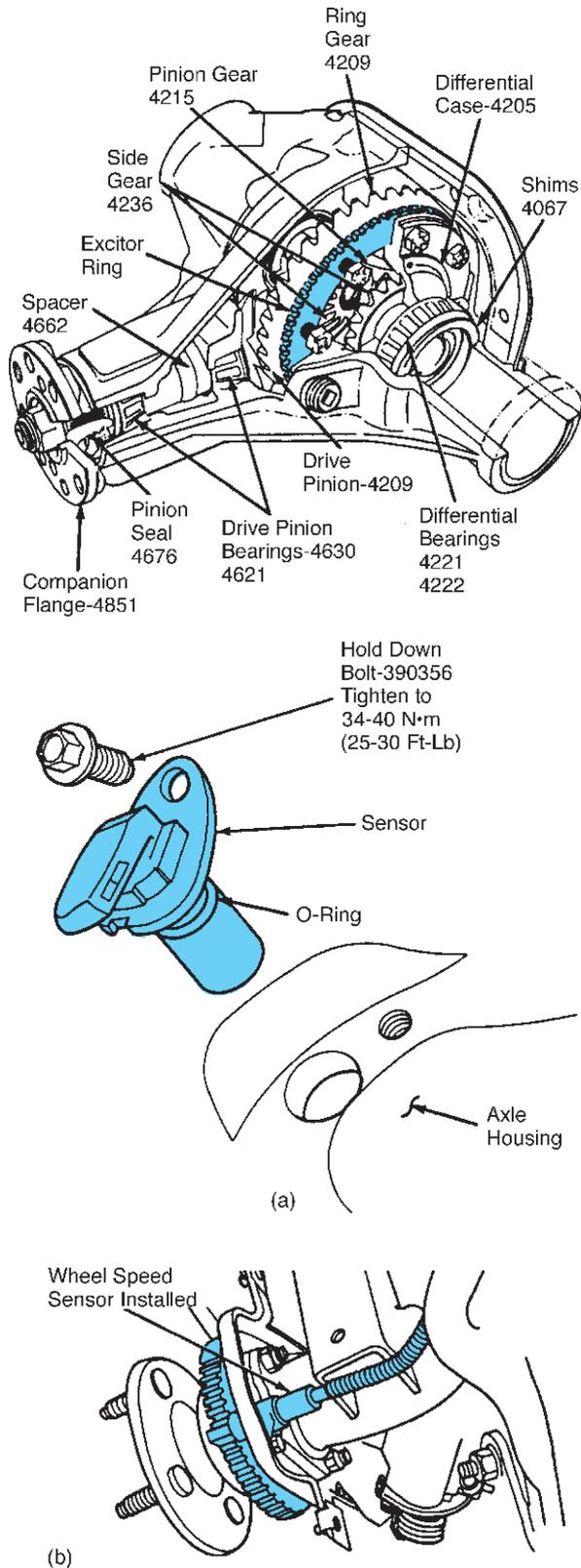
**FIGURE 11-16** Vehicles with ABS will have a single rear-wheel speed sensor at the ring gear (a) or a speed sensor at each axle shaft (b). Some will use a sensor similar to (a) at the drive pinion shaft. (Courtesy of Ford Motor Company)
