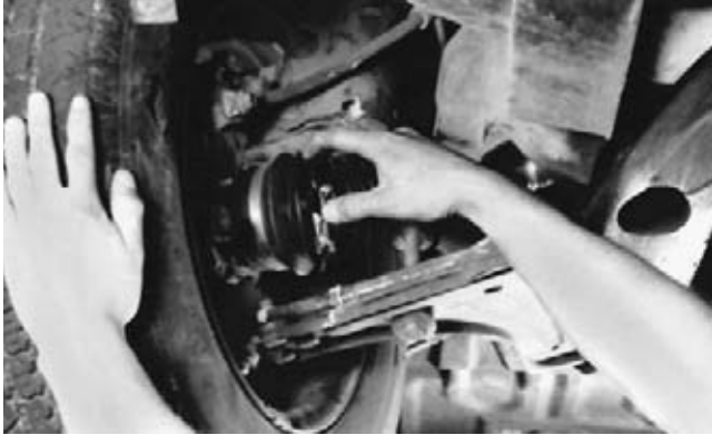
FIGURE 10-6 When checking a CV joint boot, run your finger around the boot in each of the pleats as you inspect for tears or cuts; the wheel can be turned outward on the outboard joint to get a better view of the boot. (Courtesy of Moog Automotive)
