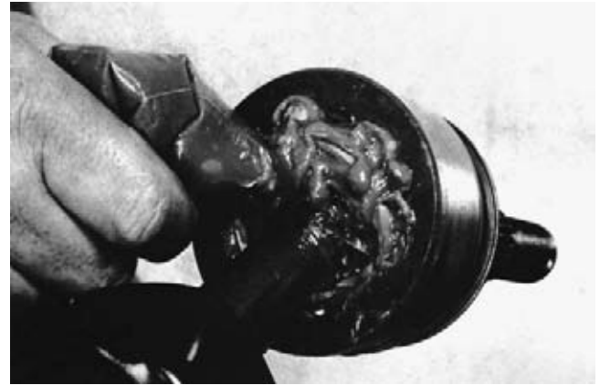
FIGURE 10-49 After the joint has been cleaned thoroughly, it is repacked with grease, working the grease into all parts of the joint. (Courtesy of NEAPCO)
