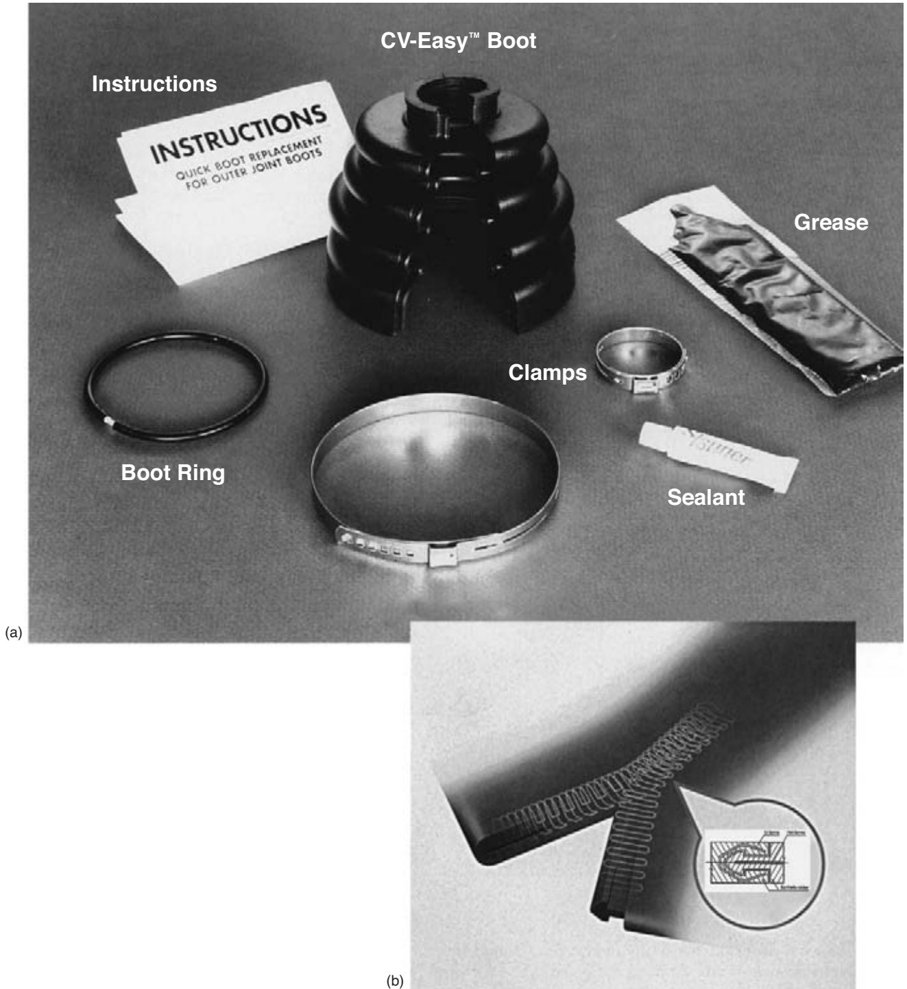
FIGURE 10-41 A Quick Replacement outer CV boot kit (a). This boot has a seam that is held together by two unique springs and the shape of the rubber (b). (Courtesy of Sisuner International)
