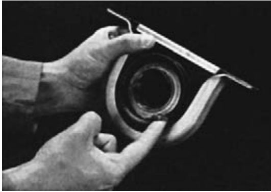
FIGURE 10-70 Before reassembling a center support bearing, waterproof grease should be packed into the cavity around the bearing to shield it from water and other contaminants. (Courtesy of Dana Corporation)
