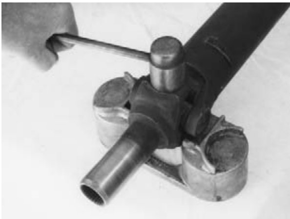
FIGURE 10-61 In the hammer and anvil method, a U-joint is disassembled by driving the cupped driving tool against the side of one yoke while the anvil supports the other yoke, along with the cross.
