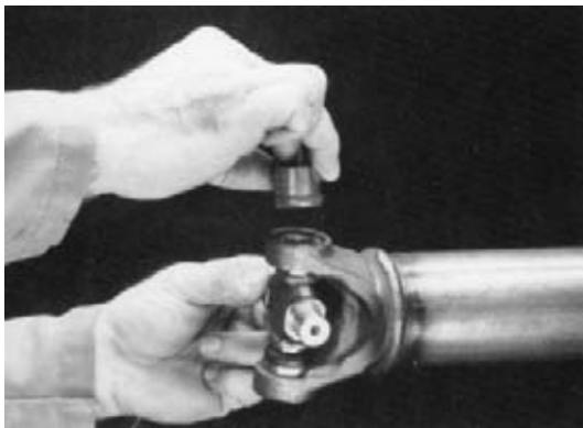
FIGURE 10-64 A Cardan U-joint is assembled by placing the cross in a yoke (a); starting a bearing cup onto a cross journal (b); pressing that bearing cup into position using a U-joint press or press with adapters (c). (a, b, are courtesy of Dana Corporation; c is courtesy of Ford Motor Company)
