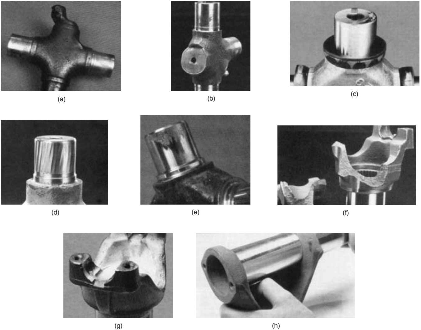
FIGURE 10-62 Commonly encountered U-joint faults are a cross with a burned journal (a); broken cross (b); a cross journal with end galling (c), brinelling (d), or spalling (e); a fractured yoke (f); a yoke with a broken tang (g); and a bent yoke (h). A special checking gauge is being used to check the yoke (h) for distortion. (Courtesy of Dana Corporation)
