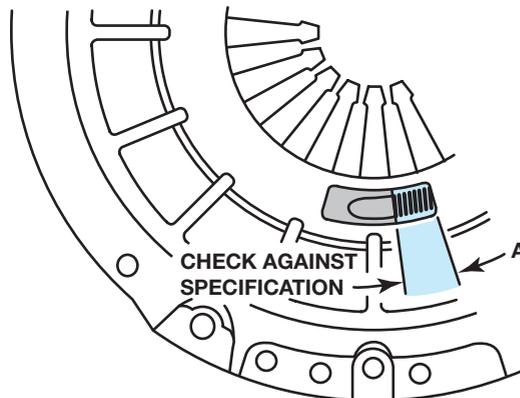
**FIGURE 5-36** When installing a pressure plate with a self-adjusting fulcrum ring, check dimension A. If the distance exceeds the specification, follow the proper procedure to adjust it.
