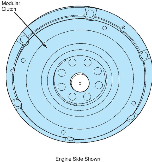
**FIGURE 5-31** When replacing a modular clutch, the new modular assembly has a new flywheel, clutch disc, and pressure plate is bolted onto the flexplate. (Courtesy of DaimlerChrysler Corporation)
