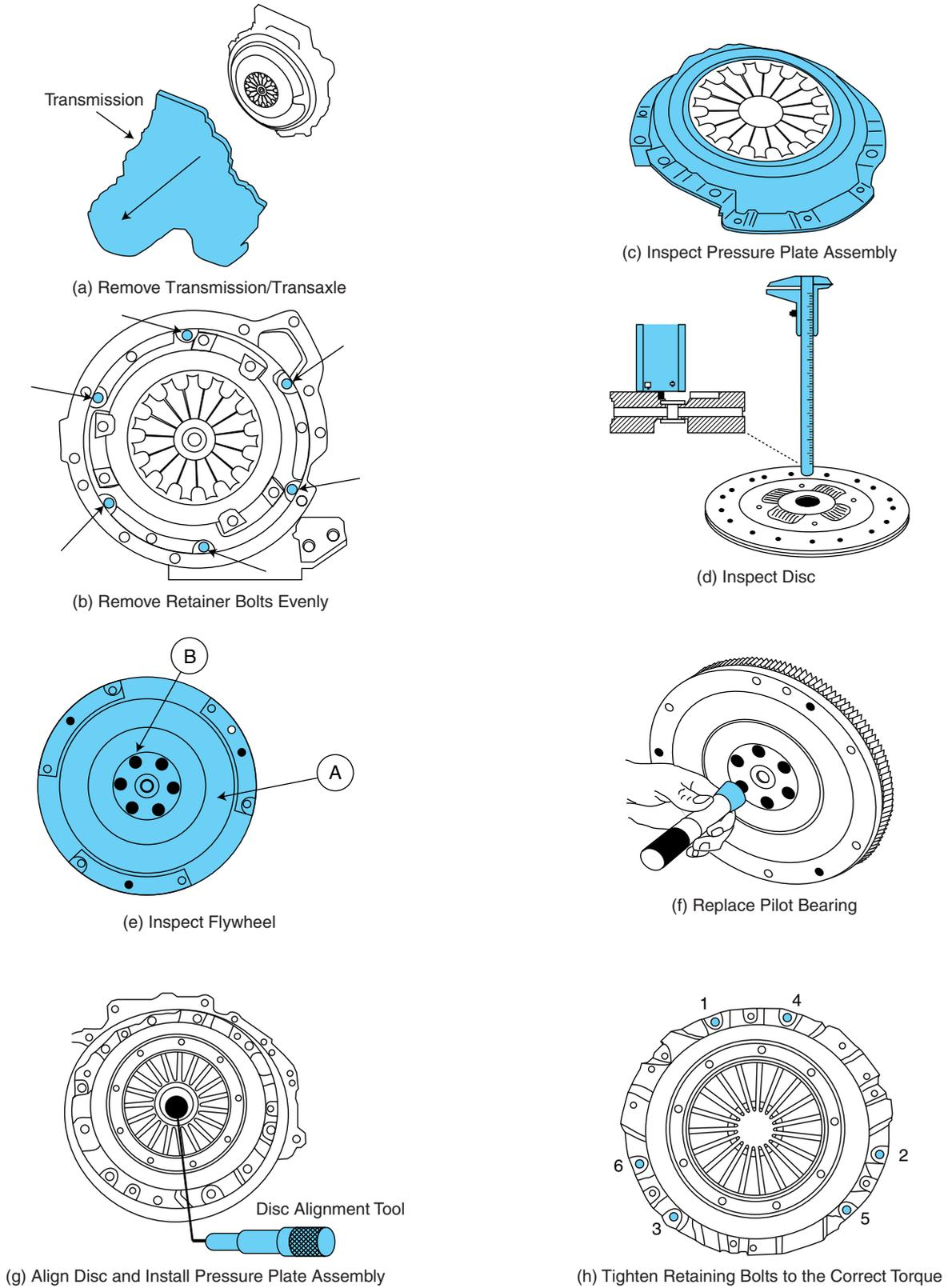
**FIGURE 5-11** The sequence for a clutch job is to remove the transmission/transaxle (a); remove the clutch components (b); inspect the pressure plate assembly (c), disc (d), flywheel (e); replace the pilot bearing (f); install and align the disc and pressure plate assembly (g); and tighten the bolts to the correct torque and in the correct sequence (h).
