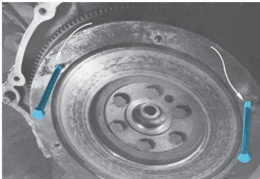
**FIGURE 5-21** Two long bolts (arrows) have been threaded into the flywheel to serve as handles for carrying and positioning.
