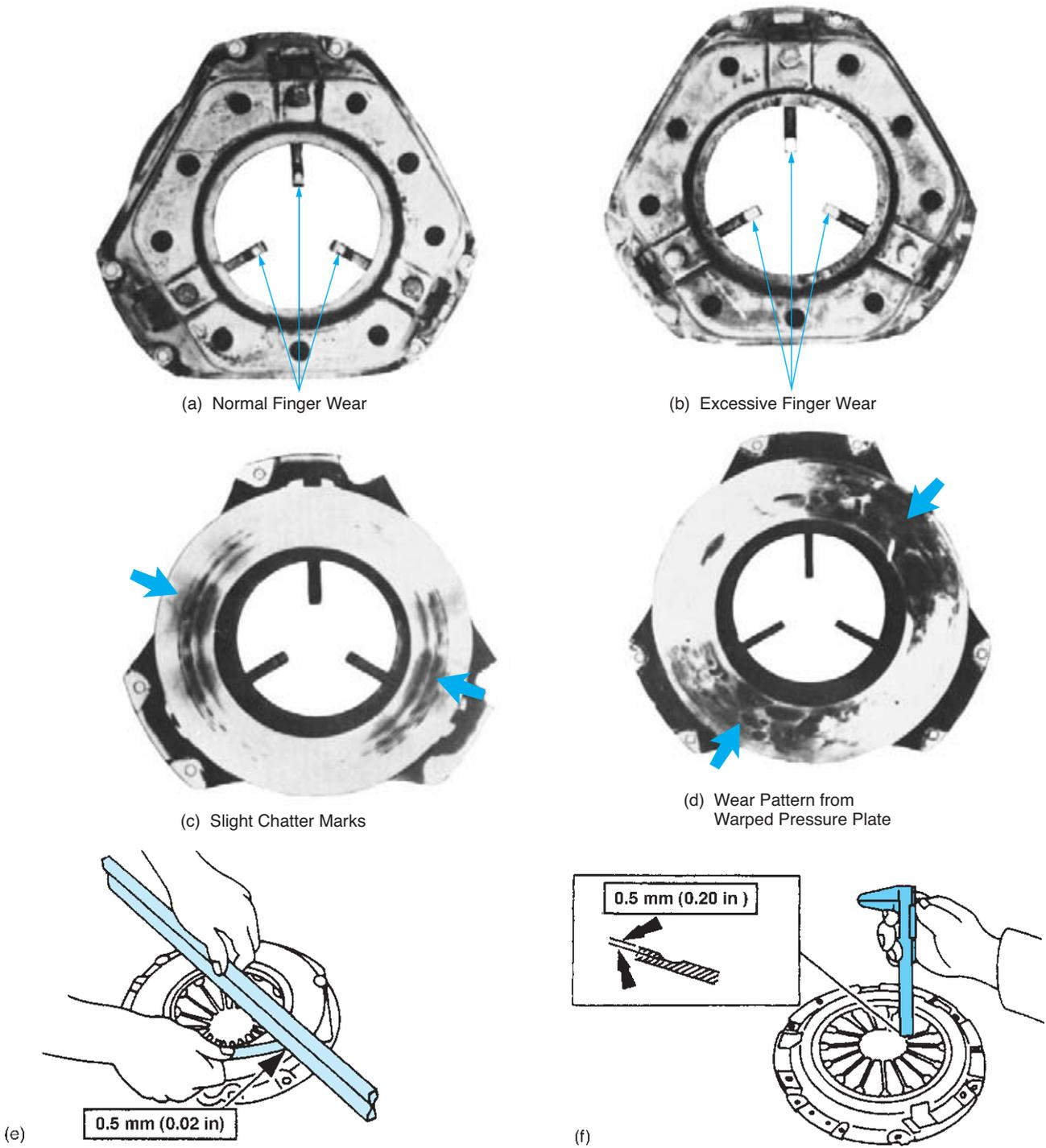
**FIGURE 5-22** Commonly encountered pressure plate faults are excessive finger wear (b and f), chatter marks (c), and excessive warpage (d and f). (Courtesy of Ford Motor Company)
