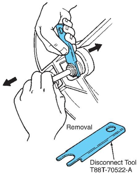
**FIGURE 5-43** Most older cars used threaded line connections to the clutch master and slave cylinders. This vehicle uses a snap-in connector that requires a special tool for disassembly. (Courtesy of Ford Motor Company)
