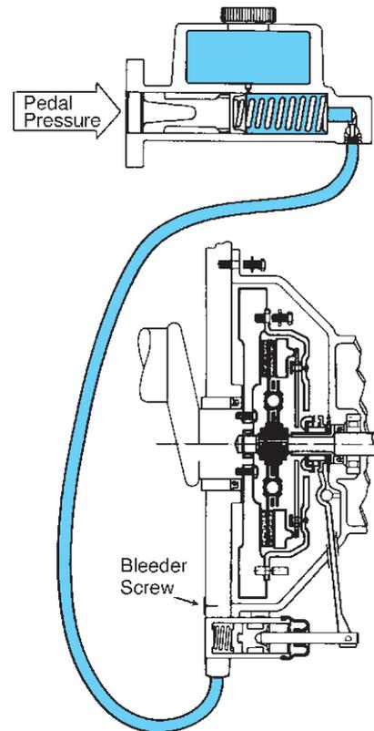
**FIGURE 5-44** On many clutch systems, loosening the bleeder screw at the slave cylinder allows gravity to push the air out of the slave cylinder. Sometimes, it is necessary to have an assistant apply pressure at the pedal as the bleeder screw is opened. (Courtesy of LUK Clutches)
