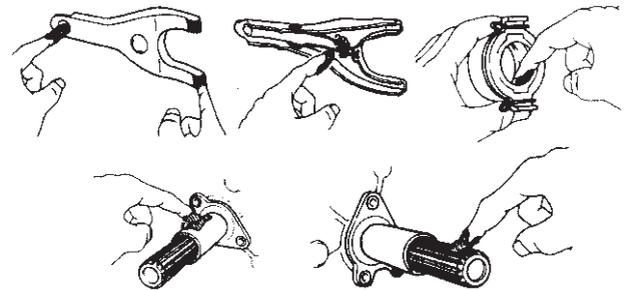
**FIGURE 5-40** The contact points of the fork and release bearing along with the transmission quill and clutch splines should be lubricated with a very thin film of grease. (Courtesy of Toyota Motor Sales USA, Inc.)
