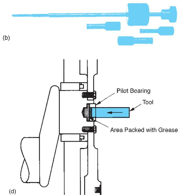
**FIGURE 5-16** A pilot bearing is removed by catching it with an expanding puller attached to a slide hammer (a) a puller set is shown (b) using a special-purpose puller (c) or filling it with grease and driving a round tool into the bearing (d). (b is courtesy of LUK Clutches; c is Courtesy of Toyota Motor Sales USA, Inc.)
