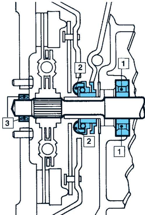
**FIGURE 5-10** Any of these three bearings can cause noise. A faulty transmission input shaft bearing (1) will cause noise while the clutch is engaged; a faulty release bearing (2) will cause noise with the pedal depressed; and a faulty pilot bearing (3) will cause noise while the clutch is released. (Courtesy of LUK Clutches)
