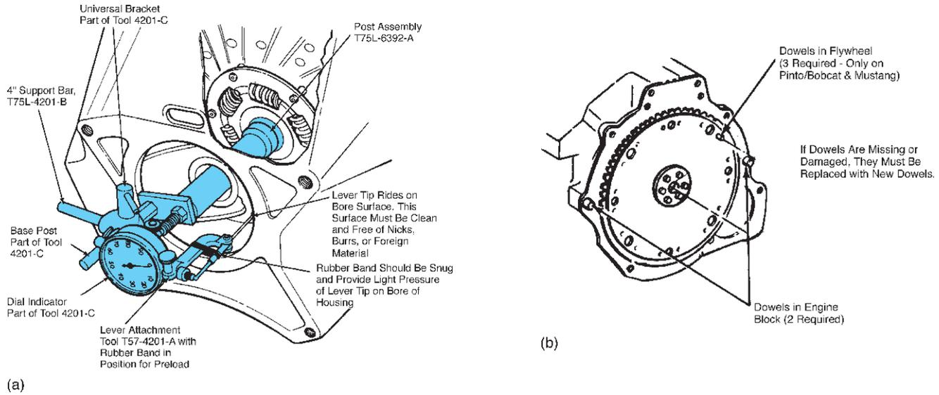
**FIGURE 5-27** (a) This dial indicator has a lever or wiggle bar added to check clutch housing bore runout. (b) Excessive runout can be caused by damaged or missing dowels; if the dowels are good, runout can be corrected by installing eccentric dowels. (Courtesy of Ford Motor Company)
