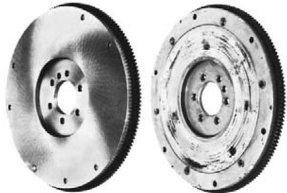
**FIGURE 5-17** A new (left) and typical worn flywheel (right). This worn flywheel should be resurfaced. (Courtesy of McLeod Industries, Inc.)
