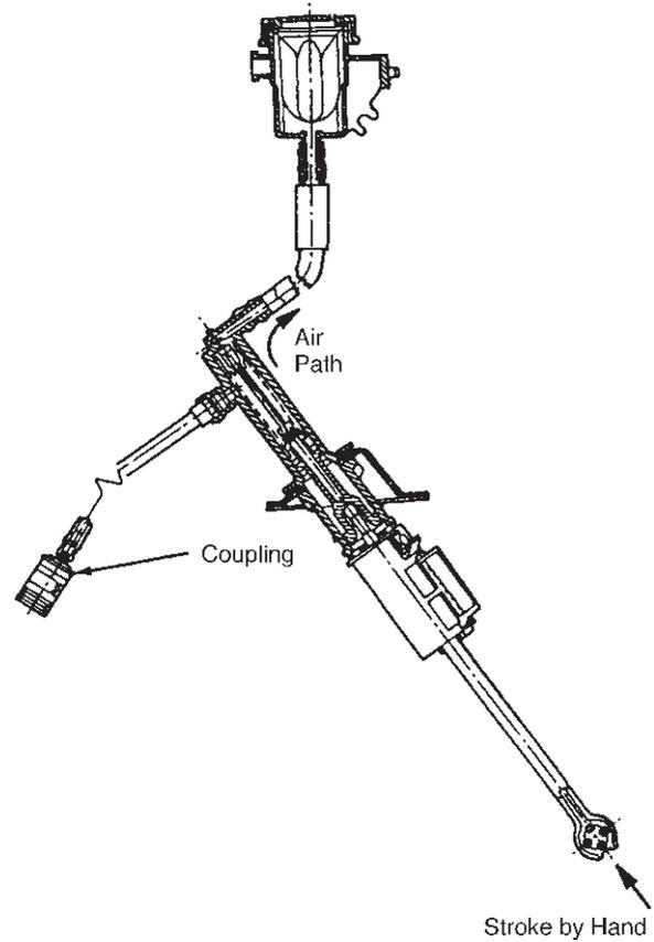
**FIGURE 5-46** This clutch master cylinder is mounted with the push-rod end above the inlet and outlet, which makes bleeding difficult. It can be bench bled by stroking the push rod by hand before mounting the master cylinder. (Courtesy of Ford Motor Company)
