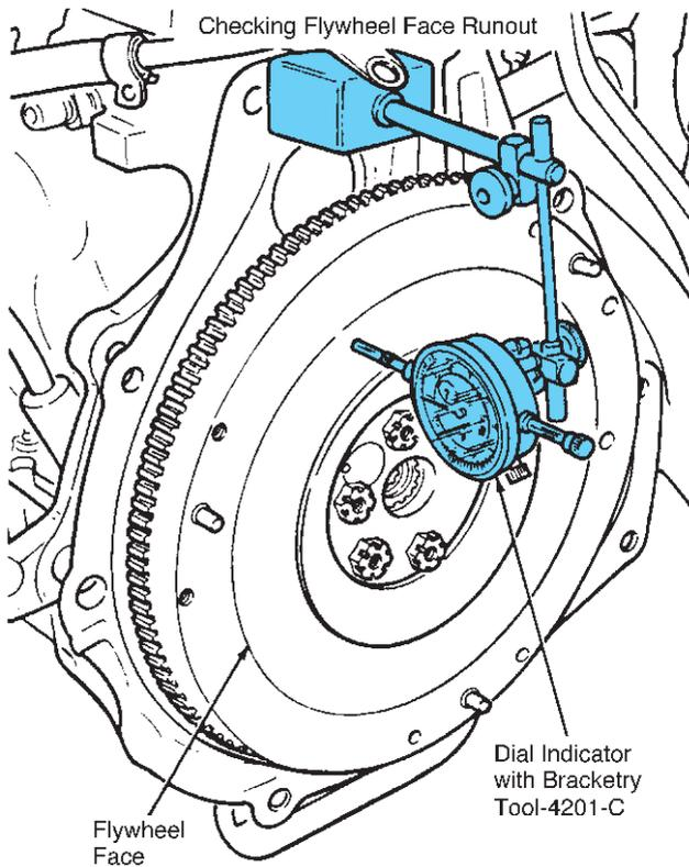
**FIGURE 5-20** This dial indicator is set up to measure flywheel face or axial runout. (Courtesy of Ford Motor Company)
