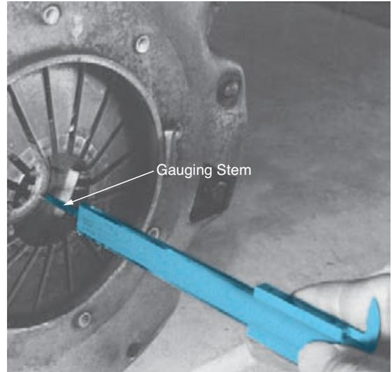
**FIGURE 5-39** The height of the release levers can be measured after the pressure plate assembly has been installed by measuring from the fingers to the hub of the disc. The readings should all be the same.
