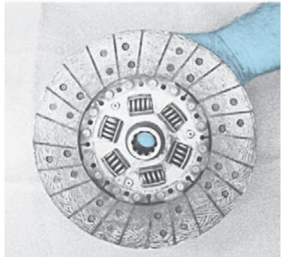
**FIGURE 5-30** A new disc should be held by the edges or center spline to prevent contamination of the facing, which can cause chatter.
