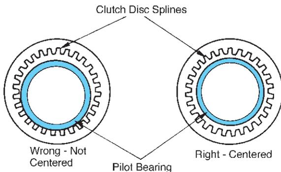
**FIGURE 5-38** After the bolts have been tightened to the correct torque, sight down the splines to make sure that they are centered to the pilot bearing.
