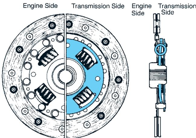
**FIGURE 5-33** Many replacement discs will have a marking indicating the flywheel or pressure plate side; the damper assembly is normally on the pressure plate or transmission side. (Courtesy of LUK Clutches)
