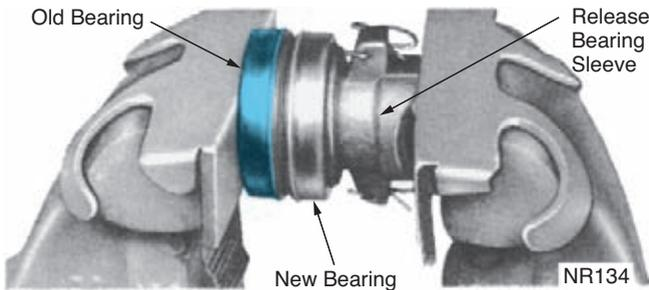
**FIGURE 5-28** Some release bearings are mounted on a sleeve, and the old bearing can be used to install the new one, as shown here. (Courtesy of DaimlerChrysler Corporation)
