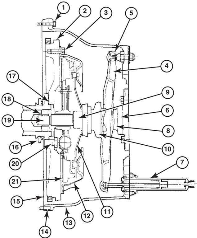
1. CHECK CLUTCH HOUSING BOLTS. TIGHTEN IF LOOSE. BE SURE HOUSING IS FULLY SEATED ON ENGINE BLOCK.
