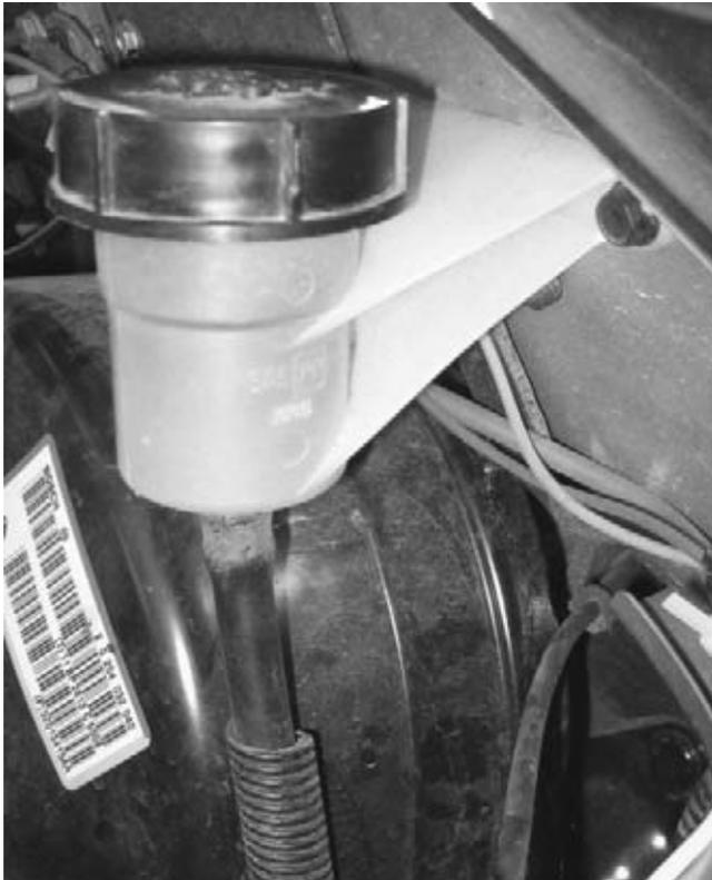
**FIGURE 5-4** The hydraulic clutch fluid is checked looking at the fluid level through the plastic reservoir.
