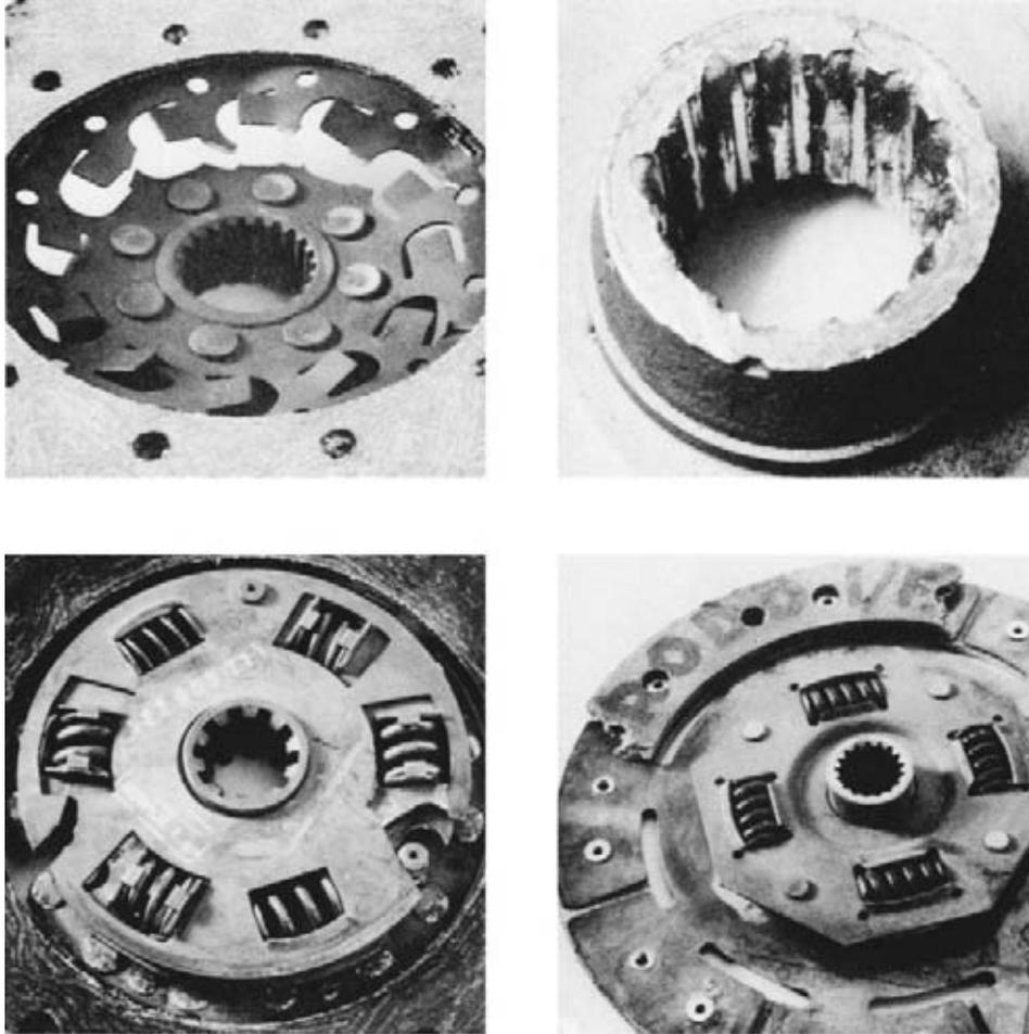
**FIGURE 5-23** Clutch disc failure comes in many forms; a good technician will determine and correct the cause of abnormal failures so they won't occur again. (Courtesy of LUK Clutches)
