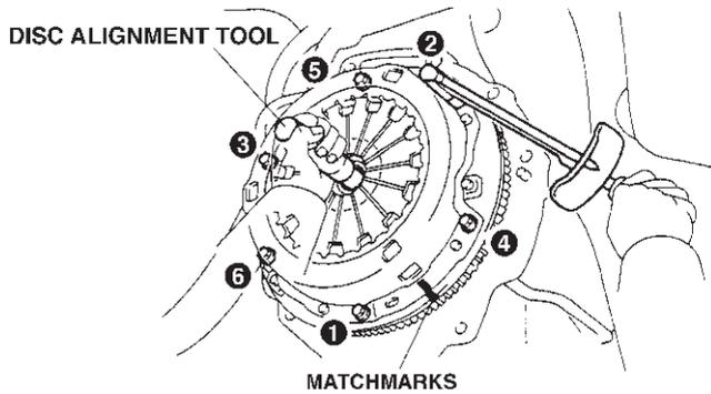
**FIGURE 5-37** With the disc held centered, the pressure plate bolts should be tightened two turns at a time in a pattern like this. (Courtesy of Toyota Motor Sales USA, Inc.)
