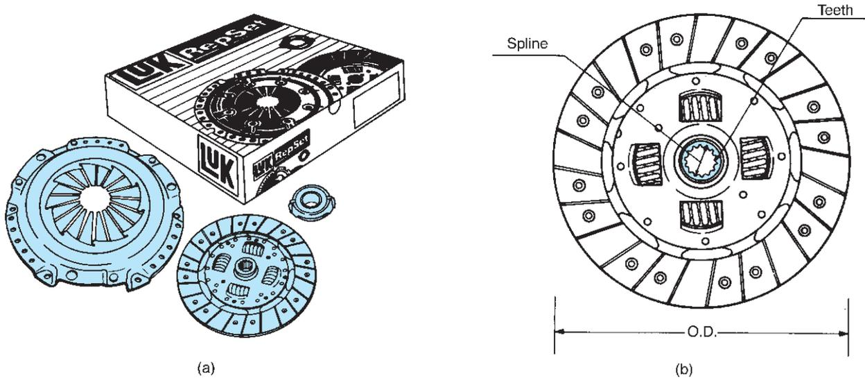
**FIGURE 5-13** Some suppliers package a replacement disc and pressure plate assembly along with the release bearing in one package (a). Sometimes the pilot bearing is also included. The critical dimensions for the replacement disc are shown in (b). (Courtesy of LUK Clutches)
