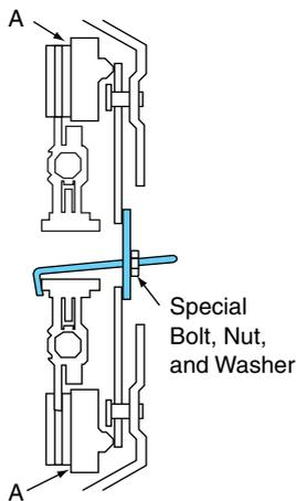
**FIGURE 5-35** A simple, shop-made tool can be used to hold the disc centered against the pressure plate as the pressure plate is installed. The gaps at the edge of the disc and pressure plate (A) should be equal.
