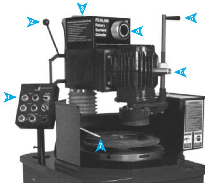
**FIGURE 5-18** A flywheel grinder rotates the flywheel as a spinning stone is lowered onto the surface. Various styles of flywheels, including stepped ones (inset), can be resurfaced using this machine. (Courtesy of Van Norman Equipment Co., Inc.)
