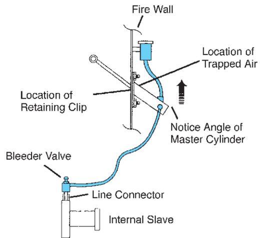
**FIGURE 5-47** Another way of bleeding a difficult clutch master cylinder is to have an assistant depress the clutch pedal, build a pressure in the system using a fluid injector at the bleeder valve, and slowly release the pedal. The pressure surge will force the trapped air upward. This operation should be repeated several times. (Courtesy of Phoenix Systems)
