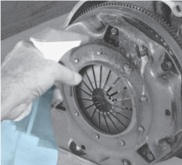
**FIGURE 5-15** Before disassembly, it is a good practice to wash the pressure plate assembly and flywheel with a mixture of soap and water. This prevents airborne asbestos fibers and precleans the clutch cover.
