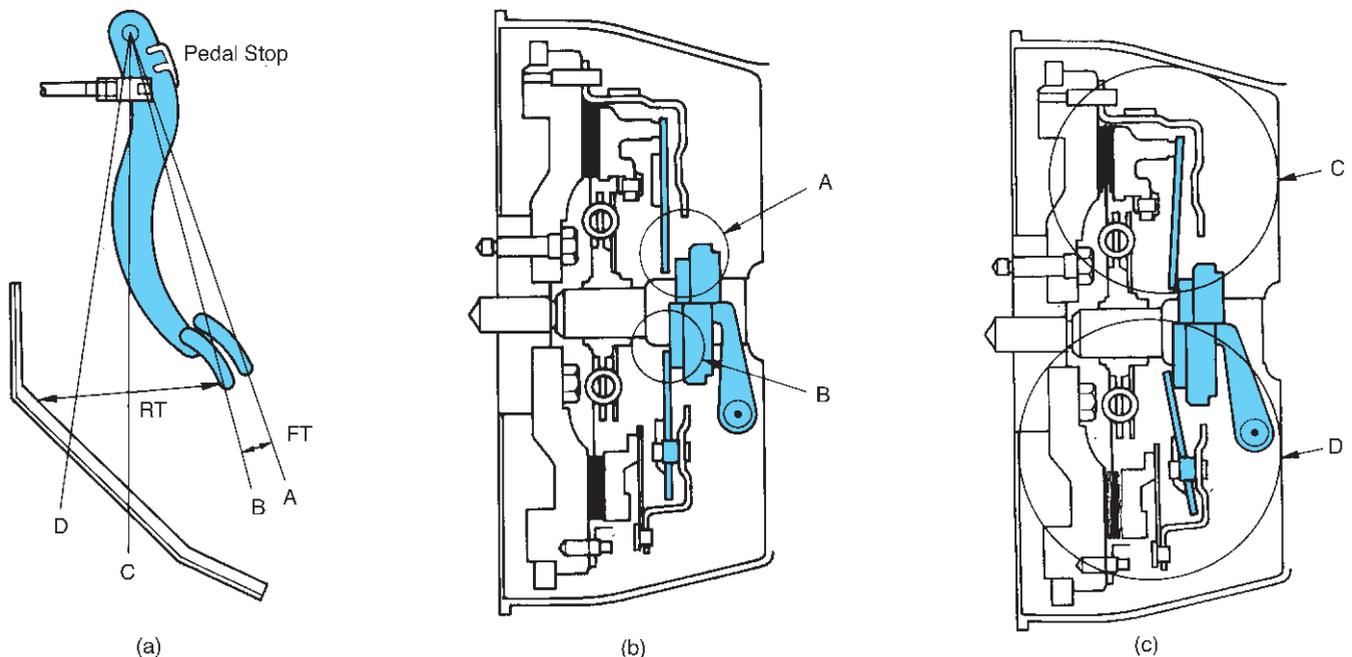
**FIGURE 5-1** As the clutch pedal is depressed (a), it will move through its free travel as the release bearing moves to contact the release levers (b). The pressure plate then moves away from the flywheel, allowing the marcel of the disc to expand (c). When the pedal reaches the floor, there should be an air gap at both sides of the disc (d).
