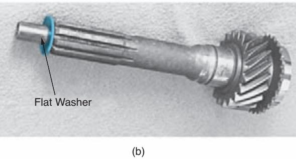
**FIGURE 5-32** (a) A new pilot bearing should be installed using a driver. (b) If a clutch shaft is used as a driver, a flat washer should be placed on the shaft to prevent damaging the bearing. (a is courtesy of Ford Motor Company)
