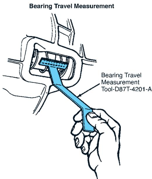
**FIGURE 5-9** If the hydraulic clutch problem is failure to release, check for proper bearing travel. Insufficient bearing travel indicates a faulty hydraulic system. (Courtesy of Ford Motor Company)
