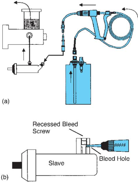
**FIGURE 5-45** A clutch hydraulic system can be reverse bled by pumping fluid through the bleeder valve or hole and up to the reservoir; the air will leave the fluid at the reservoir. (Courtesy of Phoenix Systems)
