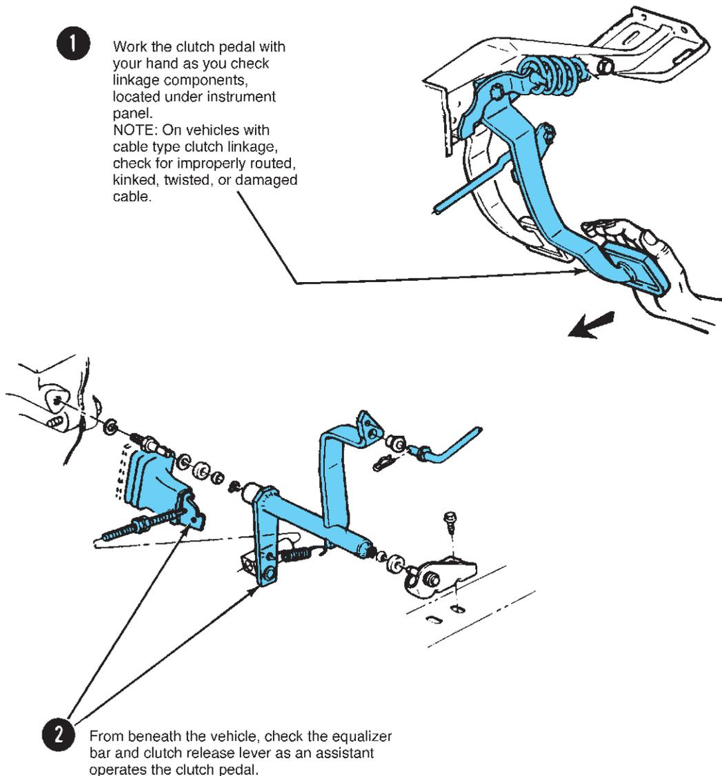
**FIGURE 5-7** Check for noises by moving the pedal by hand as you check the various parts of the linkage. If necessary, the linkage can be disconnected to isolate different portions. (Courtesy of Ford Motor Company)
