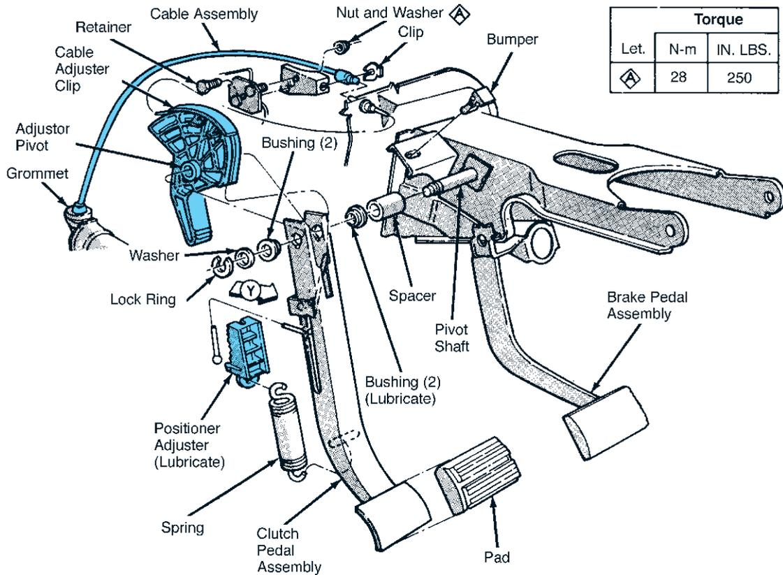
**FIGURE 5-8** With a self-adjusting clutch, check the cable, cable adjuster clip (cam), and positioner adjuster for proper operation. (Courtesy of DaimlerChrysler Corporation)
