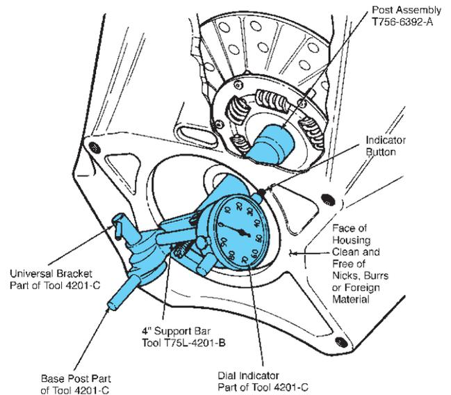
**FIGURE 5-26** A dial indicator is mounted to the clutch disc or the pressure plate assembly and the crankshaft is rotated to check for runout at the face of the clutch housing. It can also be mounted to the crankshaft to check for runout of the clutch housing surface. (Courtesy of Ford Motor Company)
