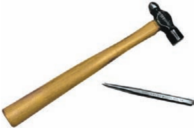
Figure E-13 Layout hammer and layout prick punch.
