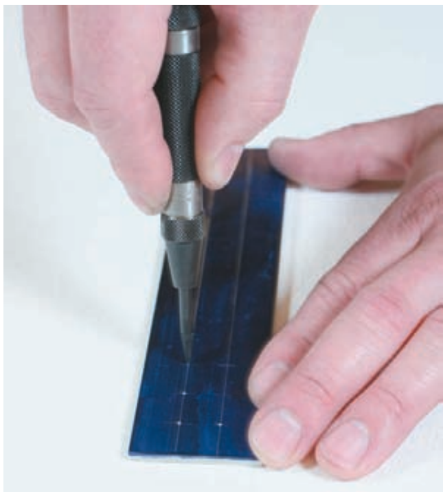
Figure E-17 Using the automatic center punch in layout.
