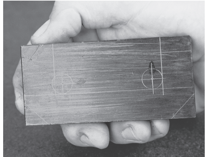
Figure E-79 Completed layout of the clamp frame.
