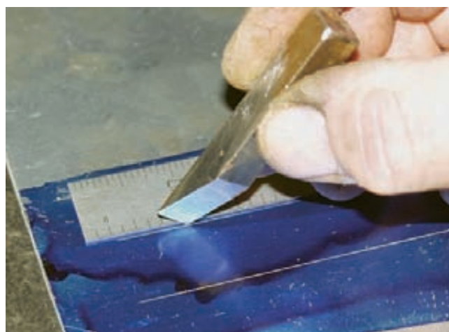
Figure E-7 Rule scribe made from a high-speed tool bit.
