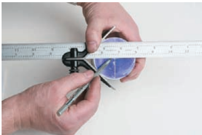
Figure E-20 Using the centerhead to lay out a centerline on round stock.
