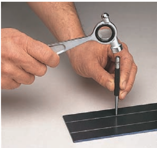
Figure E-15 Using a toolmaker's hammer and layout punch (Courtesy of The L.S. Starrett Co.).
