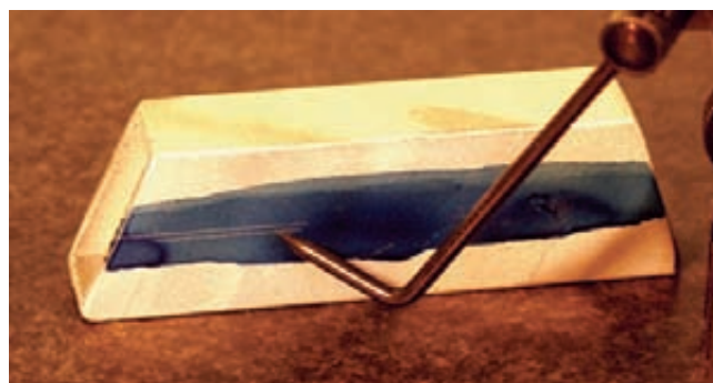
Figure E-23 Finding the centerline of the workpiece using the surface gage.
