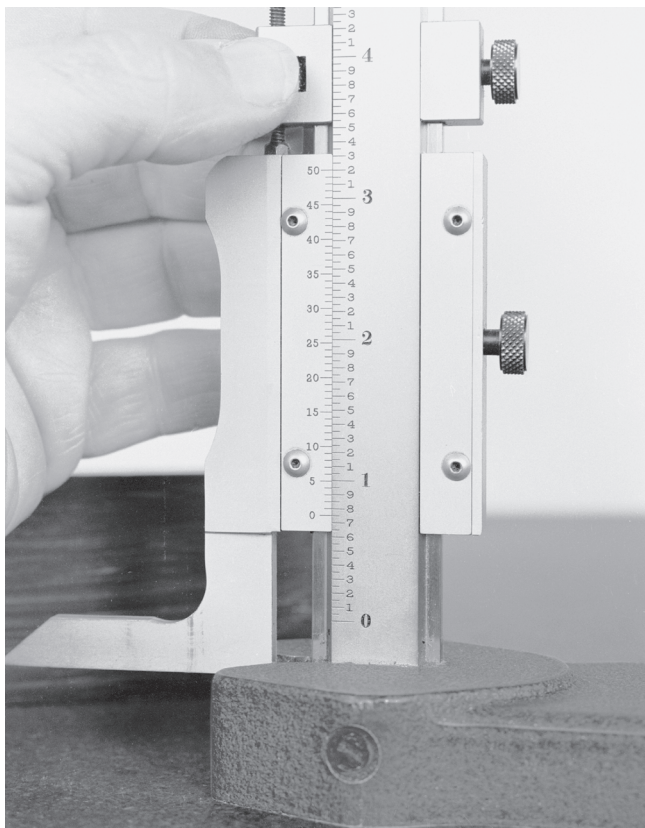
Figure E-72 Setting the height gage to a dimension of .750 in.
