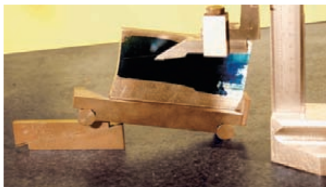
Figure E-69 Laying out angle lines using the sine bar.
