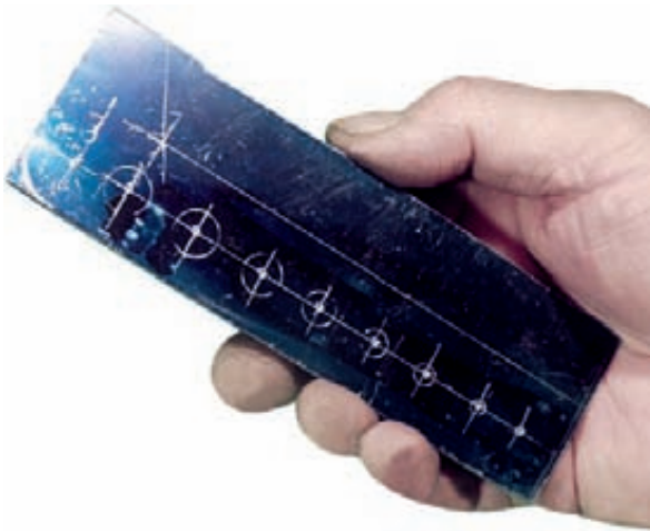
Figure E-48 Completed layout for the drill and hole gage.
