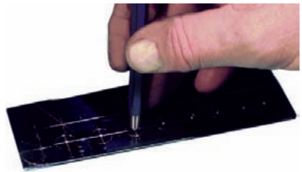
Figure E-47 Center punching the hole centers.
