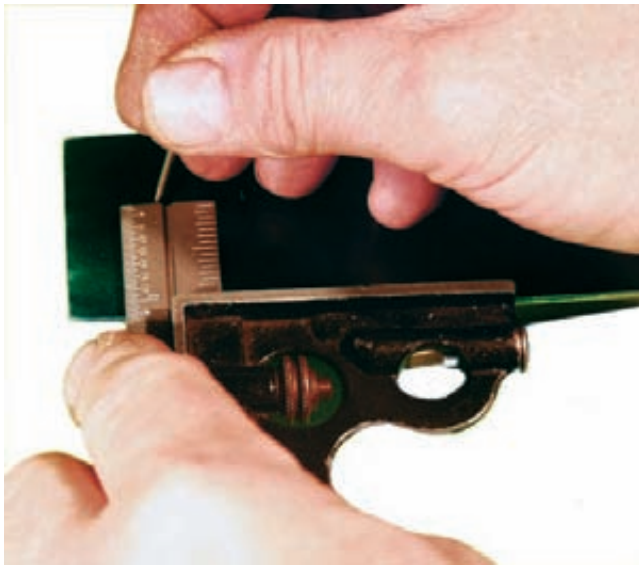
Figure E-34 Measuring and marking the width of the gage using the combination square and rule.
