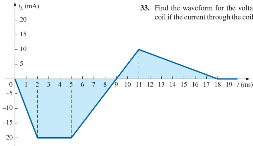
33. Find the waveform for the voltage induced across a 5 mH coil if the current through the coil is as shown in Fig. 11.104.
