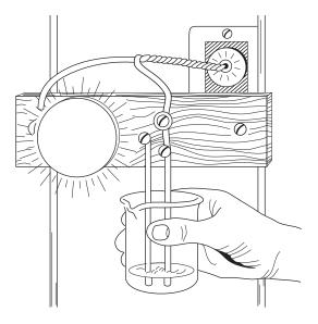
**Figure 18.1** *Conductivity-sensing apparatus*
