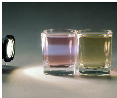
A beam of light is visible in a colloid solution (left) but not in a true solution. The size of the particles in the colloid are large enough to scatter the light beam making it visible.
