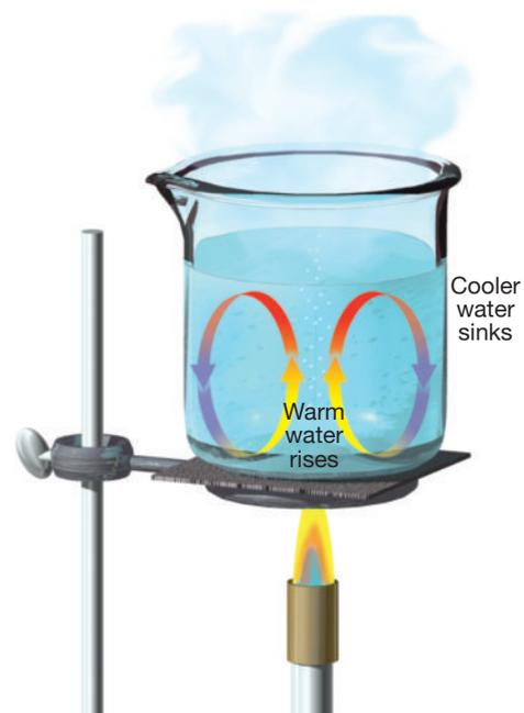
**FIGURE 12.14** A simple example of convection, which is heat transfer that involves the actual movement of a substance. Here the flame warms the water in the bottom of the beaker. This heated water expands, becomes less dense (more buoyant), and rises. Simultaneously, the cooler, denser water near the top sinks.
